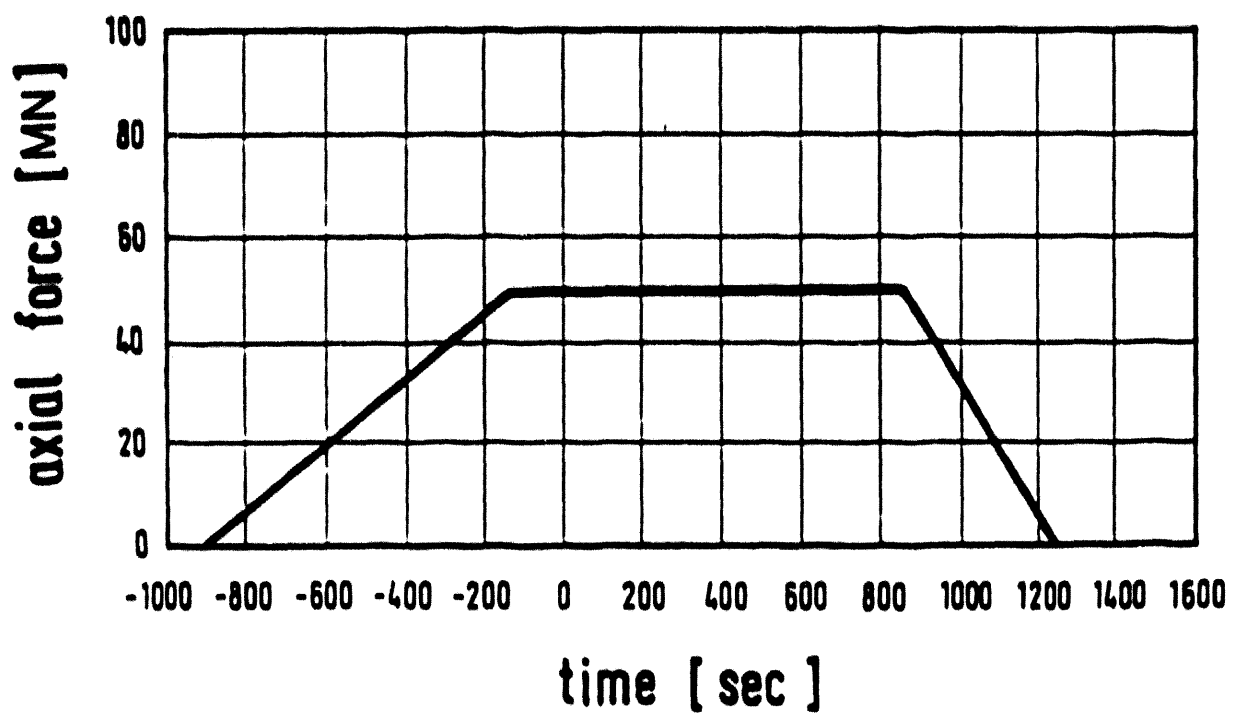
Figure 6b: Axial load vs time (NKS 4)
