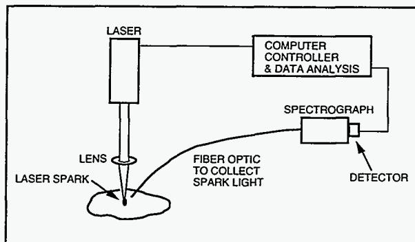
Figure 1.31a. Schematic representation of a basic laser-induced breakdown spectroscopy instrument.
