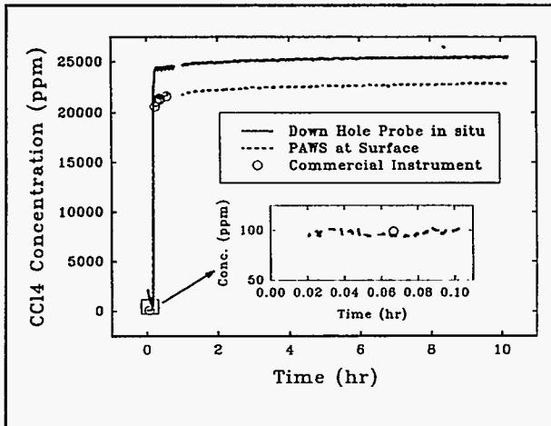
Figure 1.27c. Real-time monitoring of contamination at the Hanford Site using a down hole portable acoustic wave sensor system for in situ analysis.
