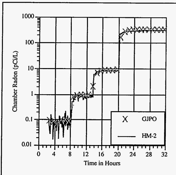
Figure 1.32c. An overlay of the particulate-corrected HM-2 and Grand Junction Project Office data.
