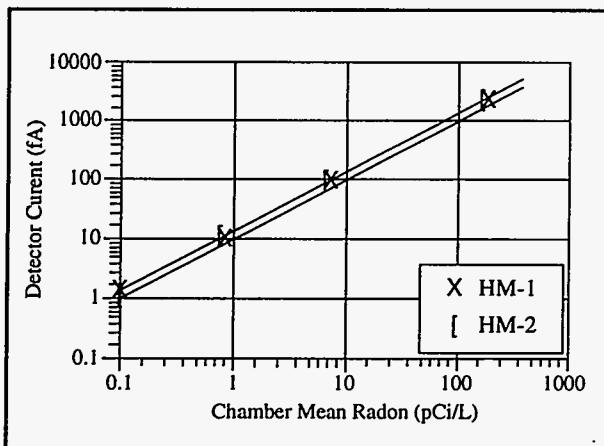
Figure 1.32b. Radon response of two long-range alpha detector, technology-based detectors, HM-1 and HM-2.
