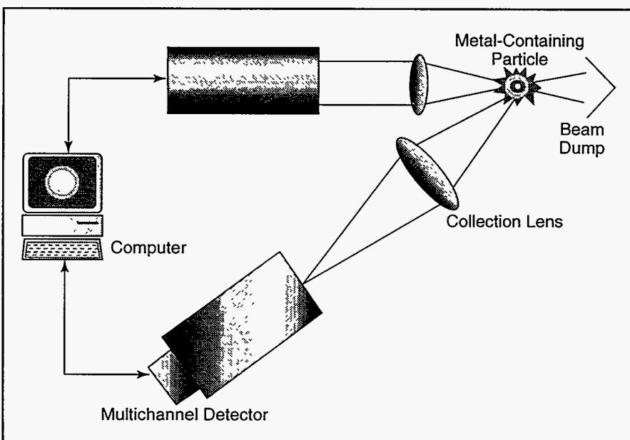
Figure 4.1. Schematic of the Laser Spark Technique measuring atomic species.
