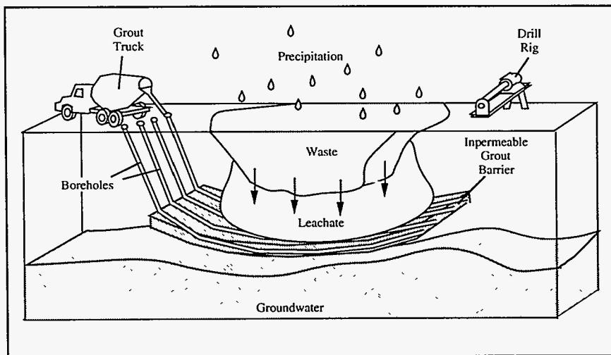
Figure 1.19. Subsurface Barrier Application.
