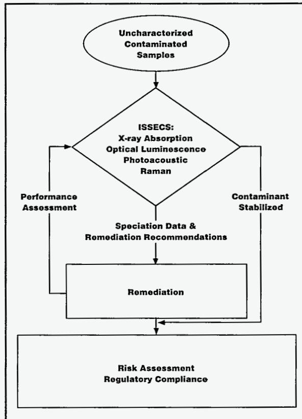
Figure 1.22. Integrated Spectroscopic System Process.
