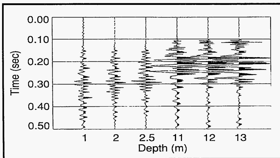
Figure 1.35b. Example of cross hole data collected with Bolt airgun at Hanford site.
