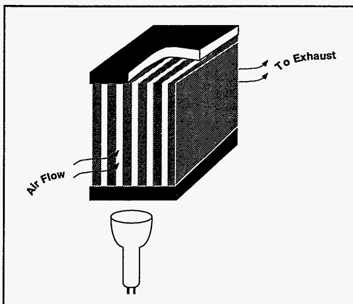
Figure 2.18a. The Large Volume Flow-Through Detection System Concept.
