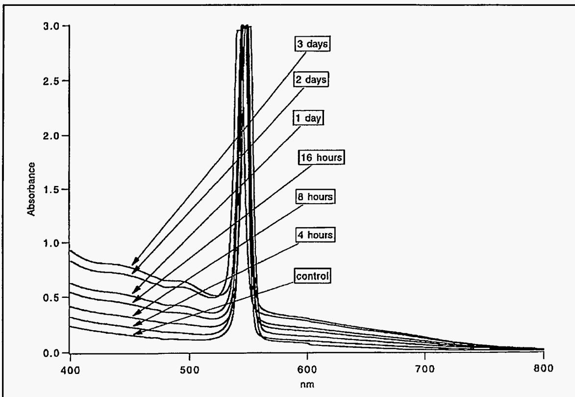
Figure 1.37. Absorption of holographic filters vs. exposure time at 435 Rad/min.
