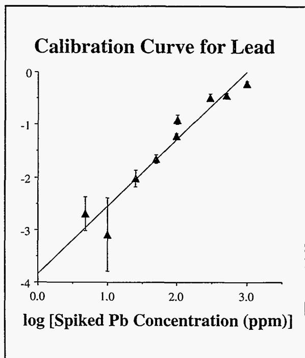
Figure 1.31b. Calibration curve for Los Alamos soil spiked with lead.
