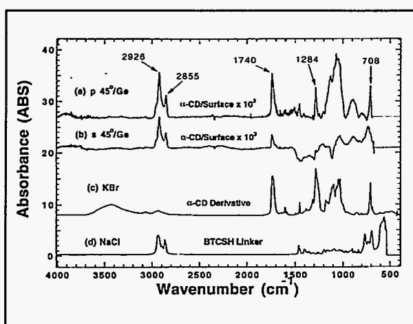
Figure 1.28a. Fourier-transform infrared-attenuated total reflection (FTIR-ATR) spectra of (a)  $\alpha$ -cyclodextrin monolayer covalently bound to the native oxide surface of  $\text{Si}\langle 100 \rangle$  with a  $\text{kGe}$  internal reflection element and  $p$ -polarized light incident at  $45^\circ$ , 1024 scans,  $2\text{cm}^{-1}$  resolution; (b)  $s$ -polarized; (c) bulk  $\alpha$ -cyclodextrin derivative (KBr disk), (d) neat linker on  $\text{NaCl}$  crystal.
