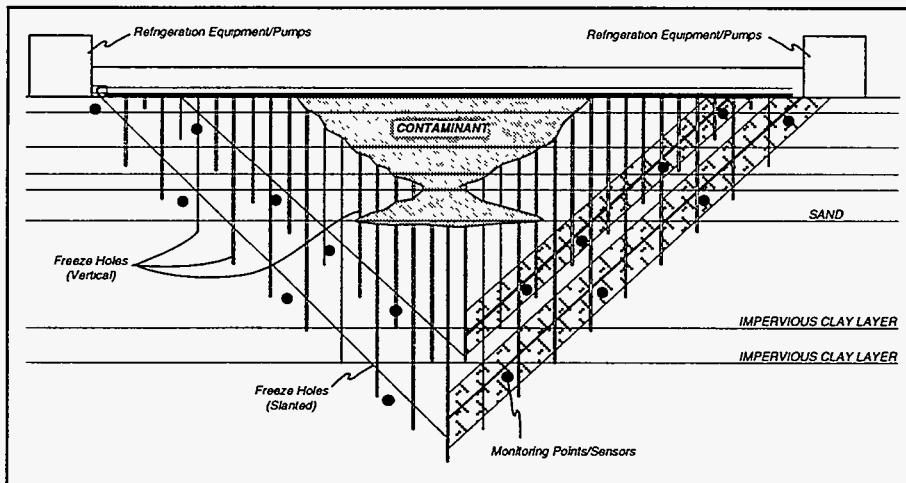
Figure 1.40. Cryogenic Barrier at an Arid site; cross-sectional view.
