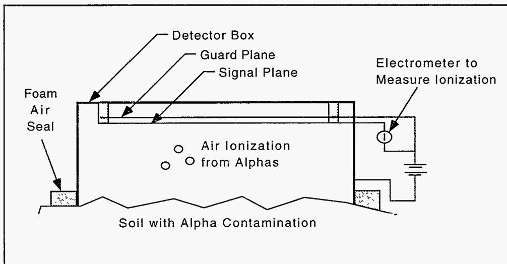
Figure 1.21. Schematic of Long-Range Alpha Detector Soil Surface Monitoring.
