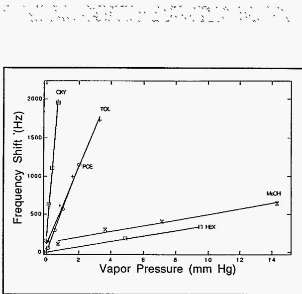
Figure 1.28b. Linear concentration dependent SAW response of various analytes to an a-cyclodextrin monolayer coated 200 Hz resonator: perchloroethylene, toluene, o-xylene, methanol, and hexane.
