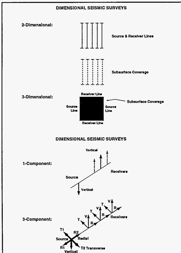
Figure 1.34a. Seismic survey definitions.
