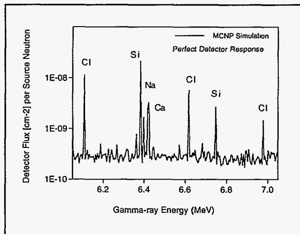
Figure 1.30a. Small portion of a simulated gamma-ray energy spectrum.
