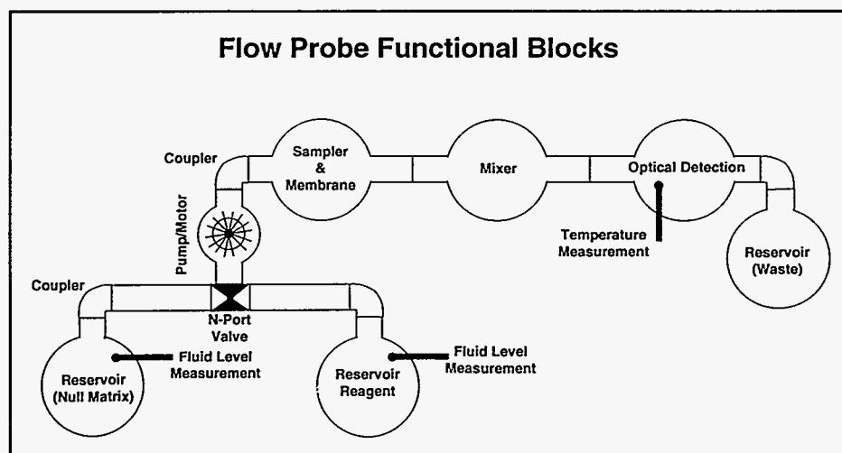
Figure 1.26. Schematic Representation of Functional Blocks for the Flow Probe in a Possible Pevice Arrangement.
