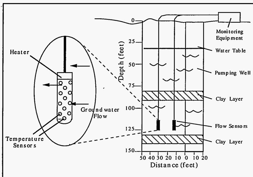
Figure 1.1. In Situ Permeable Flow Sensor.
