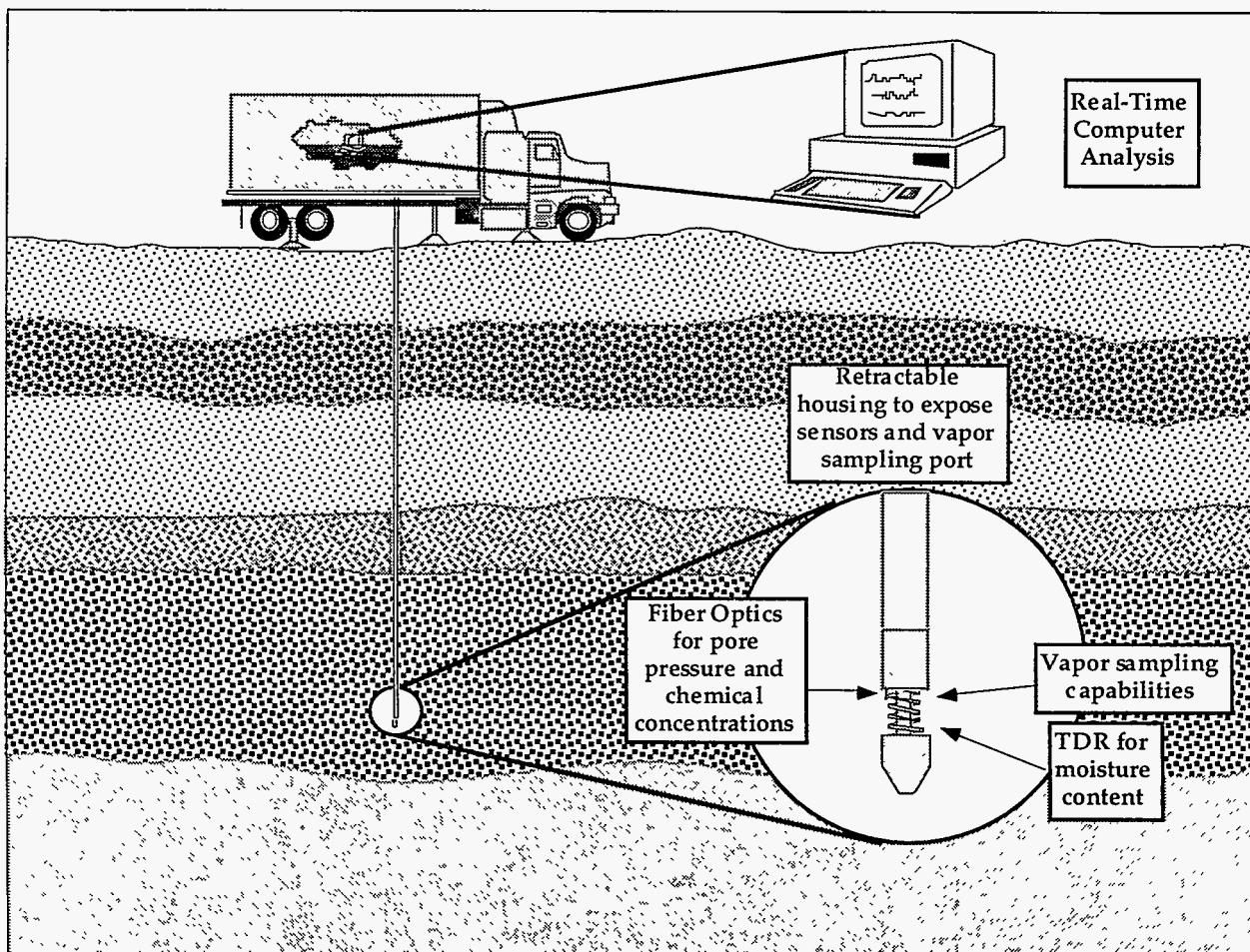
Figure 1.25. Cone Penetrometer Tip for Hydrologic Investigations.
