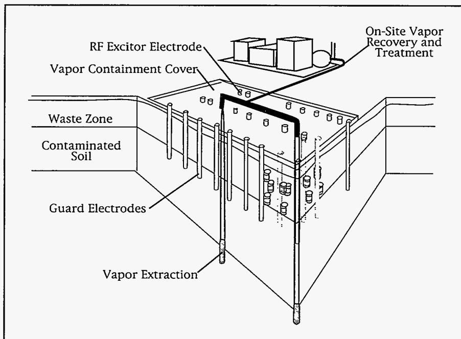
Figure 1.16. Thermal Enhanced Vapor Extraction System.
