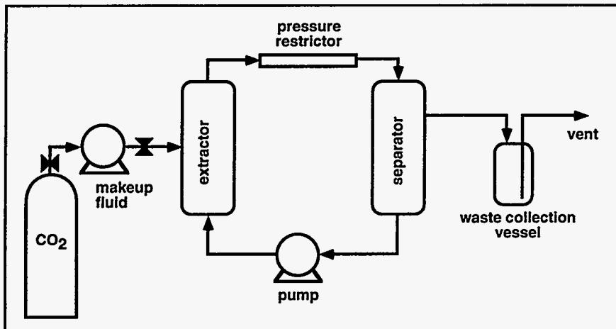
Figure 3.4. Ideal Supercritical Carbon Dioxide Cleaning System.
