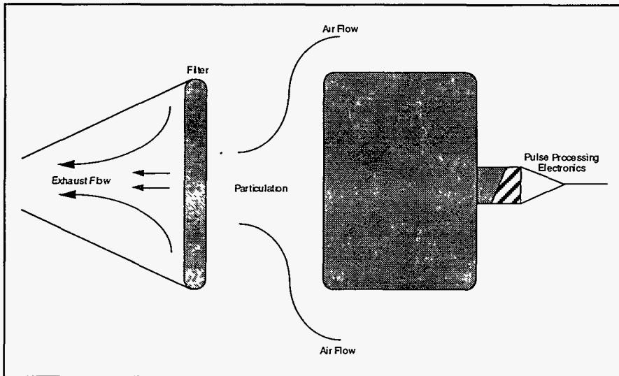
Figure 2.18b. Typical Stack Gas Alpha Detection System.
