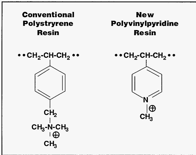
Figure 2.11. New resins have greatly improved chemical and radiation stability.
