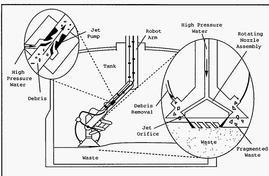
Figure 2.6. Water Jet Cutting.
