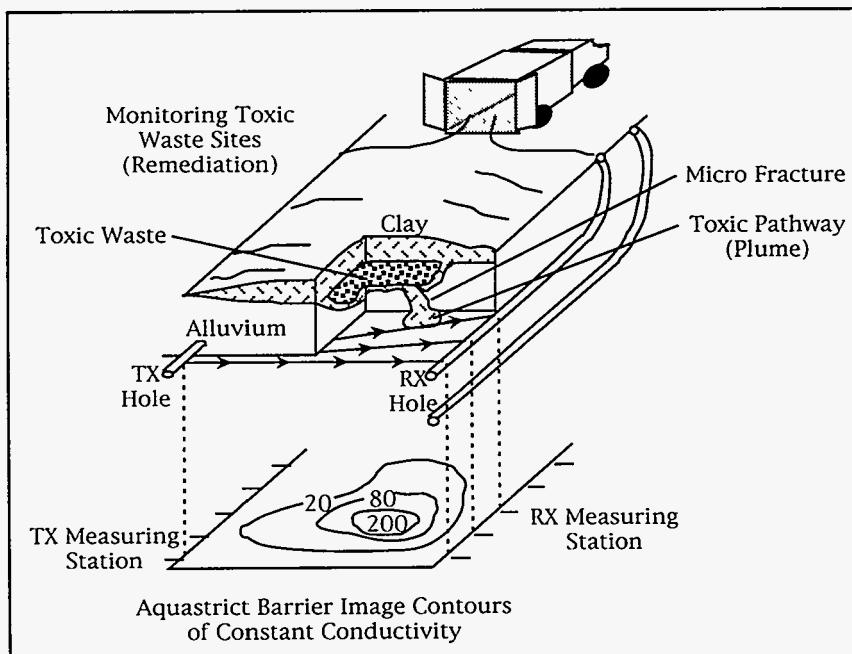
Figure 1.13. Cross Borehole Electromagnetic Imaging.
