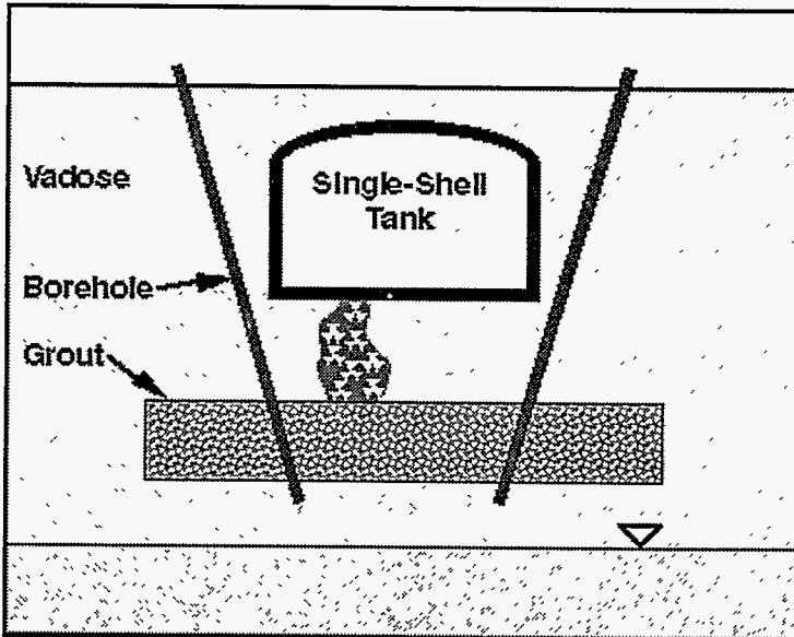
Figure 1.38. Evaluation of new grout barriers.
