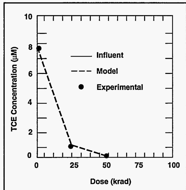
Figure 2.13. Simulated and Experimental Removal of 1 ppm TCE in Potable Water.
