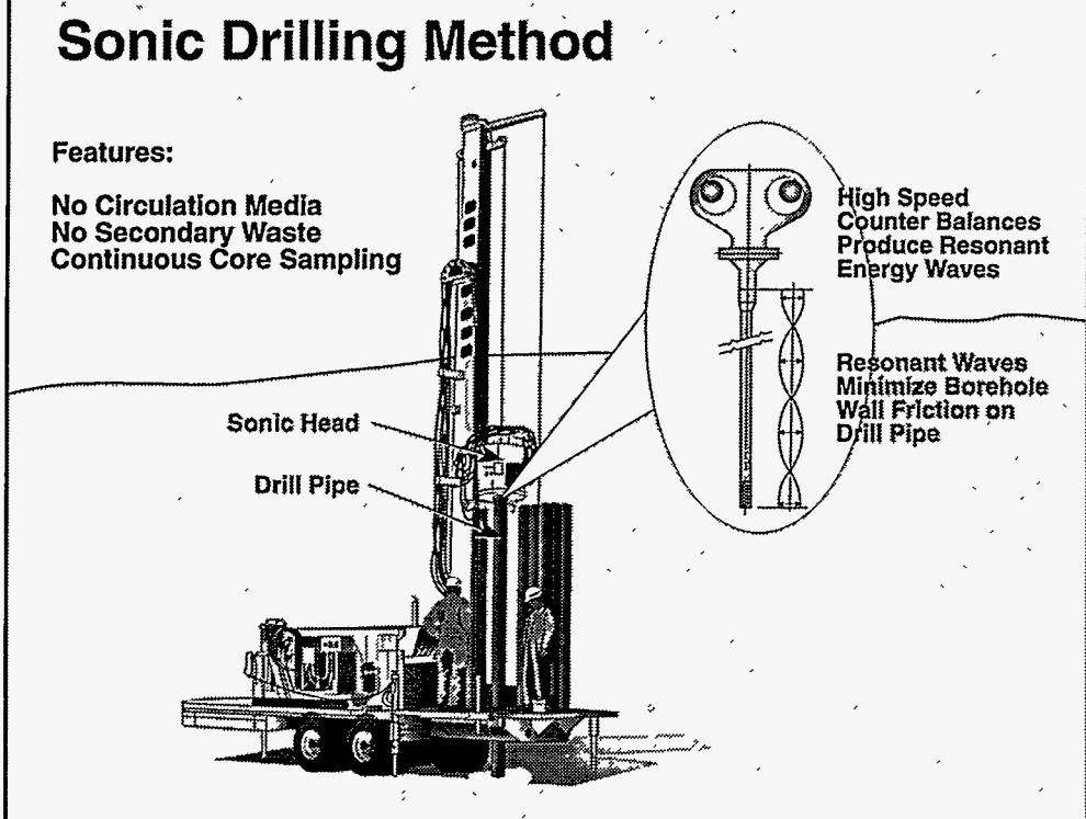
Figure 1.3a. ResonantSonic<sup>SM</sup> Drilling.
