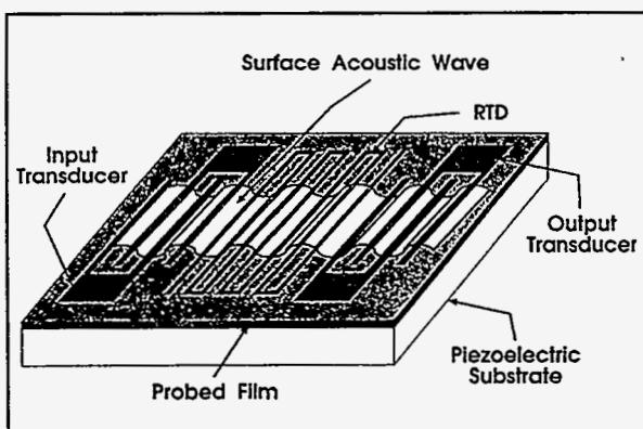
Figure 1.27a. Schematic of a Surface Acoustic Wave Sensor.
