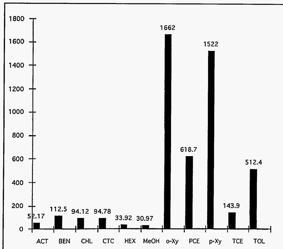
Figure 1.28c. Comparisons of the responses of the self-assembled a-cyclodextrin monolayer coated 200 MHz SAW resonator microsensors to a variety of analytes at unit organic vapor concentration (Hz/mmHg): Acetone, benzene, chloroform, carbon tetrachloride, hexanes, methanol, o-xylene (o-Xy, perchloroethylene, p-xylene, trichloroethane, and toluene. Note the a-cyclodextrin coated monolayer thin film is very selective to xylenes, PCE, and toluene.
