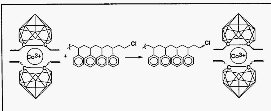
Figure 2.7. Incorporation of Dicarbollides onto Polymers.
