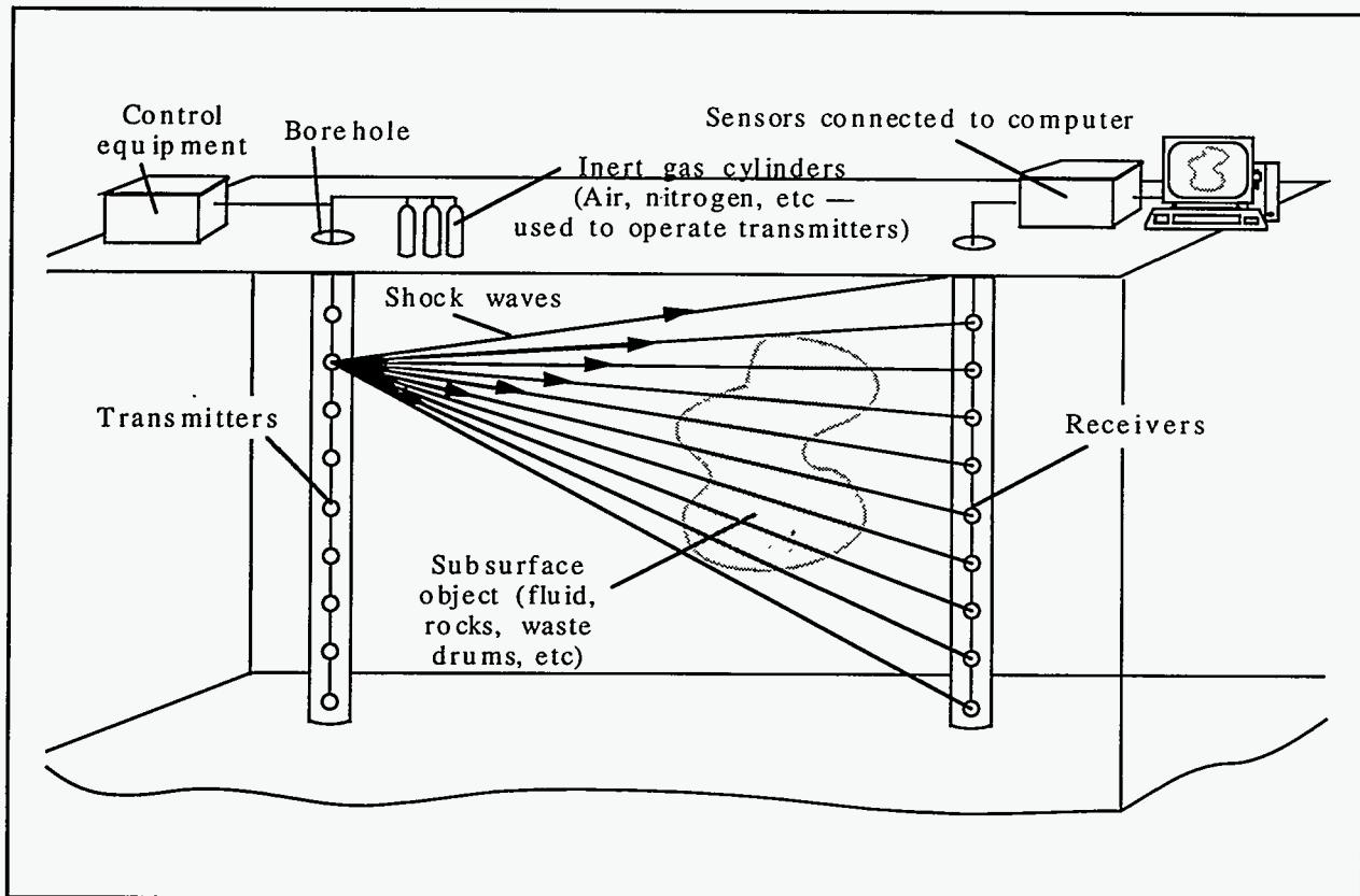
Figure 1.2. Crosswell Seismic Imaging.
