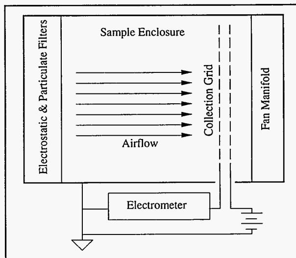
Figure 1.32a. Schematic of a long-range alpha detector, technology-based air-quality monitor.
