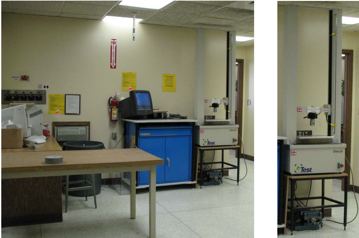
Figure 4. The MTS Q-Test/25 load cell used to measure shear strength of the ESW glass-to-metal bonds.
