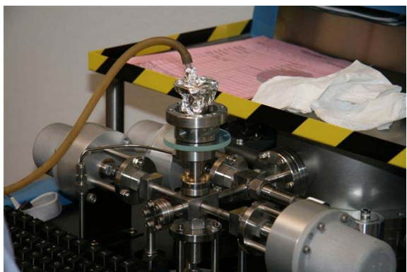
Figure 11b. The glass is jacketed with pure helium at 1 atm, and the helium leak rate is measured after it stabilizes (several hours).
