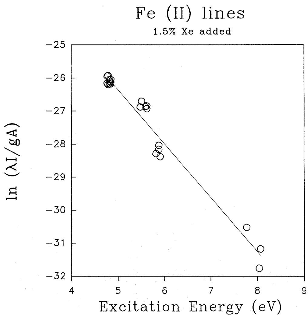
Figure 10. Boltzmann plot for the emission of Fe (II) lines with 1.5% xenon added to the central channel of the ICP.
