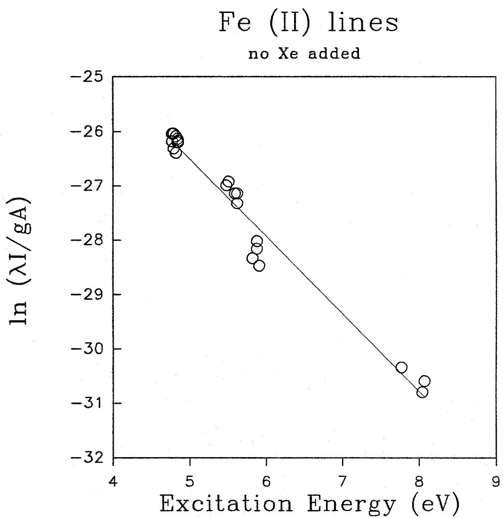
Figure 7. Boltzmann plot for the emission of Fe (II) lines with no xenon added to the central channel of the ICP.
