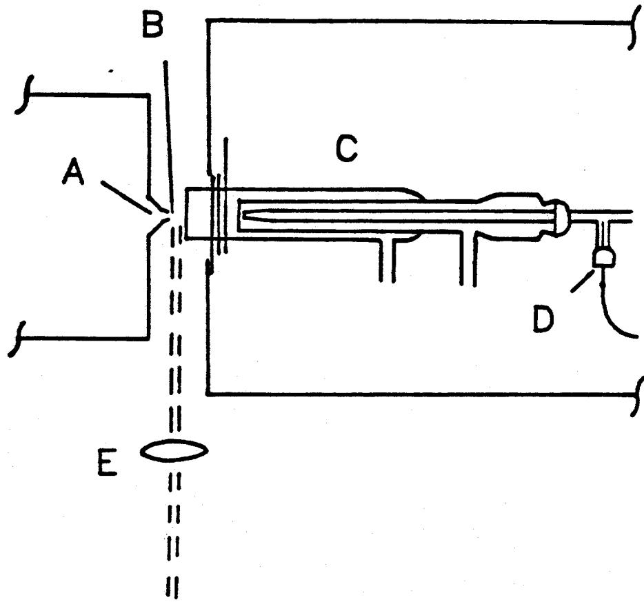
Figure 1. Instrumental setup for observation of Fe (I) and Fe (II) emission from the ICP. A = sampler on ICP-MS interface, B = region viewed by monochromator, C = ICP torch, D = quartz tee for the introduction of xenon, E = lens. Reproduced from reference (144) with permission.
