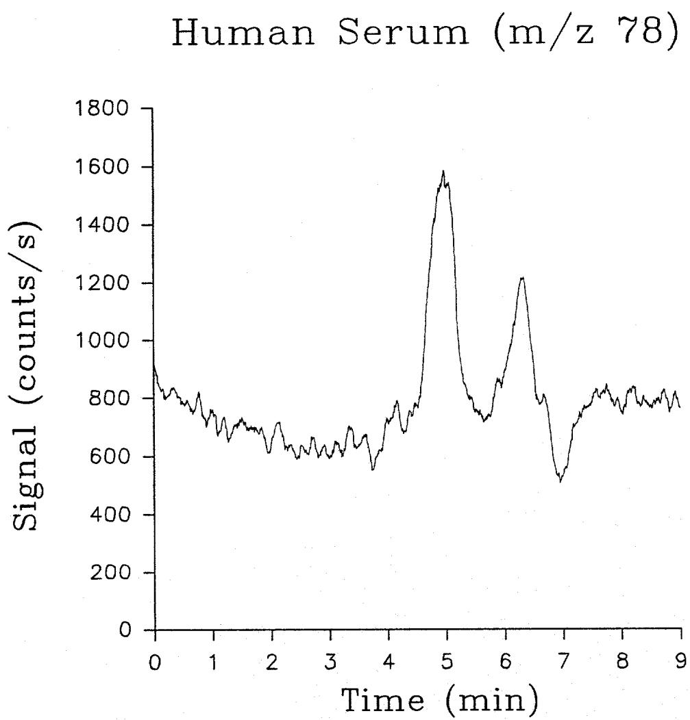
Figure 2. Selected ion chromatogram of metalloproteins in human serum monitoring m/z 78.
