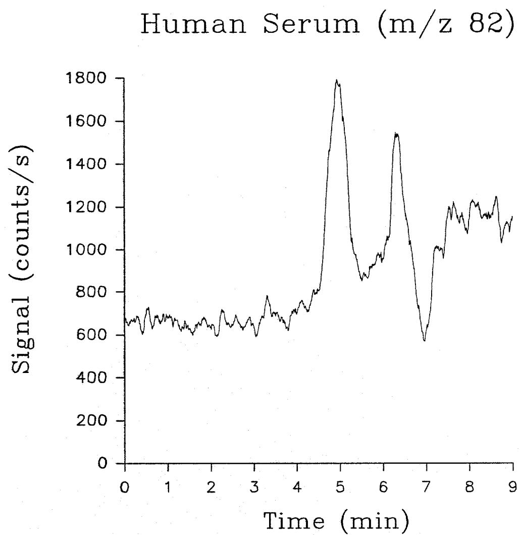
Figure 3. Selected ion chromatogram of metalloproteins in human serum monitoring m/z 82.
