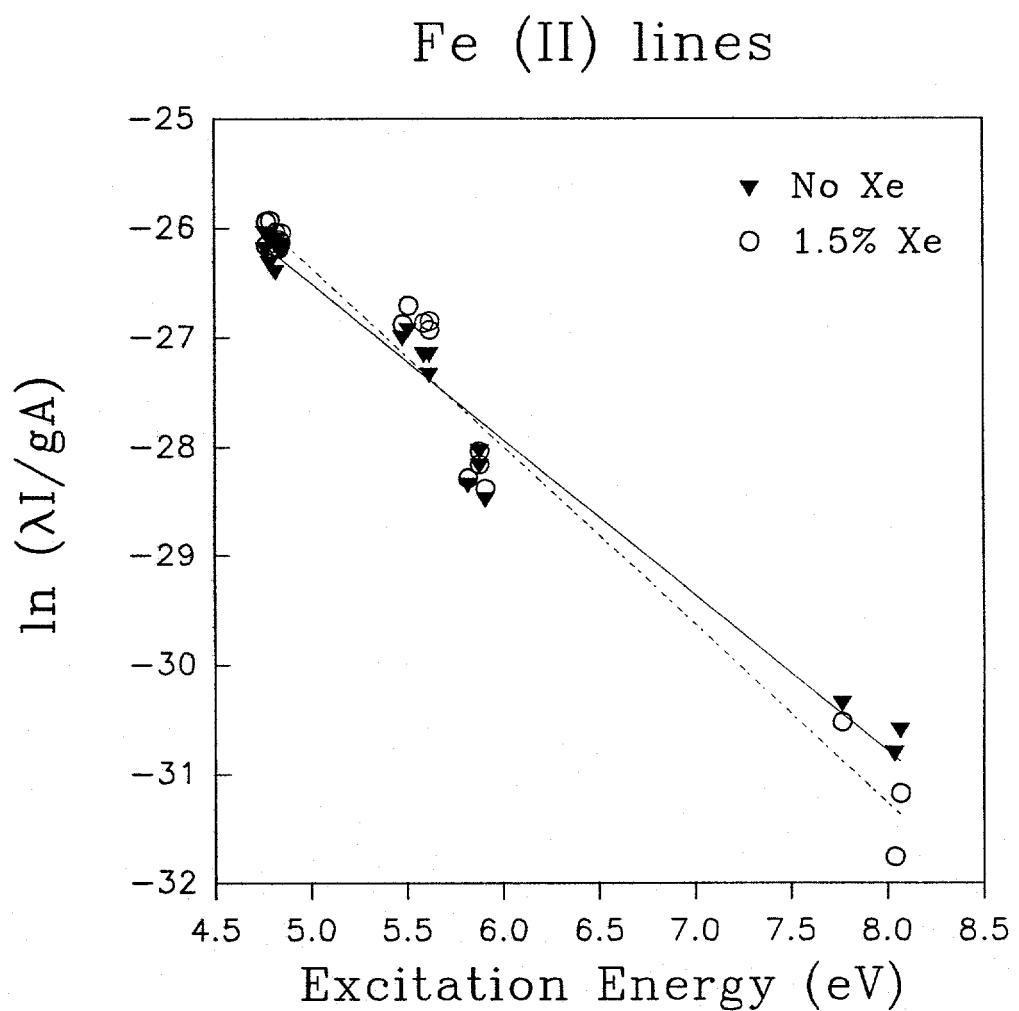
Figure 11. Boltzmann plots for the emission of Fe (II) lines with 0 and 1.5% xenon added to the central channel of the ICP.
