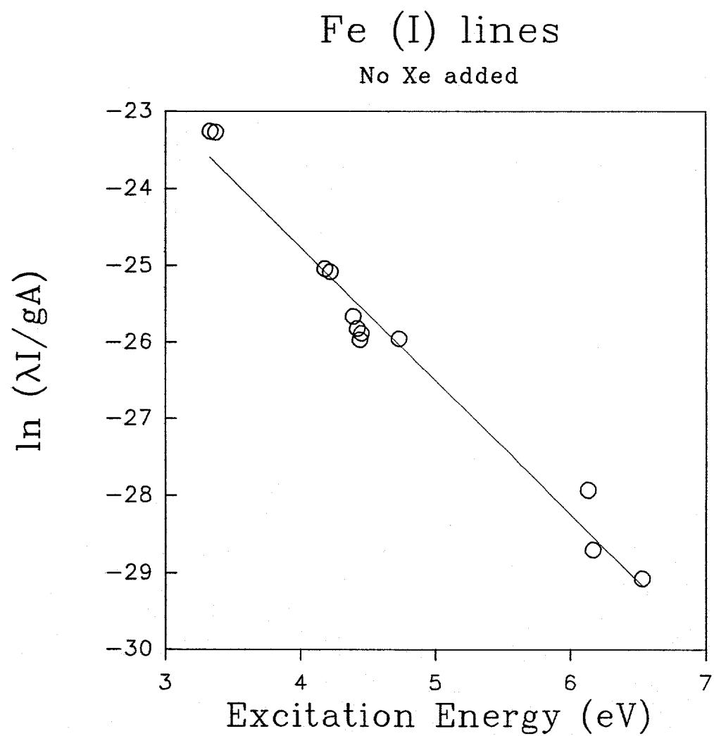
Figure 2. Boltzmann plot for emission from Fe (I) lines with no xenon added to the central channel of the ICP.
