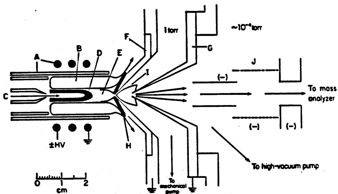
Figure 1. ICP and ion sampling interface. A = torch and load coil (HV = high voltage), B = induction region of ICP, C = a solution aerosol being injected into axial channel, D = initial radiation zone, E = normal analytical zone, F = nickel cone with sampling orifice in tip, G = skimmer cone, H = boundary layer of ICP gas deflected outside sampling orifice, I = expanding jet of C gas sampled from ICP, and J = ion lens elements. Reproduced from reference (76) with permission.
