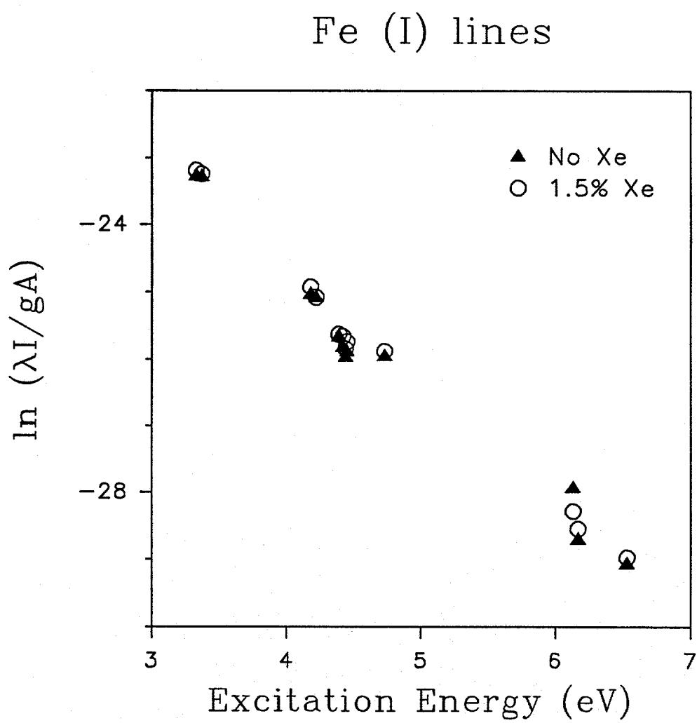
Figure 6. Boltzmann plots for the emission of Fe (I) lines with 0 and 1.5% xenon added to the central channel of the ICP.
