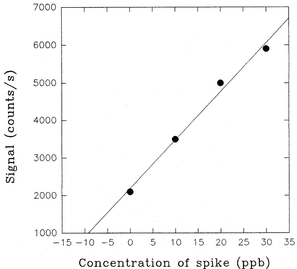
Figure 5. Standard additions plot for selenium in human serum ( $R = 0.9948$ ).
