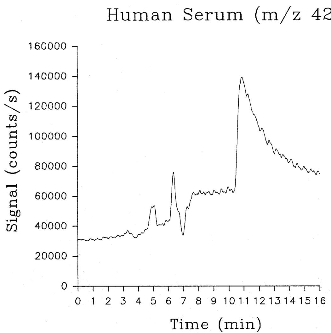
Figure 4. Selected ion chromatogram of metalloproteins in human serum monitoring m/z 42.
