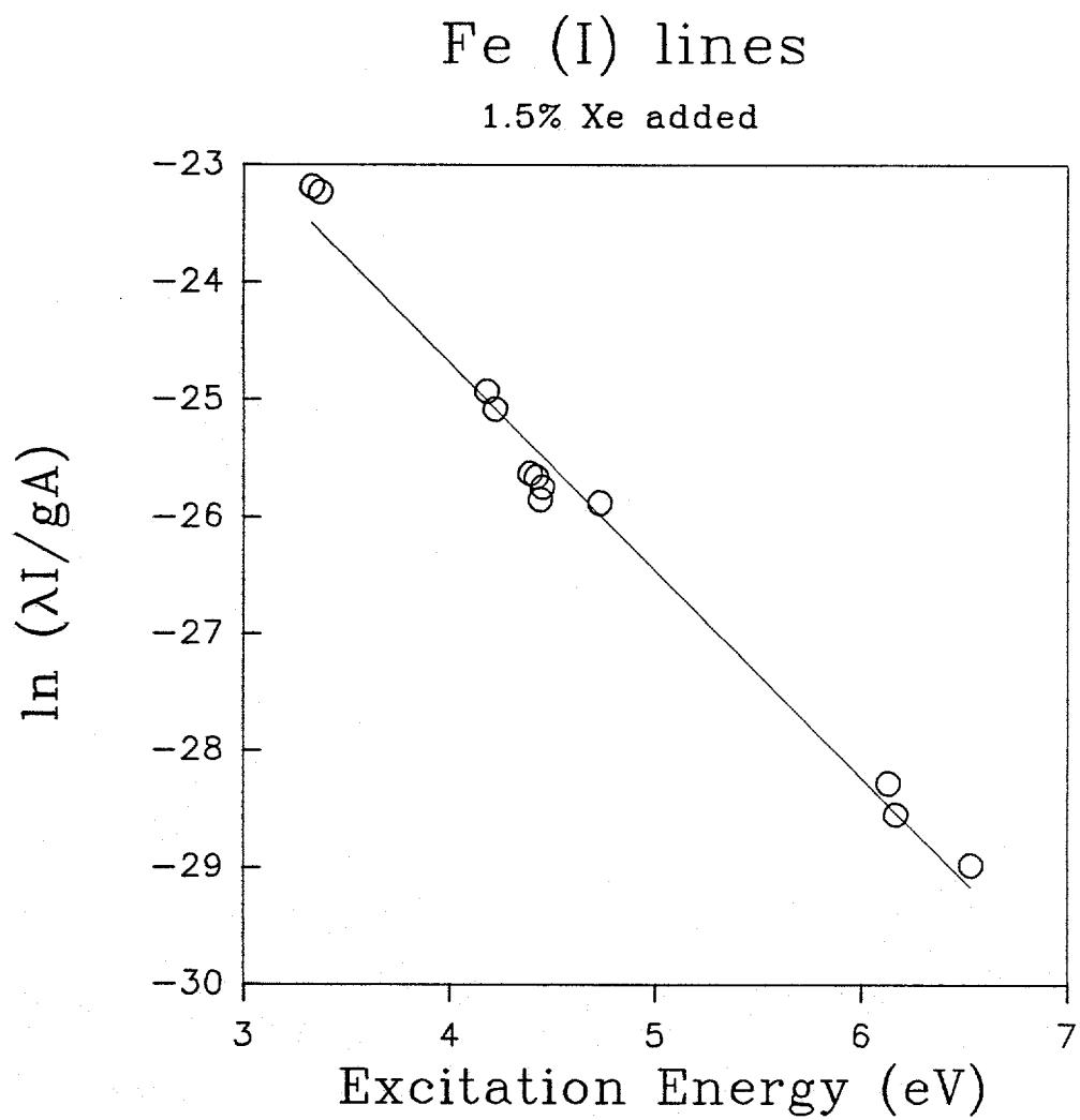
Figure 5. Boltzmann plot of emission from Fe (I) lines with 1.5% xenon added to the central channel of the ICP.
