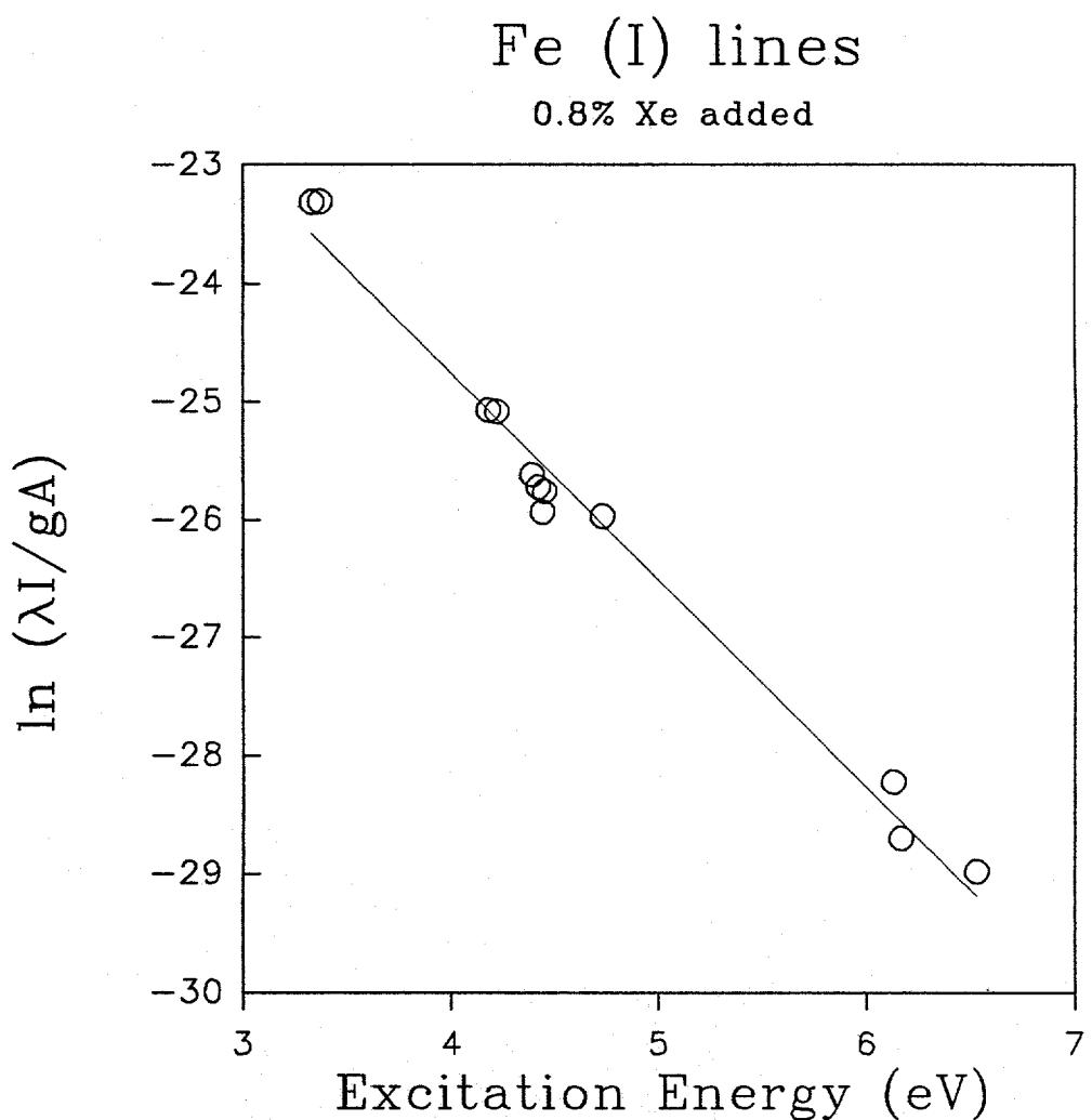
Figure 4. Boltzmann plot for the emission of Fe (I) lines with 0.8% xenon added to the central channel of the ICP.
