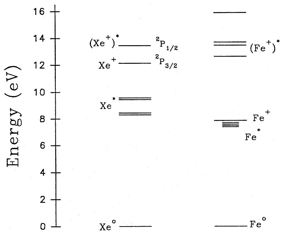
Figure 13. Energy level diagram showing some of the states of xenon and iron below 16 eV.
