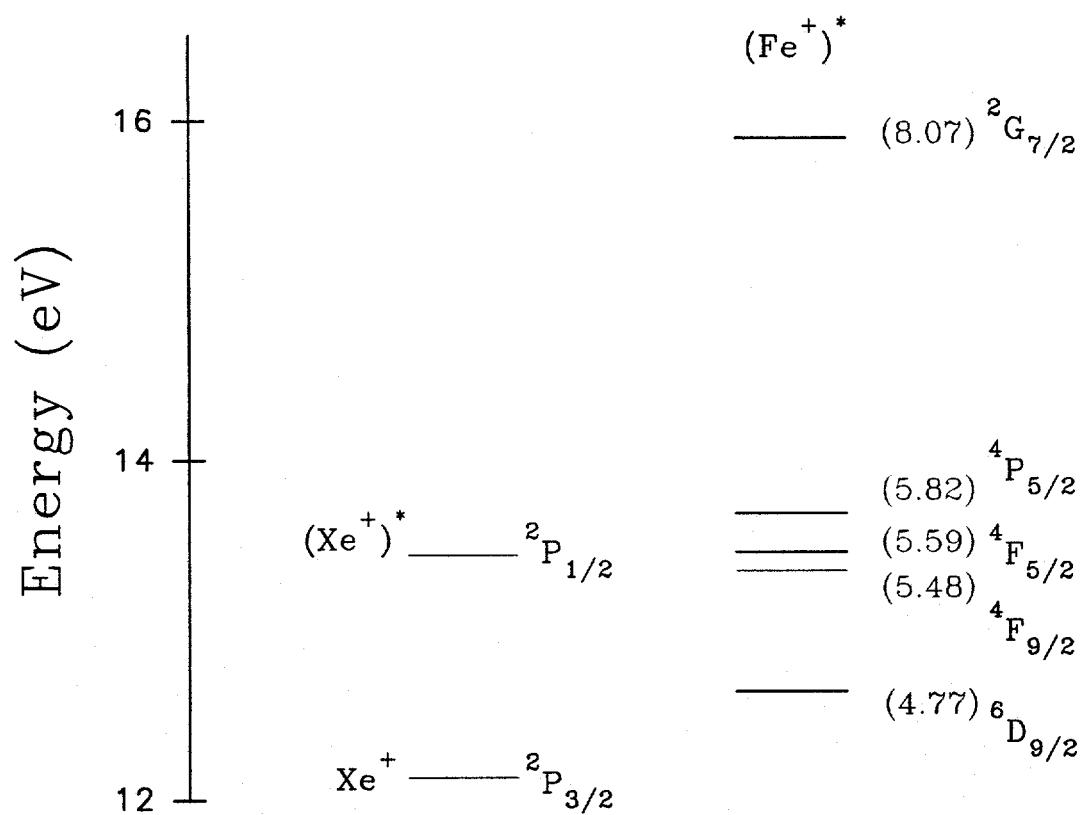
Figure 14. Energy level diagram showing states of xenon and iron between 12 and 16 eV.
