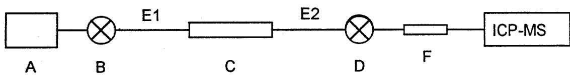
**Figure 1.** Schematic diagram of instrumental setup for the speciation of selenium in human serum with ICP-MS detection. A = HPLC pump, B = injection valve with 3  $\mu$ l sample loop, C = analytical column, D = switching valve, E1, E2 = polysil connecting tubing, F = direct injection nebulizer (DIN).
