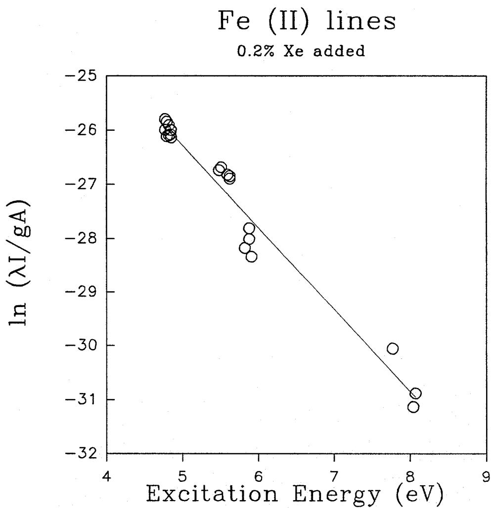
Figure 8. Boltzmann plot for the emission of Fe (II) lines with 0.2% xenon added to the central channel of the ICP.
