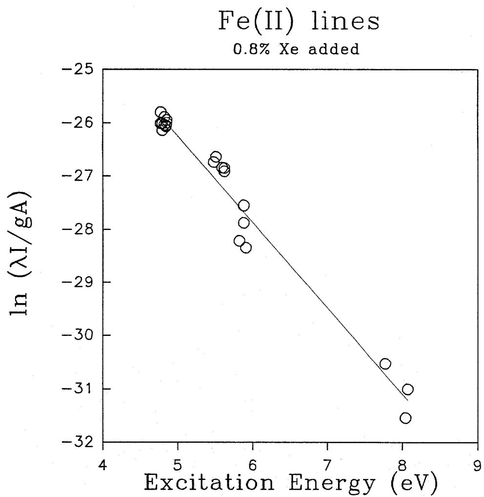
Figure 9. Boltzmann plot for the emission of Fe (II) lines with 0.8% xenon added to the central channel of the ICP.
