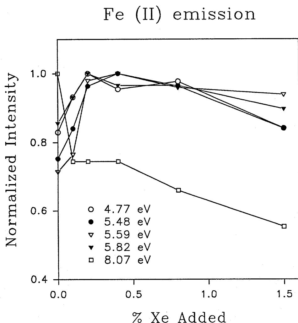
Figure 12. Plot of normalized emission intensity versus percent xenon added to the central channel of the ICP for several Fe (II) lines of various excitation energies.
