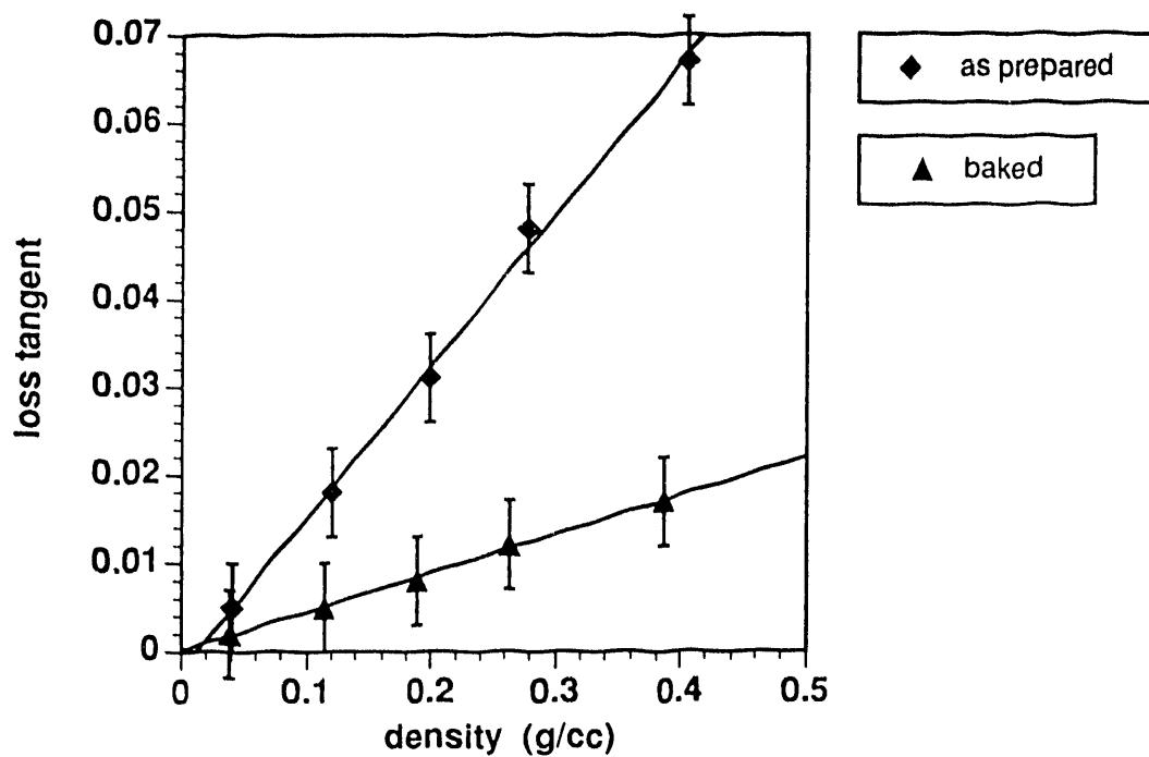
Figure 2. Plot of loss tangent for 'as prepared' and 'baked' silica aerogel versus density.
