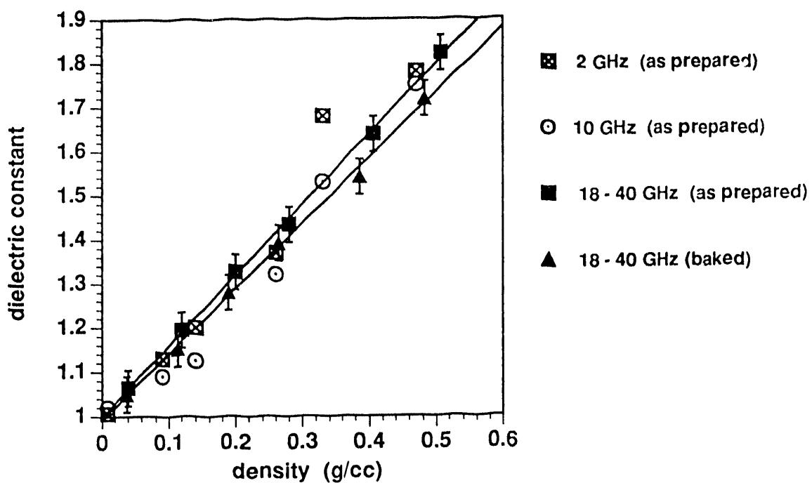
Figure 1. Plot of dielectric constant for 'as prepared' and 'baked' silica aerogel versus density.
