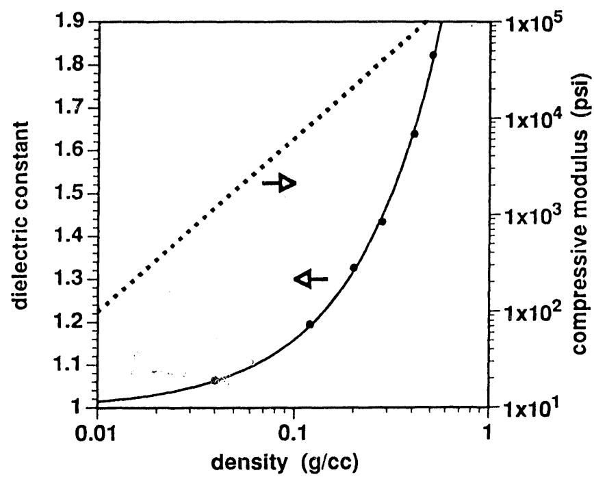
Figure 5. Dielectric constant and modulus vs density for silica aerogel.
