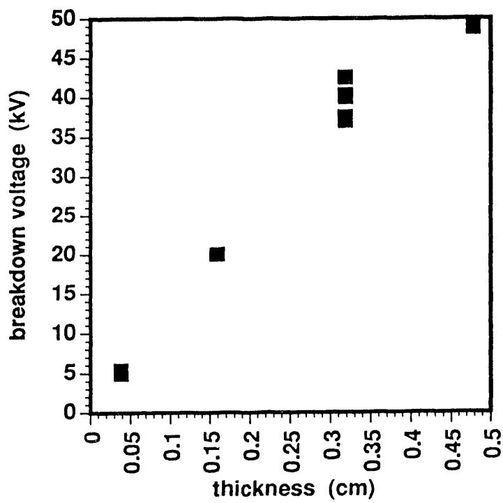
Figure 6. Breakdown voltage for various thicknesses of silica aerogel. The average dielectric strength for the silica aerogels is 128 kV/cm.
