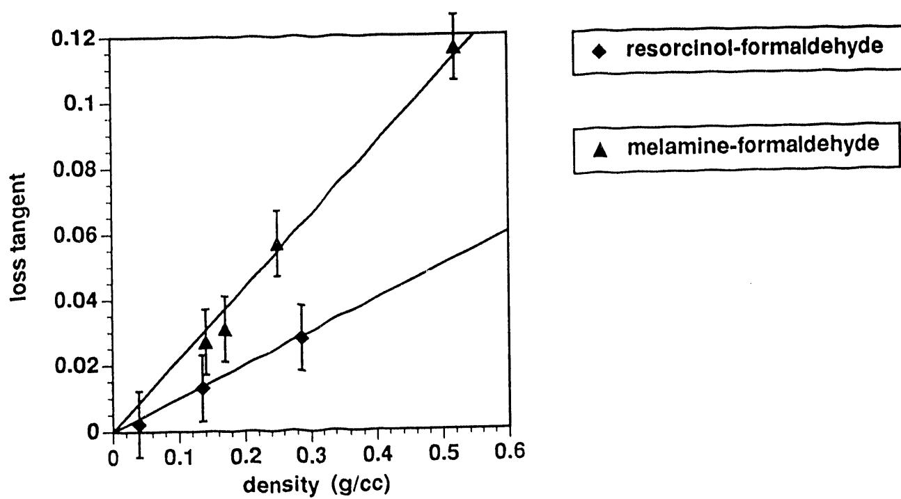
Figure 4. Plot of the loss tangent for organic aerogels versus density.
