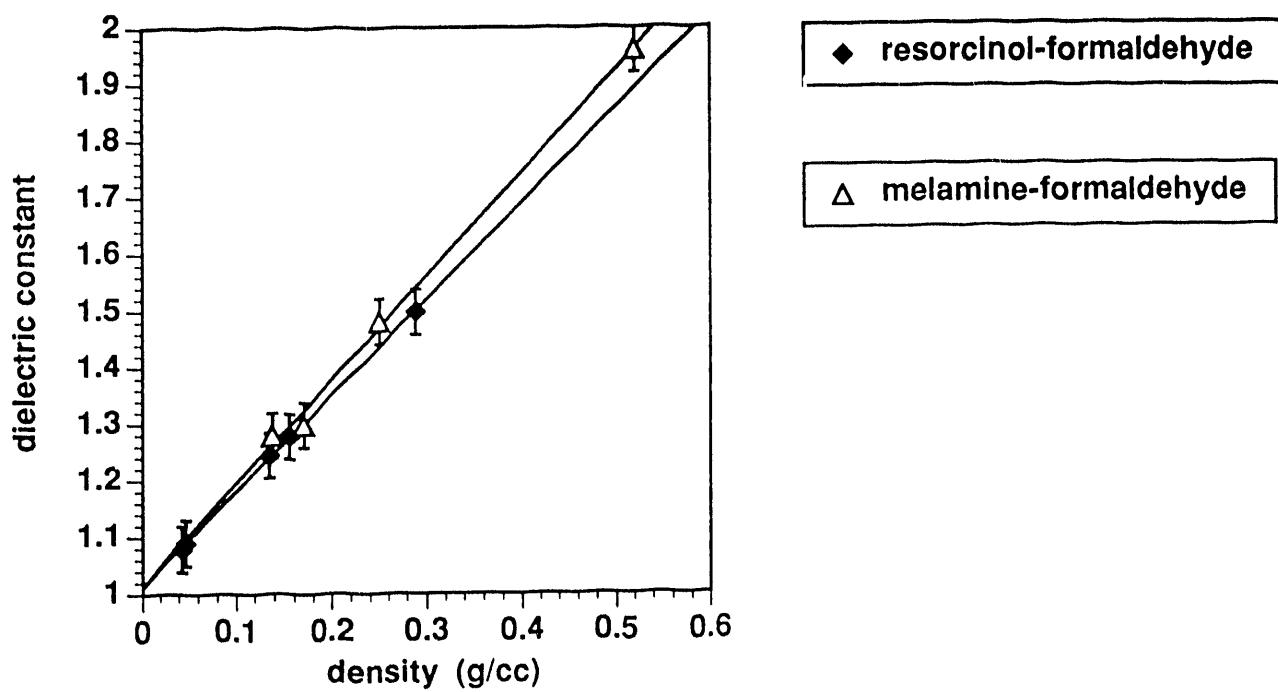
Figure 3. Plot of the dielectric constant for organic aerogels versus density.
