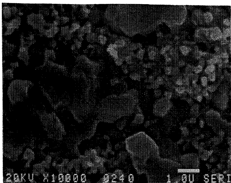
Fig. 5a. SEM of a selenized film obtained from a glass/Mo/In/Cu precursor. Large grain areas were found to be Cu rich.
