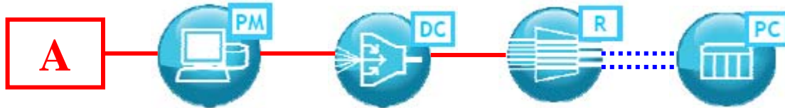
Figure 35. Testbed setup for Experiment R.5 (1000BASE-TX SFP, 1Gbps).
