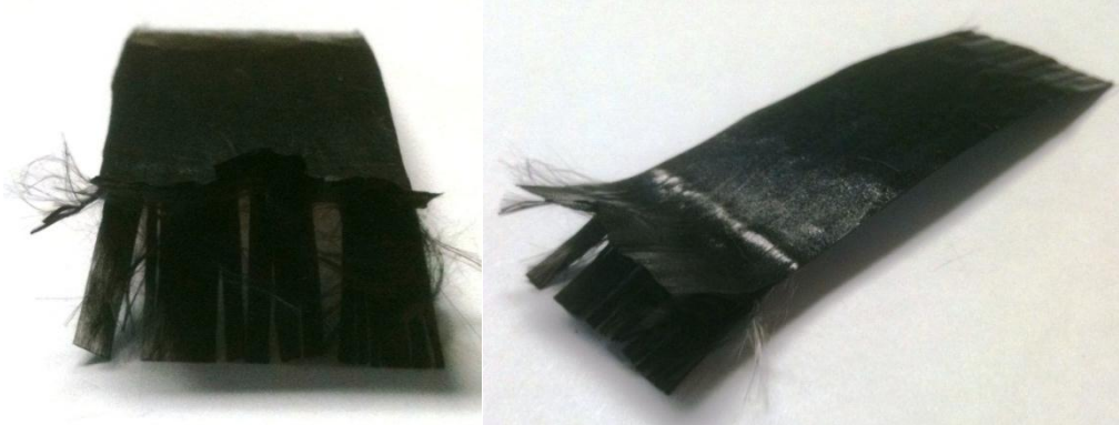
Figure 2. Partially impregnated composite prepreg tape sample with resin rich top and bottom surfaces (e.g. “shiny” surfaces of the tape within the figure) versus the fibrous dry center.
