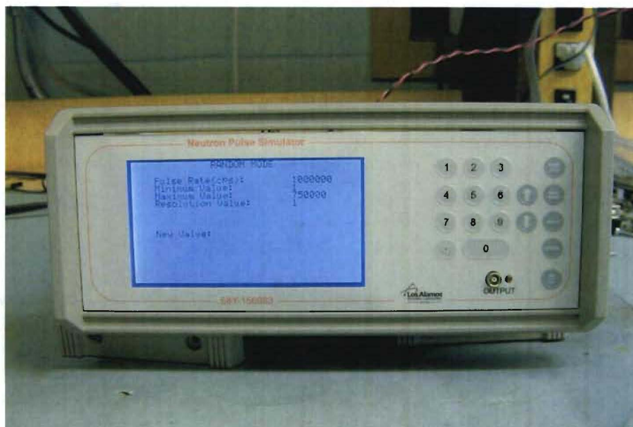
Figure 4: Picture of the neutron pulse simulator.
