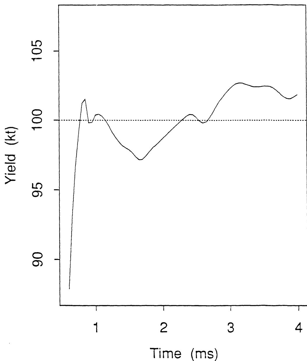
**Figure 1.** A typical yield-versus-time curve from a single CORTEX cable. The average yield was set arbitrarily at 100 kt.
