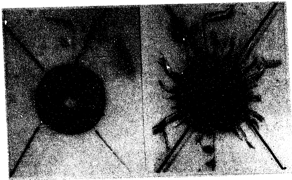
Figure 13. Photographs of the impact (left) and exit (right) craters in the PMMA target plate for Test 19. Plate thickness = 5.39 mm and impact velocity = 4.61 km/s.
