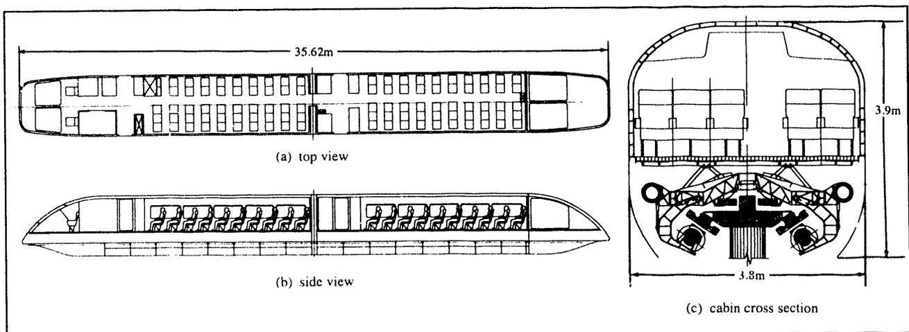
Fig. 1. Illustration of Grumman Maglev concept.
