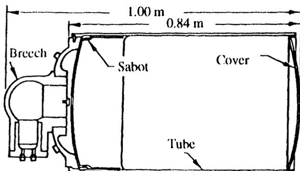
Fig. 8. Parachute deployment mortar (Ref. 8).
