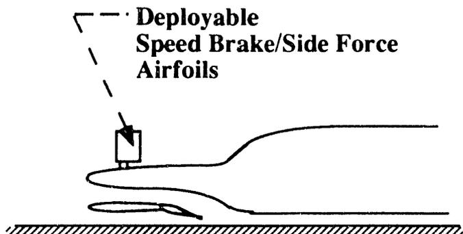
Figure 10 Deployable speed brakes are used to generate guidance forces in switches
