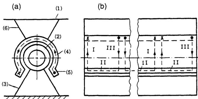
Fig. 3: Current path in motor: (a) front view; (b) side view. (1) vehicle, (2) primary drive coils, (3) primary support, (4) motor secondary: passive conducting cut cylinder, (5) edge, and (6) support for the secondary part.
