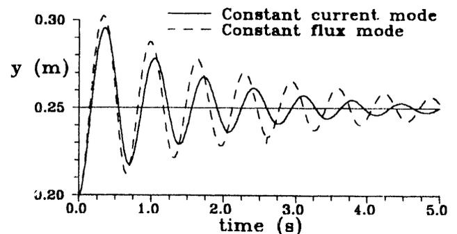
Fig. 9 - Step response with aluminium damping coils  $d = 0.10$  m.
