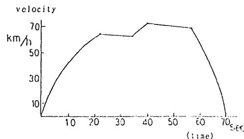
Fig. 6 The run curve for measuring energy consumption
