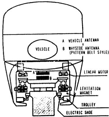
Fig.10 Layout of the girder structure and the signal systems in the Yokohama Exposition
