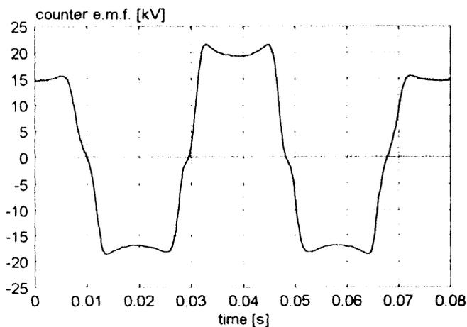
Fig.5 - Instantaneous c.e.m.f. at 500 km/h.
