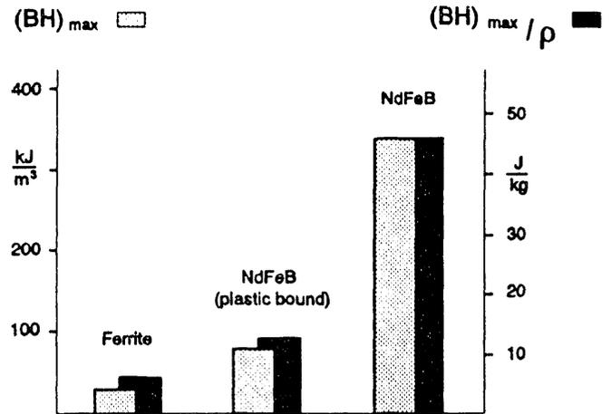
Fig. 4: Energy density of permanent magnetic materials
