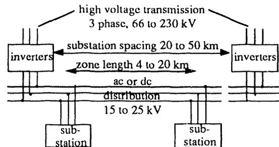
Fig. 6. Typical power distribution.
