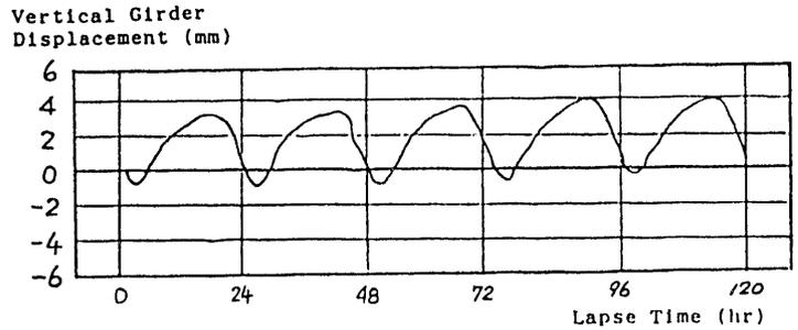
Fig.10 Daily change of Girder vertical displacement
