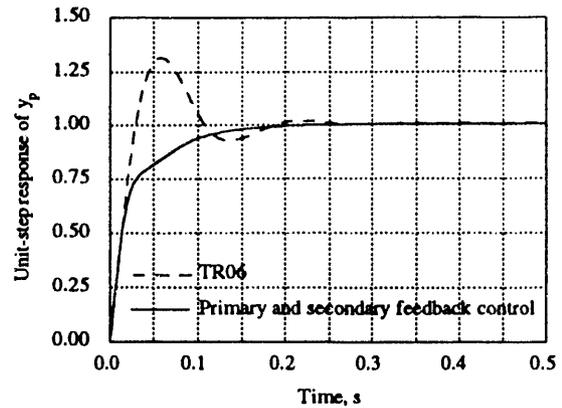
Fig. 10. Comparison of transient response  $y_p$  of primary suspension with unit-step input of guideway perturbation for TR06 and a new system using active and semiactive feedback controls in primary and secondary suspensions.
