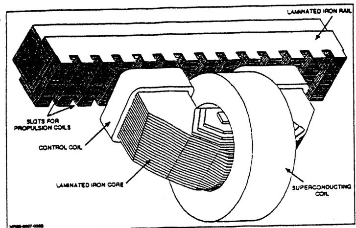
Fig. 1. EMS Levitation and Propulsion Systems
