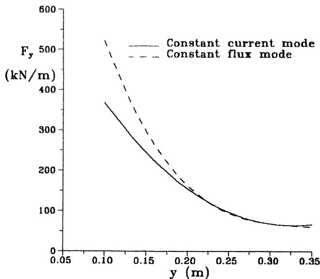
Fig. 6 - Static force-height characteristic.
