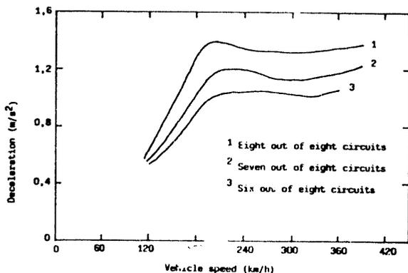
Fig.3 Braking characteristics of TR 07 eddy current brake (result of TÜV acceptance tests)
