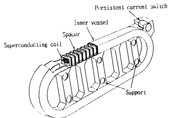
Fig.3 Illustration of the superconducting coil
