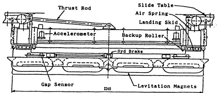
Fig.3 Module structure
