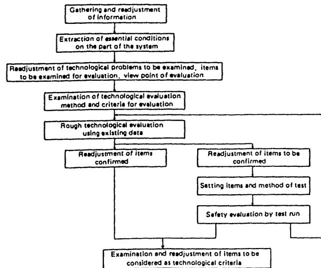
Fig. 1 Procedure of safety evaluation
