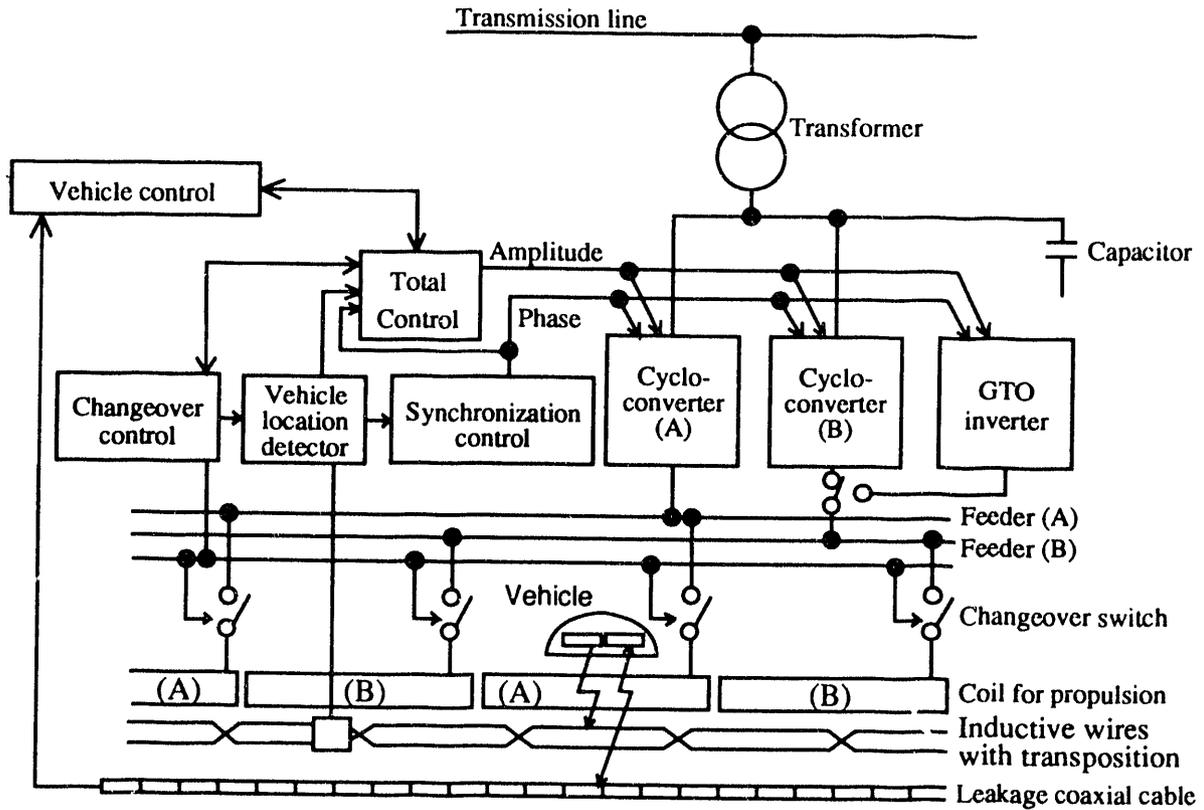
Fig. 1. Power supply system of Miyazaki test track
