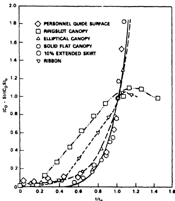
Fig. 5. Drag-area ratio versus dimensionless filling time (Ref. 5).
