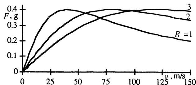
Fig. 4. Typical dynamic braking force vs. velocity for different  $R$
