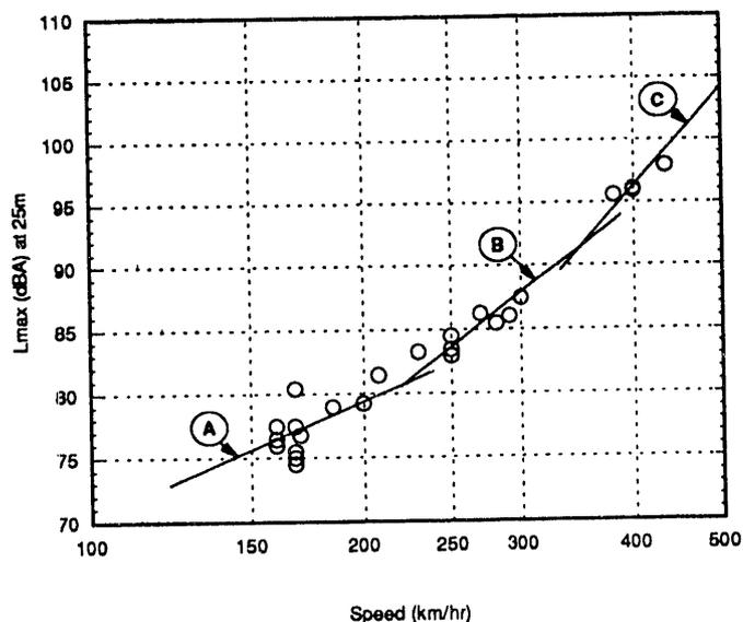
Fig. 2. Measured Noise of TR07 Compared With Estimates
