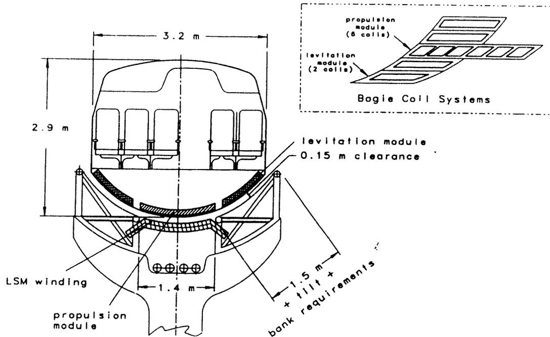
Fig. 1 Vehicle and Guideway Cross Section. Note: typical bogie arrangement.
