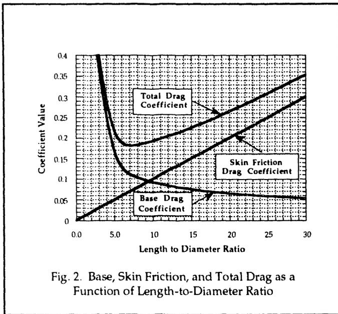
Fig. 2. Base, Skin Friction, and Total Drag as a Function of Length-to-Diameter Ratio
