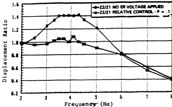
Fig. 9. Experimental transmissibility curves for soft passive and relative damping control algorithm.
