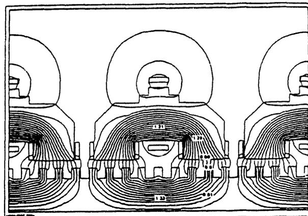
Figure 9: Baseline Magnetic Field Calculations with 2-D Code (Permendur Iron)
