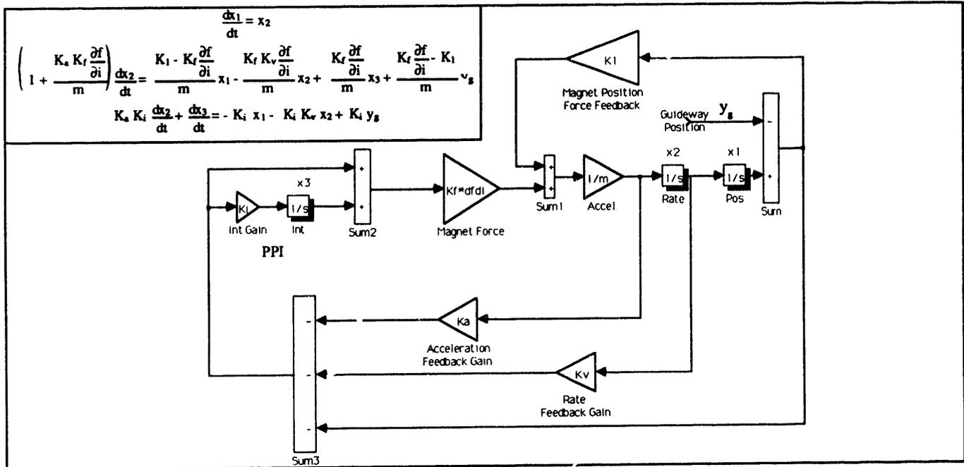
Fig. 1. Block Diagram of Magnet Servo Linear Model
