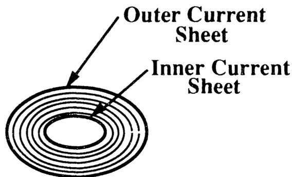
Figure 6 Currents can be distributed around a closed path in such a way as to contain the flux to the interior region
