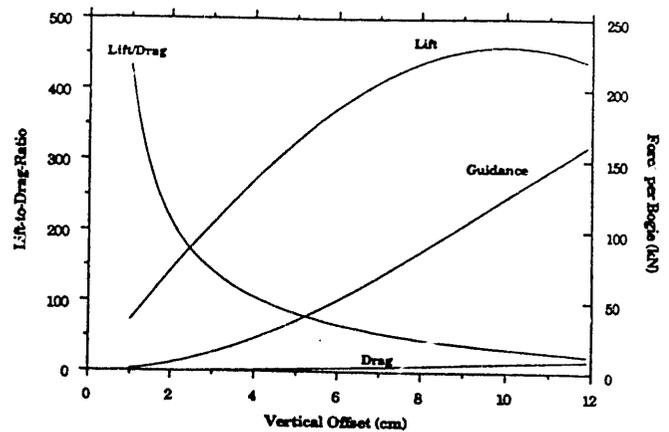
Figure 5. Magnetic Forces vs Vertical Displacements at 134 m/s. 8 rungs/meter; 0.20-m gap; 400 kA-T current; 16 magnets/bogie (ANL)
