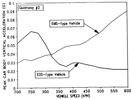
Figure 5. Concrete Box Guideway, 21 m Span, Carbody Vertical Accelerations
