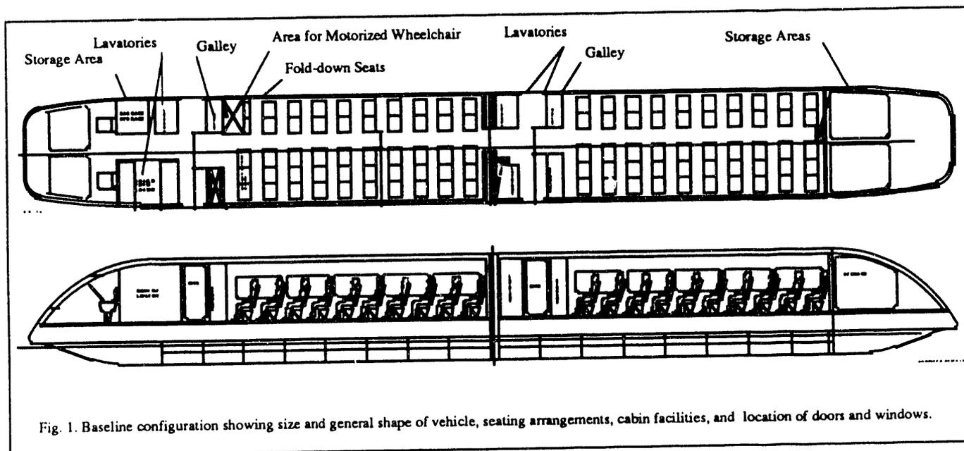
Fig. 1. Baseline configuration showing size and general shape of vehicle, seating arrangements, cabin facilities, and location of doors and windows.
