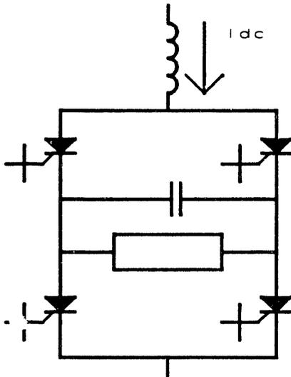
Fig. 4 A PWM Current Source Inverter
