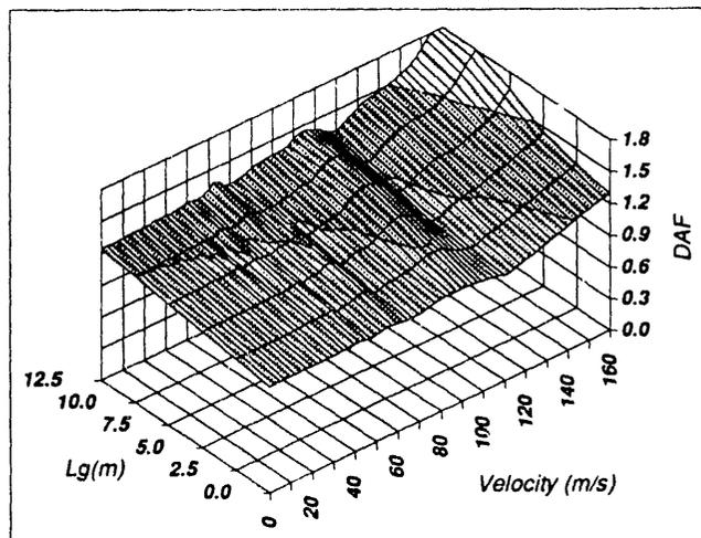
Figure 12. Vehicle Loading Pad Length (DAF)
