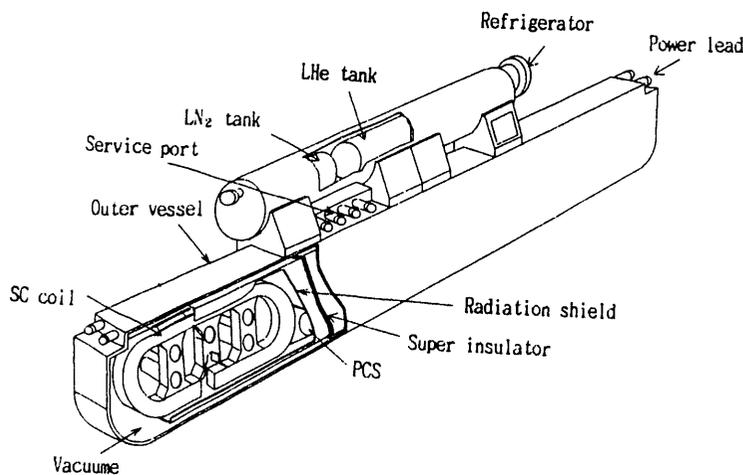
Fig.2 Illustration of the superconducting magnet
