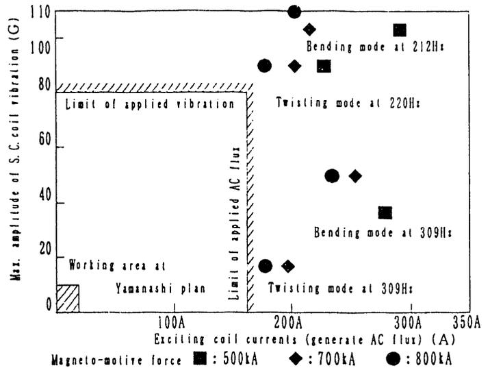
Fig. 7 Typical result of electromagnetic coil vibrating tests
