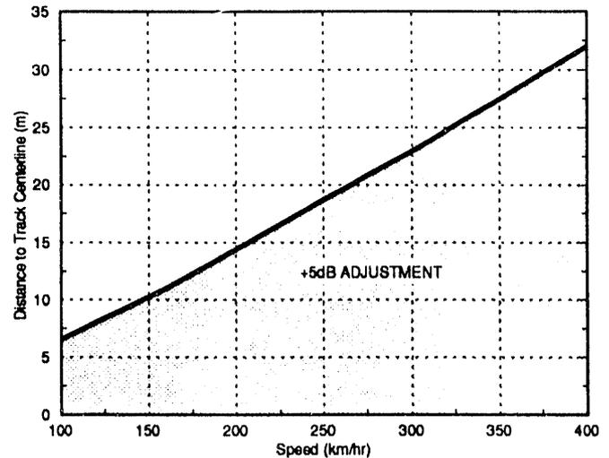
Fig. 6. Onset Rate Adjustment to Maglev SEL
