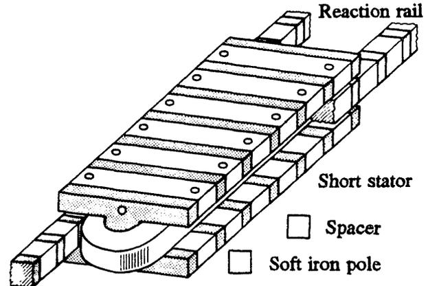
Fig. 6. Transverse flux short-stator motor
