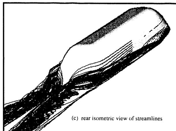
Fig. 7. Flow pattern computed about simplified model.
