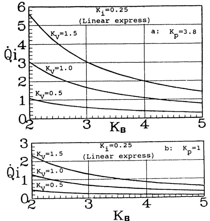
Fig.3. Ratio between the quantities of armature insulating material ( $\dot{Q}_i=Q_{id}/Q_{im}$ ) as a function of the ratio between the average flux densities in the armature plane ( $K_B=B_d/B_m$ ); parameter: ratio between maximum feeding voltages ( $K_v=V_{Md}/V_{Mm}$ ); a:  $K_p=3.8$ ; b:  $K_p=1$ .
