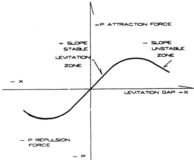
Fig. 2 Definition of positive directions for force +P and displacement +X and MPW characteristic curve of magnetic levitation and/or repulsion force -P vs levitation displacement gap -X obtained with setup fig. 1.
