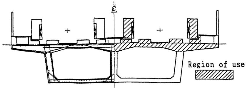
Fig.3 Region of use of low magnetic steel
