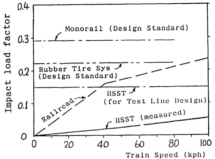
Fig.11 Impact load factor on PC girder
