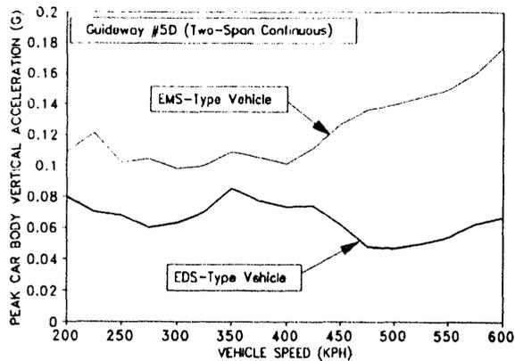
Figure 10. Steel "V" Guideway (Transrapid), Two-Span Continuous Guideway, Carbody Vertical Accelerations
