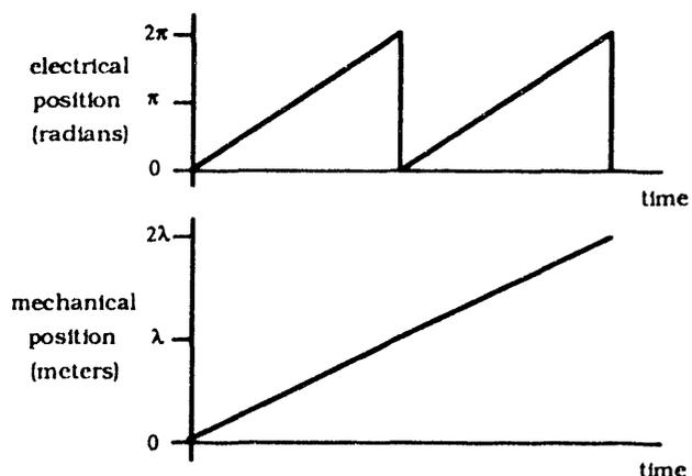
Fig. 3 Comparison of electrical and mechanical position
