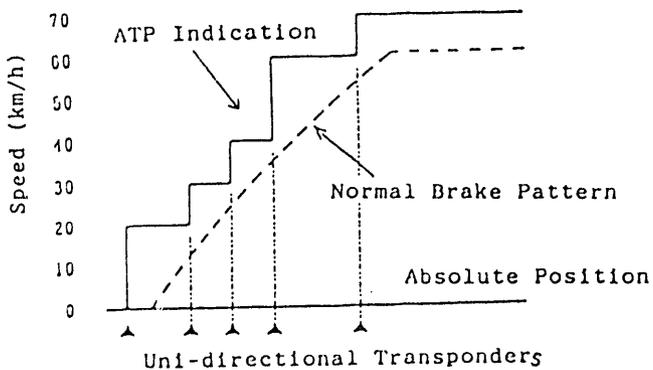
Fig.8 Overrun protection function
