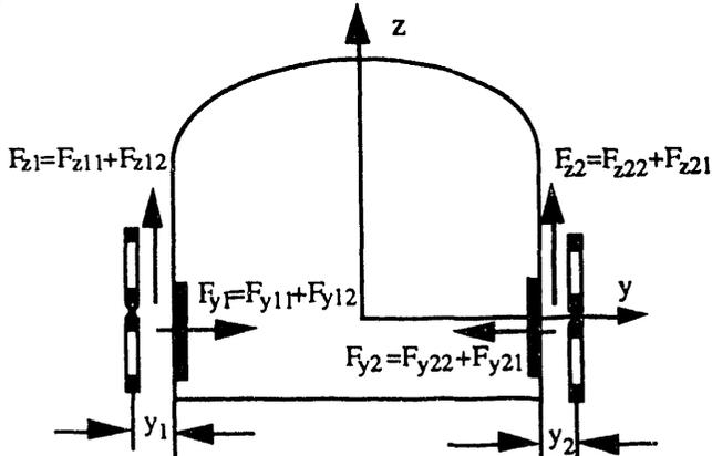
Fig 5 Cross-Sectional View of the Side-Wall Null-Flux Suspension System
