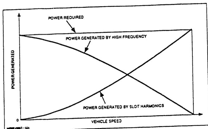
Fig. 4. Control of Power Generation as a Function of Vehicle Speed
