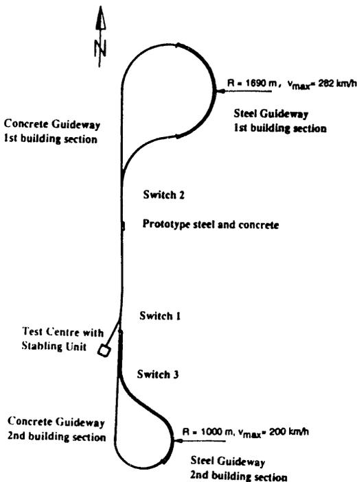
Fig. 1 Test Facility in Emsland
