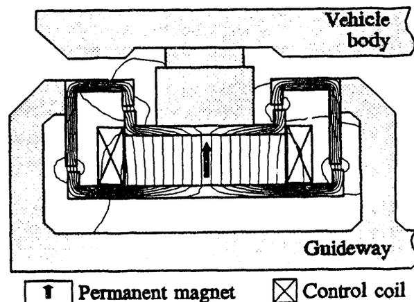
Fig. 2. Magnet with stable guidance force
