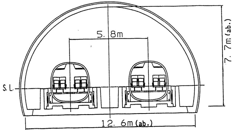
Fig.4 Tunnel cross section
