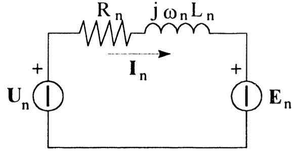
Fig.4 - Single-phase equivalent circuit related to one section of the armature winding.
