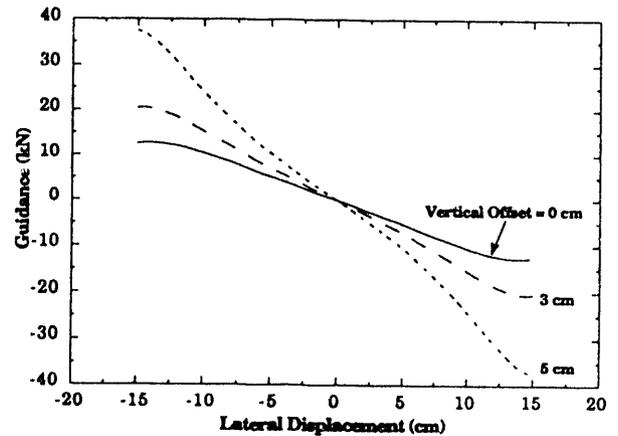
Fig. 10 Total Guidance Force vs Lateral Displacement with Vertical Offset as a Parameter. Speed: 138 m/s; Effective Gap: 20 cm; Vertical Offset: 3 cm. (Ref. Table 1)
