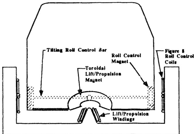
Figure 4 Stage three vehicle cross-section
