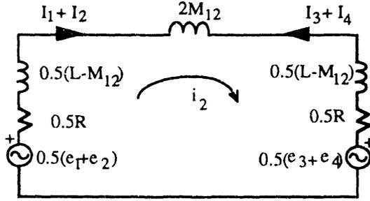
Fig. 4 Simplified Equivalent Circuit for Determining Null-Flux Guidance Force
