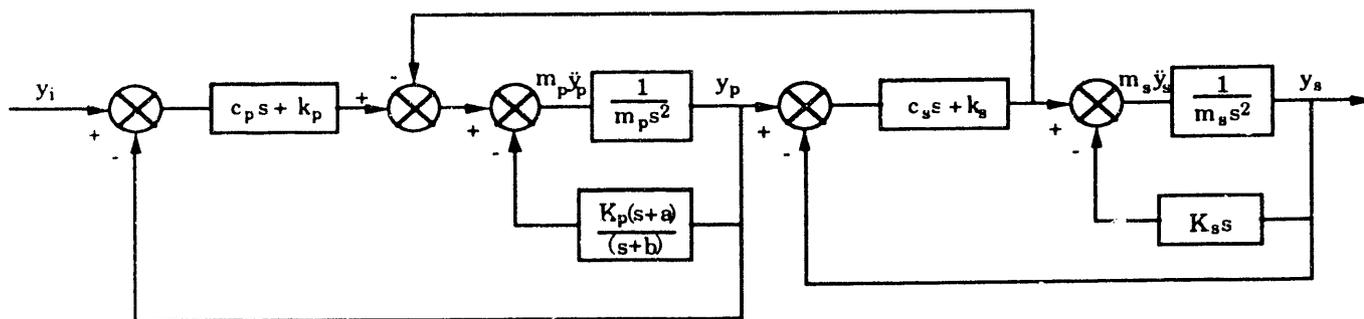
Fig. 7. Block diagram for two-degree-of-freedom vehicle model of maglev system with primary and secondary suspension feedback controls.
