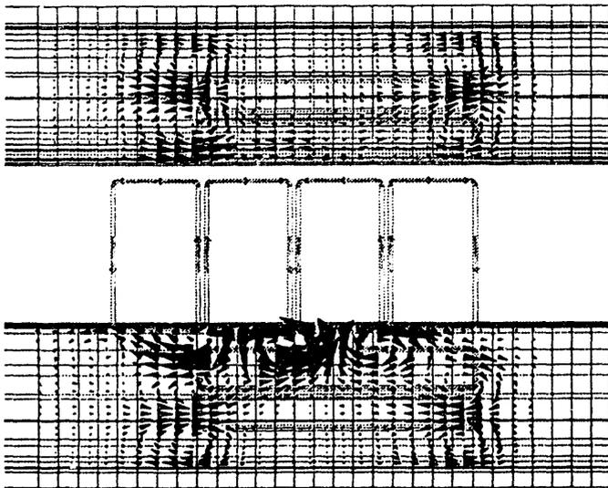
Figure 14. Eddy Current Pattern Induced in Guideway by Magneplane-Type System, with Levitation Magnets but only Four Propulsion Coils.
