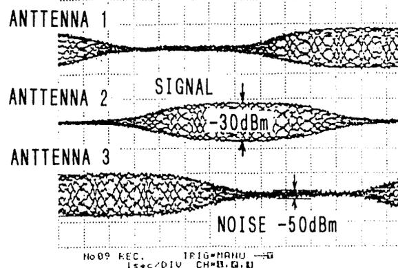
Fig. 7 Speed signal receiving level
