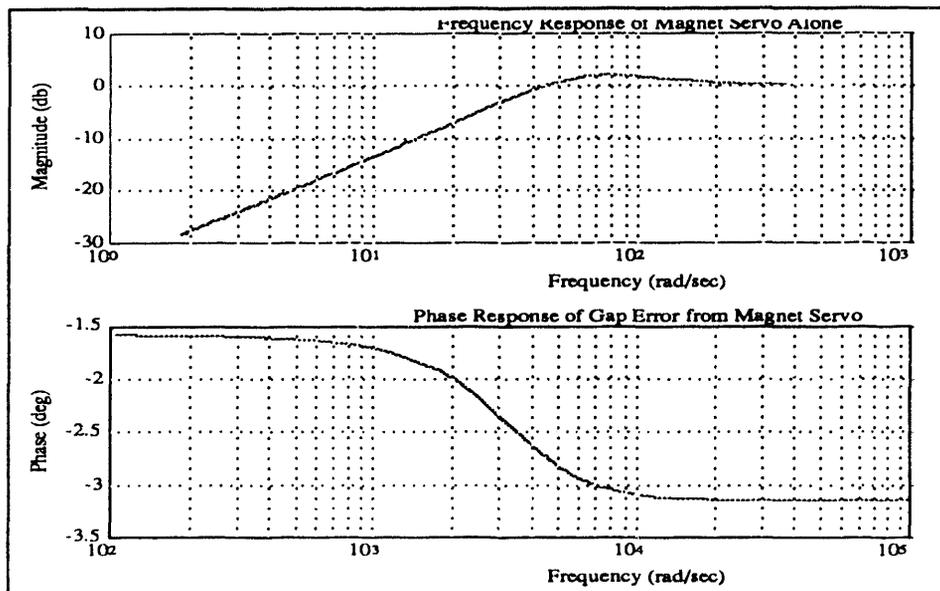
Fig. 3. Frequency Response Plot of the Position to Gap Error Transfer Function for the Magnet Servo
