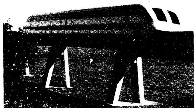
Fig.1 TRANSRAPID 07 on TVE elevated guideway
