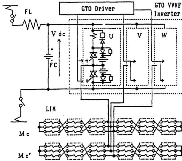
Fig.1 Main Circuit Connection Diagram
