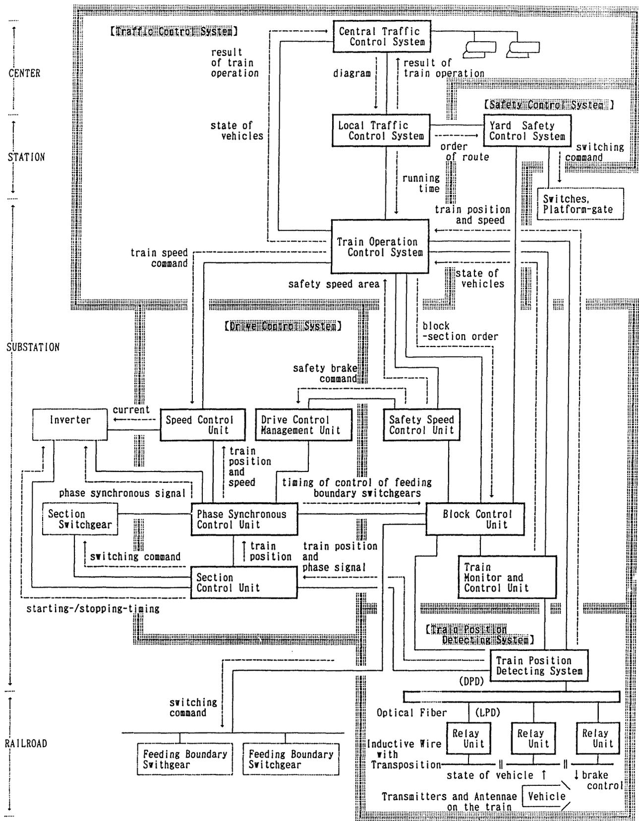
Fig. 2. Structure of the Train Control System
