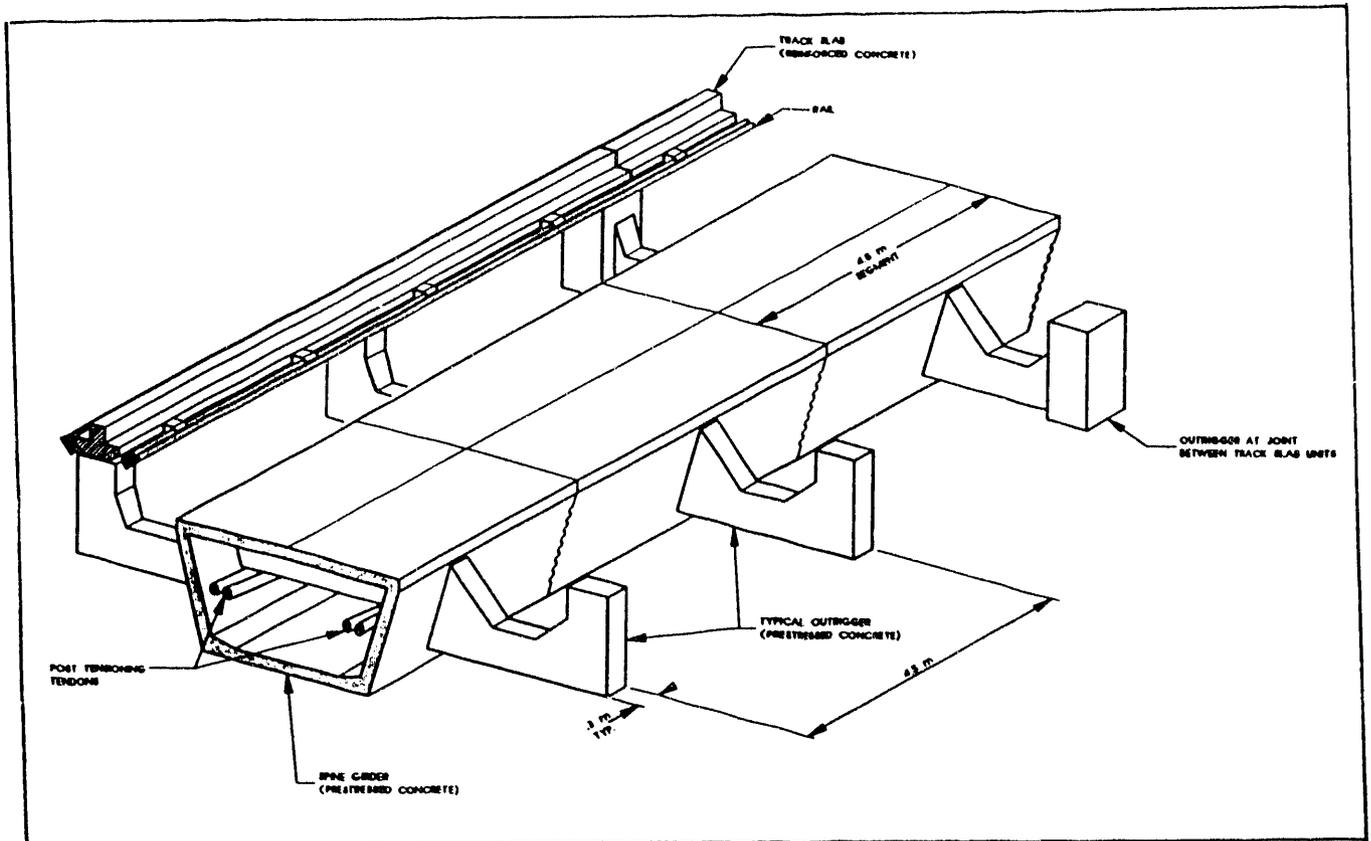
**Figure 4. Isometric Showing the Box Girder Outrigger-Layout and Post-tensioning Cables**
