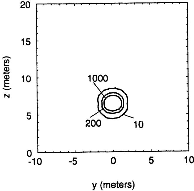
Fig. 5. Magnetic Field From LSM Winding in mG
