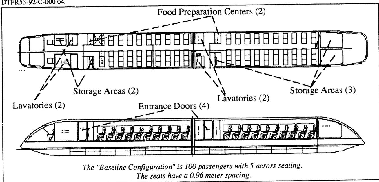
Fig. 1 . Grumman baseline Maglev vehicle configuration
