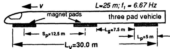
Figure 6. Three Pad Vehicle,  $S_p = 12.5 \text{ m}$  ( $L_v = 30 \text{ m}$ )
