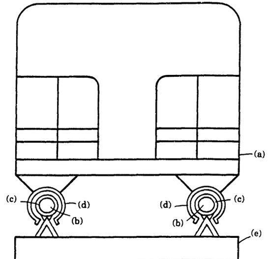
**Fig. 1:** Proposed Maglev System with energization from the wayside.
