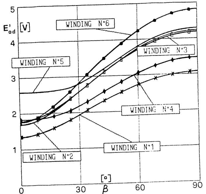
Fig.6. No-load rectified voltages  $E'_{od}$  of the 6 windings of fig.5, as a function of  $\beta$ .
