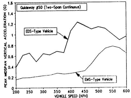
Figure 18. Steel "V" Guideway (Transrapid), Two-Span Continuous Guideway, Mid-Span Vertical Beam Accelerations.
