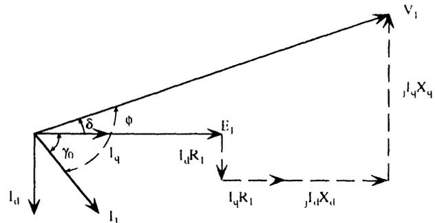
Fig. 7. Iron Core LSM Phasor Diagram for Lagging Power Factor
