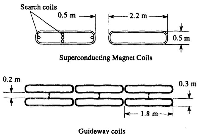
Figure 3. Coil configurations
