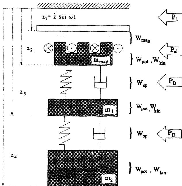
Fig. 1: Energy balance of an electromagnetic support system
