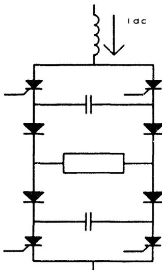
Fig. 3 The ASCI quasi-square wave CSI.
