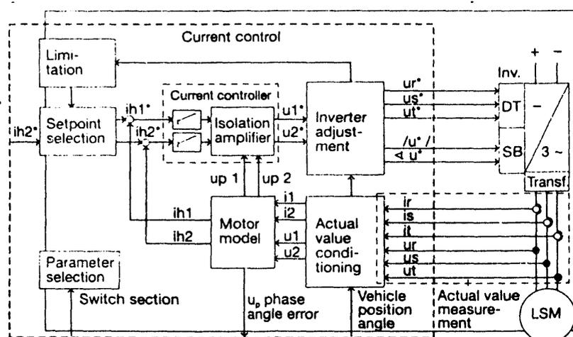
Fig. 5. Block diagram of digital current control
