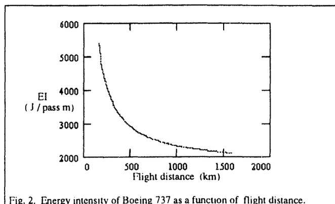
Fig. 2. Energy intensity of Boeing 737 as a function of flight distance.
