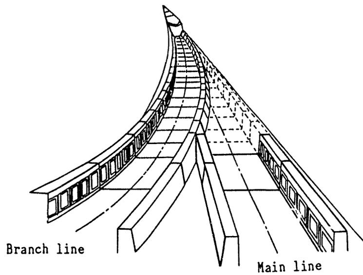
Fig. 5 Turnout of a traverse type
