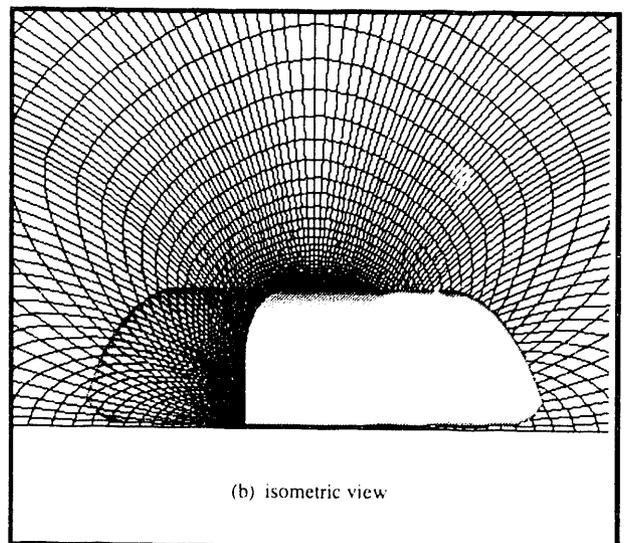
Fig. 4. Computational grid at mid-section of simplified model.
