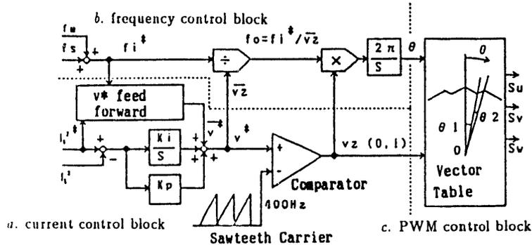
Fig.3 Control Block Diagram
