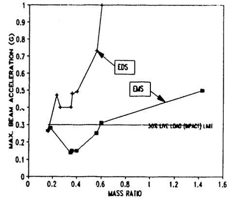
Figure 20. Maximum Accelerations vs. Mass Ratio for Responses between 100 to 400 km/h
