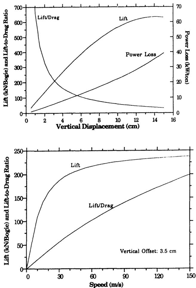
Figure 1. Suspension force vs vertical offset at 134 m/s (top) and vs speed with 0.035 m offset (bottom). Gap = 0.275 m, Velocity = 34 m/s, Current = 1800 kA-T, Conductor cross-section = 16 cm<sup>2</sup>.
