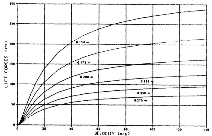
Figure 12. Lift Forces Calculated for Two Sets of Two Magnets on a Single Bogie of the Baseline 45-Passenger Vehicle. Magnets 2.25 m long, 0.4 m wide, 0.1 m spacing. (ANL)
