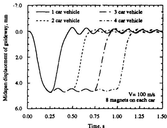
Fig. 2. Midspan displacements of guideway for multicar vehicles with eight magnets on each car and traveling along the guideway at 100 m/s.
