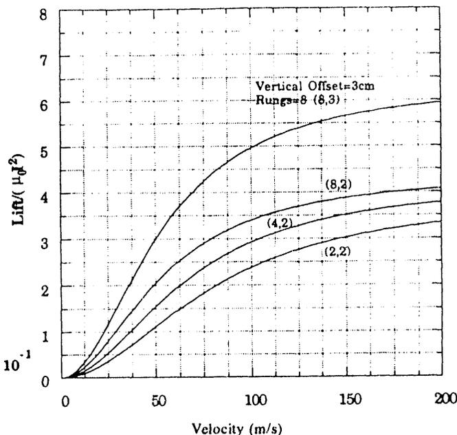
Figure 3. Normalized Lift vs Speed with Number of Rungs and Vertical Offset as Parameters (ANL). See text for parameters.
