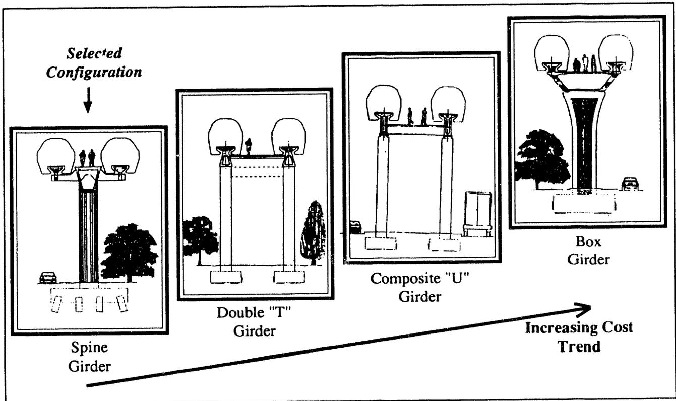
Fig. 7. Alternate guideway structures considered
