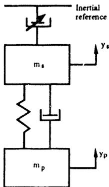
Fig. 8. Skyhook damper for secondary suspensions.
