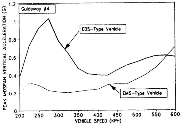
Figure 15. Twin Concrete Box Beam Guideway (HSST), 21 m Span, Mid-Span Vertical Beam Accelerations
