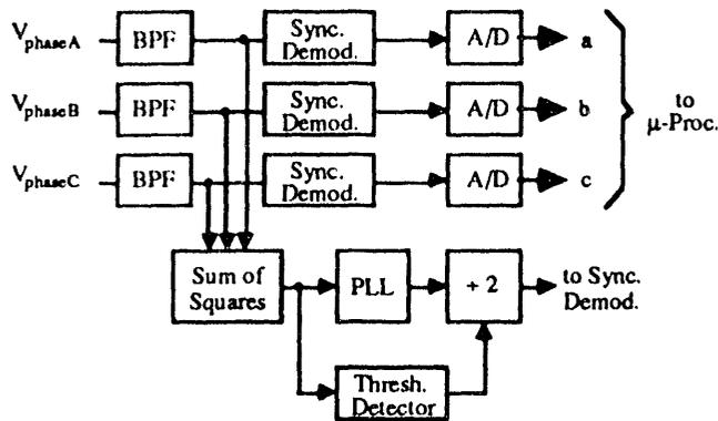
Fig. 7 Block diagram of demodulator circuitry
