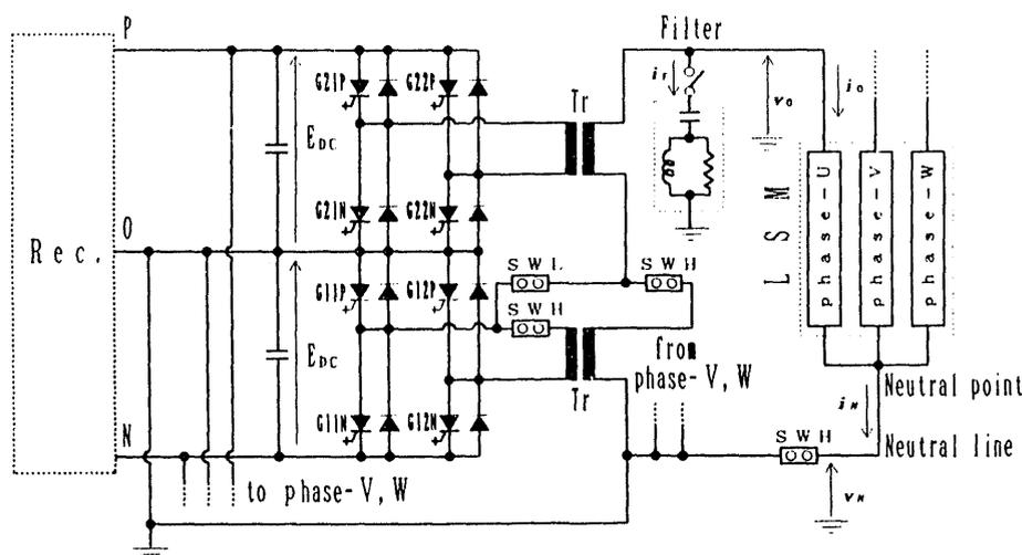
Fig. 3 Main circuit of PWM inverter for Miyazaki test track
