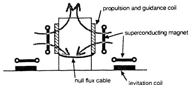
Fig. 1. Inverted T type guideway
