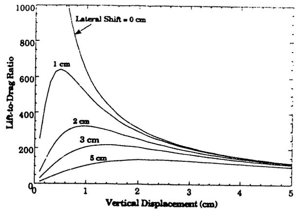
Fig. 9 Lift-to-Drag Ratio Profile as a Function of Vertical Displacement with Lateral Offset as a Parameter. Speed: 138 m/s; Effective Gap: 20 cm. (Ref. Table 1)
