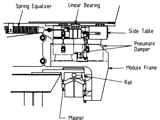
Fig. 7. Secondary Suspension
