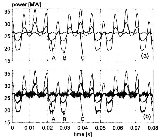
Fig.7 - Power vs. time for the three proposed strategies in the case of ideal (a) and actual (b) inverter.
