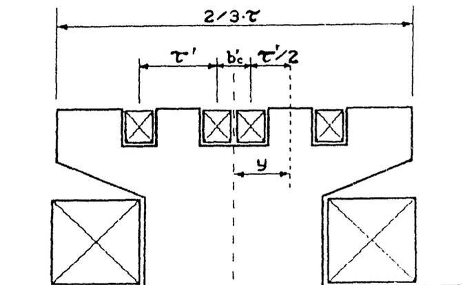
Fig.7. Double single-phase winding with adjacent coils arranged in three slots.
