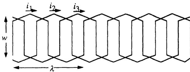
Fig. 2. One conductor per slot, 3-phase meander winding.
