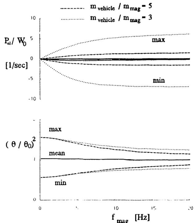
Fig. 3: Influence of the cut-off frequency to the energy exchange
