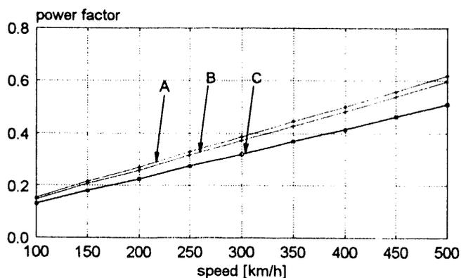
Fig.10 - Power factor versus speed for the three proposed strategies.
