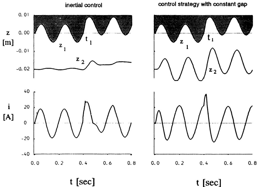
Fig. 7: Simulated behavior of the inertial gap control
