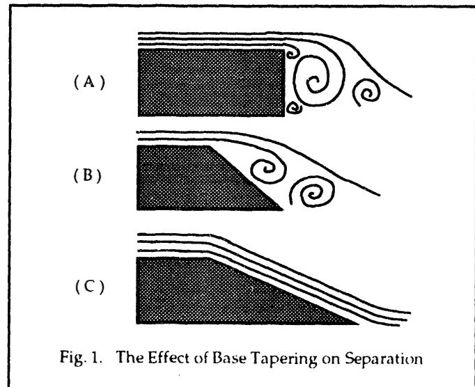
Fig. 1. The Effect of Base Tapering on Separation
