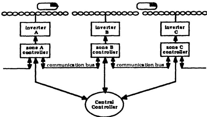
Fig. 1 Hierarchical control architecture
