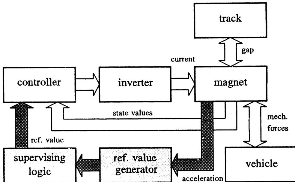
Fig. 6: Block diagram of the inertial gap control
