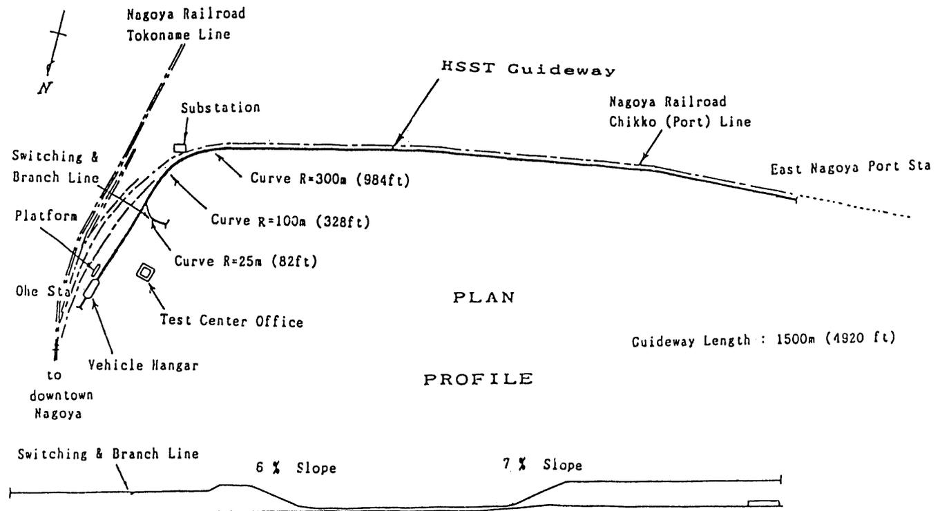
Fig.1 Plan and profile of test line
