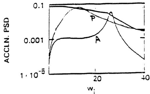
Fig. 5. Acceleration PSD for the secondary mass (for an EDS system with Null-flux guideway)  $\zeta_2 = 1.2$  and  $A = 10^6$  m. (UTACV standard and active response Aa) and passive response (P)
