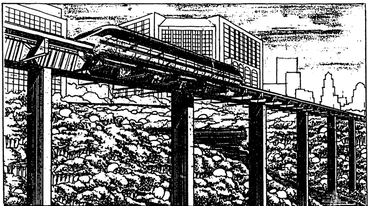
**Figure 5. An artist rendering showing relationship of track slab and outriggers to the central concrete box girder guideway.**
