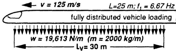
Figure 3. Fully Distributed Vehicle Loading
