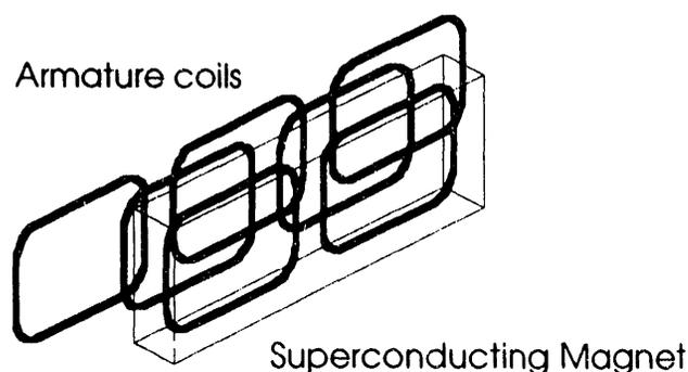
Fig. 1. Structure of a superconducting synchronous motor.
