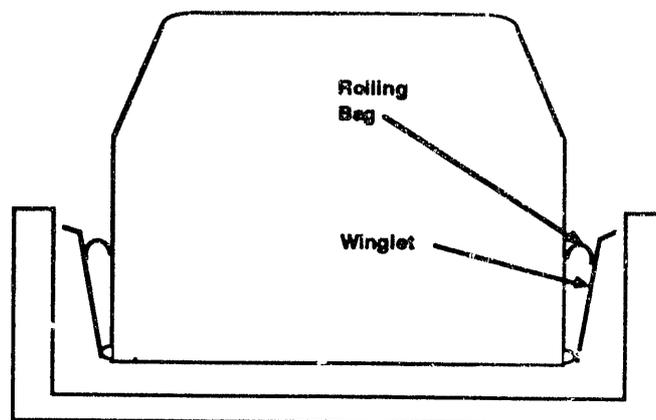
Fig. 1 Stage One Vehicle Cross-section
