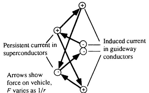
FIG. 6. 2-D MODEL OF SIDEWALL NULL-FLUX EDS.
