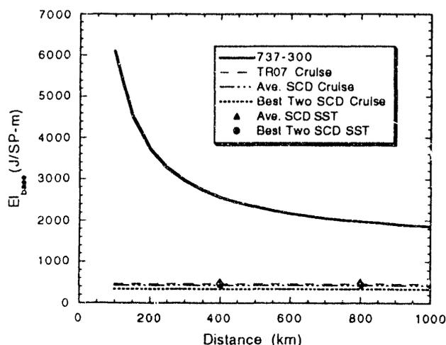
Fig 1. Base energy intensity at system connection (airport or electrical supply)
