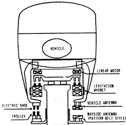
Fig. 13 Layout of the girder structure and the signal systems in the test track
