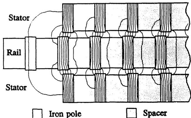
Fig. 8. Flux plot of reluctance motor in longitudinal-section
