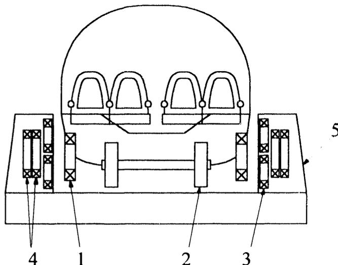
**Fig.1** - Schematic cross section of an EDS-MAGLEV vehicle. [1: on-board SC coils; 2: auxiliary suspension; 3: ground levitation coils; 4: two-layer armature coils; 5: guideway]
