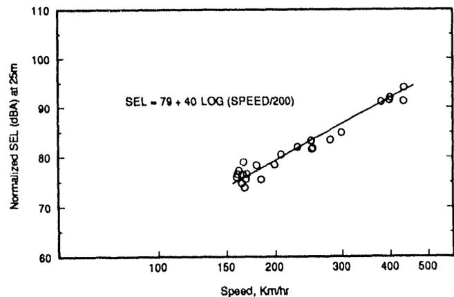
Fig. 4. SEL of TR07 Normalized to Single Vehicle
