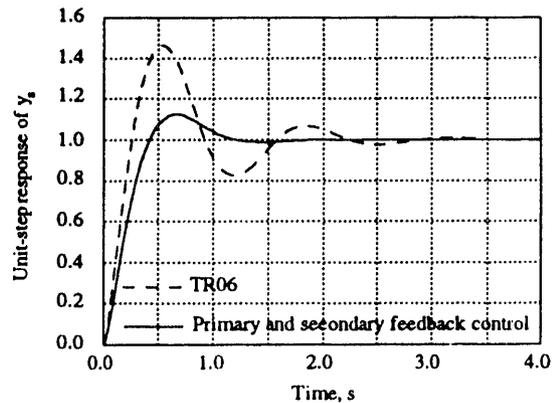
Fig. 11. Comparison of transient response  $y_s$  of secondary suspension with unit-step input of guideway perturbation for TR06 and a new system using active and semiactive feedback controls in primary and secondary suspensions.
