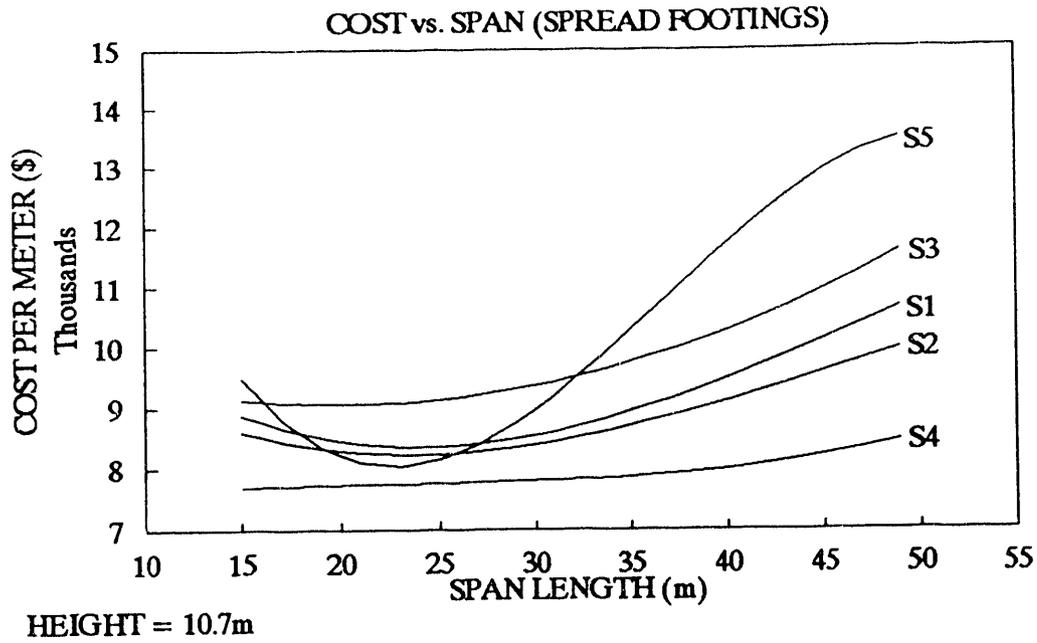
**Figure 2. Results of the parametric cost analysis for the guideway**
