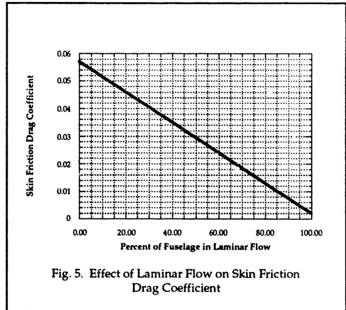
Fig. 5. Effect of Laminar Flow on Skin Friction Drag Coefficient
