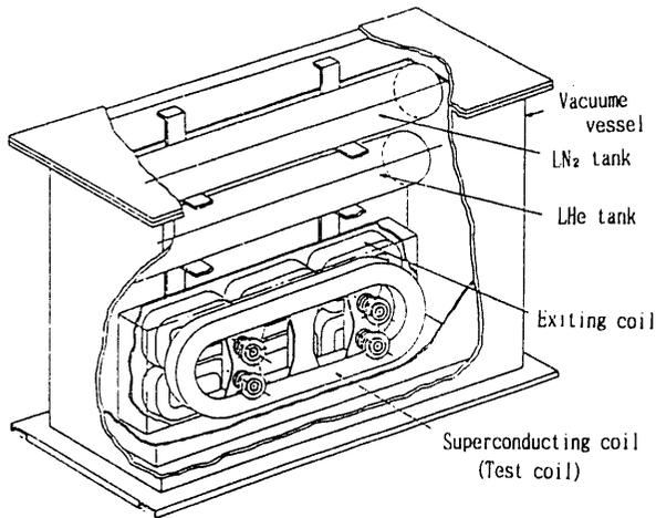
Fig. 6 Electro-magnetical coil vibrating test facility
