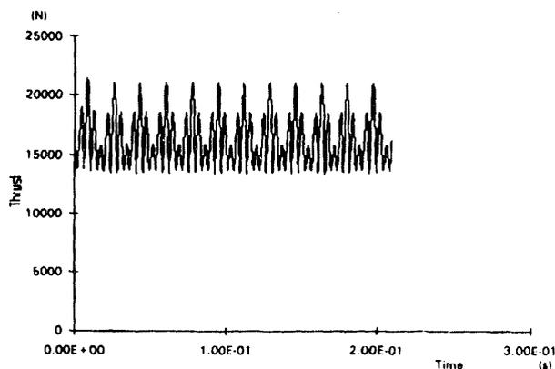
Fig. 5. Instantaneous thrust vs. time in a double layered structure
