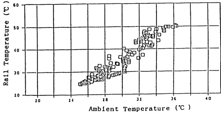
Fig.9 Rail Temperature vs Ambient Temperature
