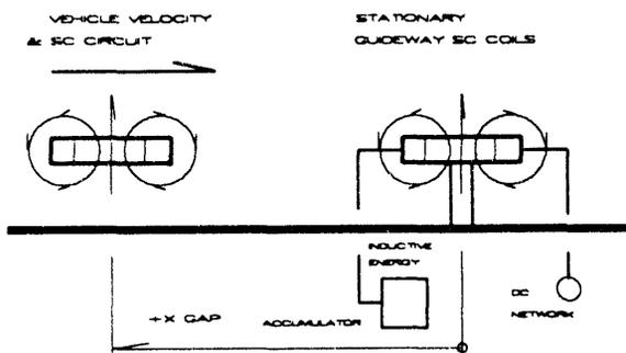
Fig. 3 Illustrates a hypothetical MPW linear motor and guideway configuration concept postulated by Kozoriz [1-5].
