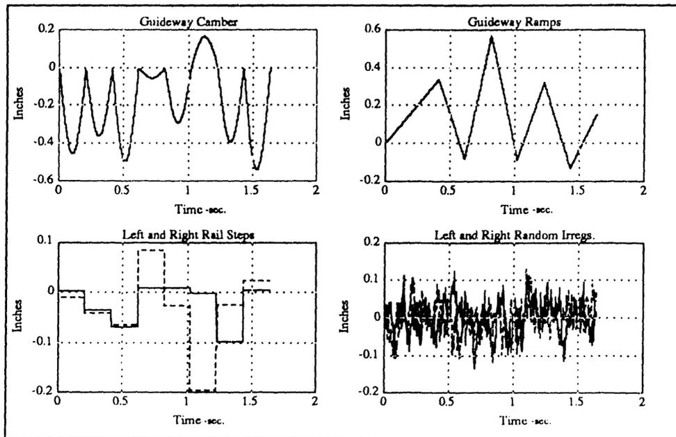
Fig. 8. Guideway Irregularities - Camber, Ramps, Steps and Random
