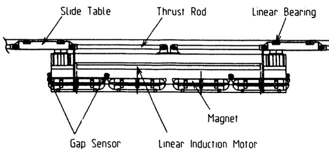
Fig. 5. Module Assembly
