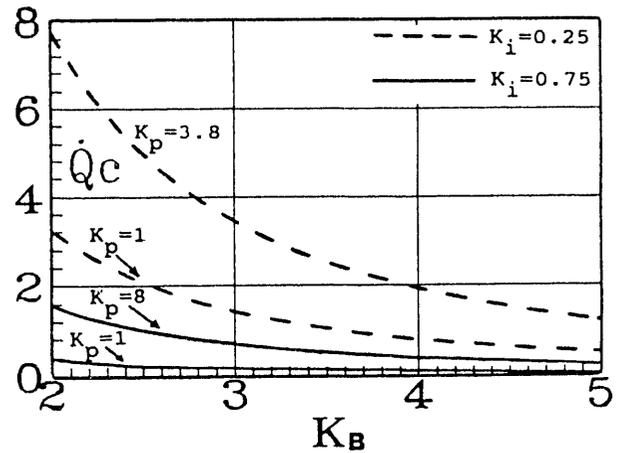
Fig.2. Ratio between the quantities of conductive material ( $Q_c=Q_{cd}/Q_{cm}$ ) as a function of the ratio between the average flux density within the armature plane ( $K_B=B_d/B_m$ ); parameters: polar pitch ratio ( $K_p=\tau_d/\tau_m$ ) and ratio between the inductor lengths ( $K_i=L_{id}/L_{im}$ ).
