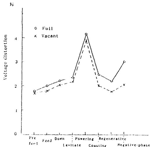
Fig. 5 The harmonic voltage distortion at the receiving end
