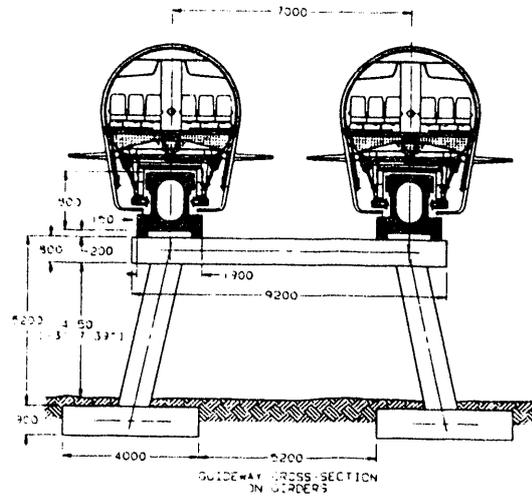
Fig. 1 Vehicle/Guideway Cross Section
