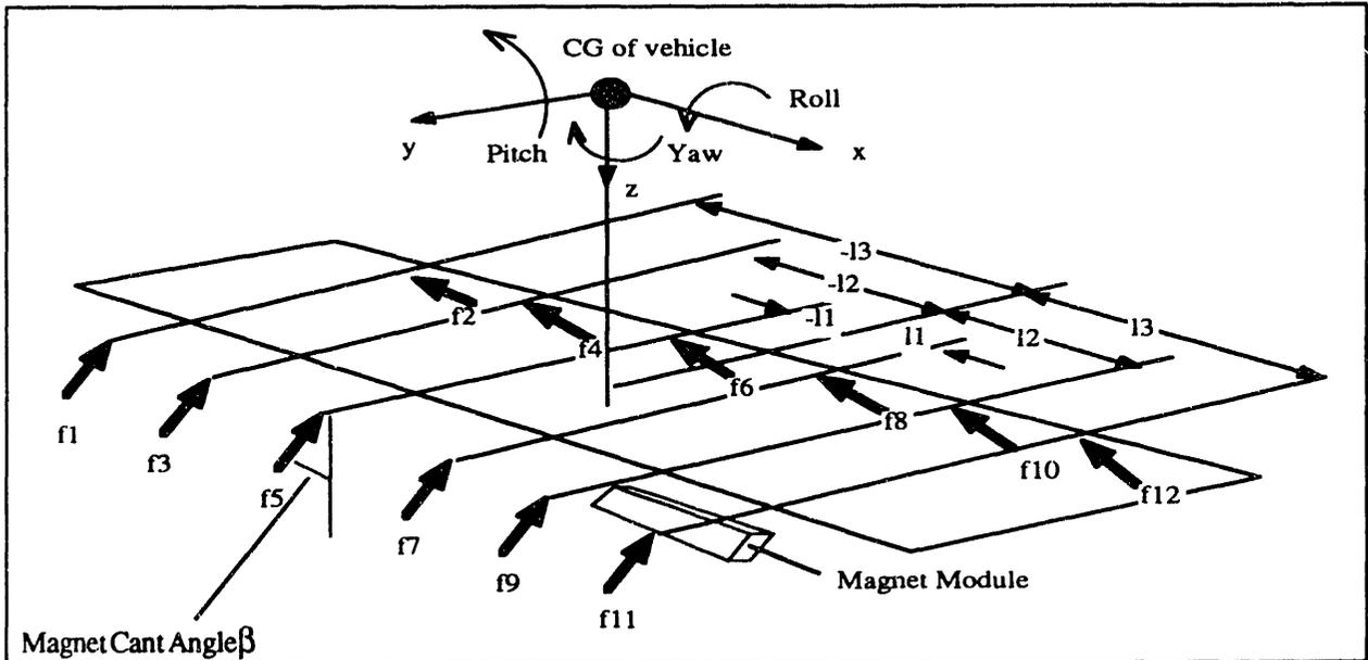
Fig. 5. Forces and Moments Created by 12 Magnet Modules
