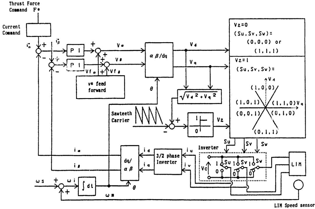
Fig.5 HSST-100 Control Block Diagram
