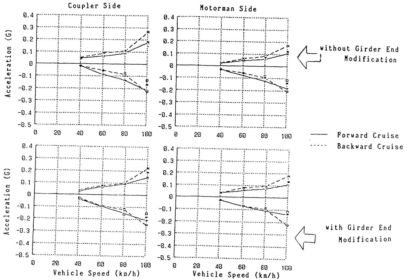
Fig.3 Maximum Acceleration of Car Body in Girder Deflection Test
