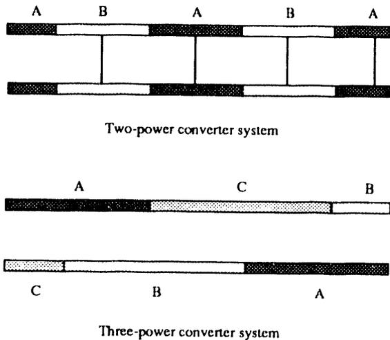
Fig. 2. Feeding Arrangement for propulsion coils
