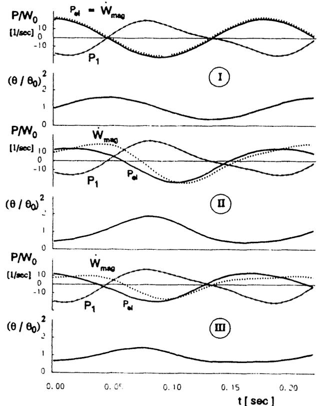
Fig. 2: Time behavior of the energy exchange at a sinusoidal track disturbance
