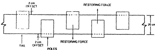
Figure 8. Position of Magnet Poles on Guideway Rail (LSM Stator) to Provide Stability Against Lateral Motion. (Grumman)
