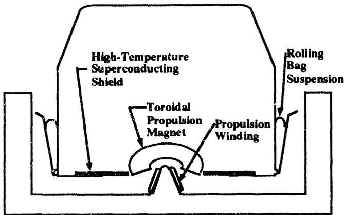
Figure 3 Stage two vehicle cross section
