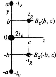
FIG. 8. 2-D MODEL OF FLUX CANCELING SUSPENSION.
