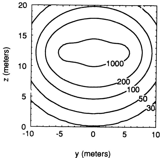
Fig. 3. Magnetic Field From a Transmission Line in mG
