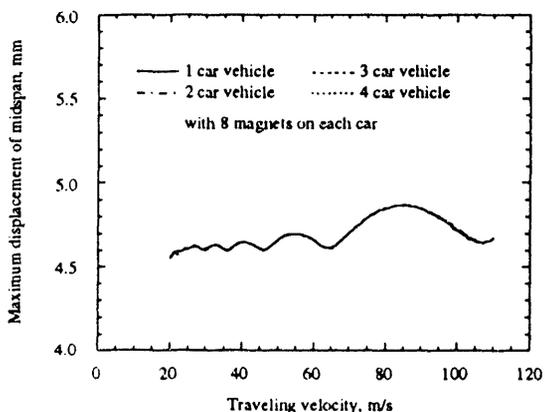
Fig. 3. Maximum midspan displacements of guideway when multicar vehicles with eight magnets on each car travel along the guideway at various speeds.
