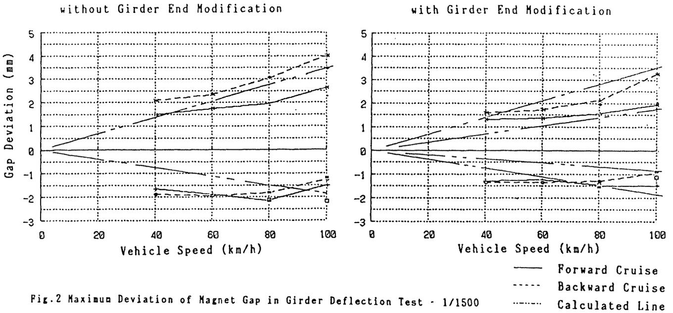
Fig.2 Maximum Deviation of Magnet Gap in Girder Deflection Test - 1/1500
