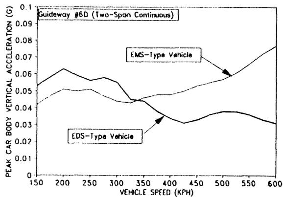
Figure 11. AASHTO Concrete Girders, Two-Span Continuous Guideway, Carbody Vertical Accelerations
