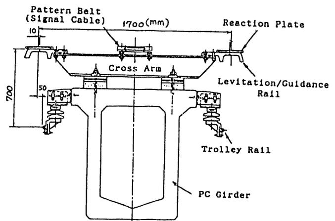
Fig.4 Cross section of guideway (standard)
