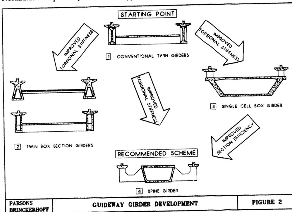
Conventional twin I girders (1) were the starting point. Although they have been used on low speed guideways, the girders have poor torsional stiffness which makes them unsuitable for curved track. As well, it is difficult to integrate the emergency evacuation slab into the section.
