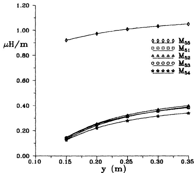
Fig. 4 - Self- and mutual inductances (for 1 turn)  $M_{55}$ ,  $M_{51}$ ,  $M_{52}$ ,  $M_{53}$ ,  $M_{54}$  versus levitation height.
