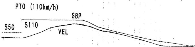
Fig. 8 Automatic operation following the normal-braking pattern
