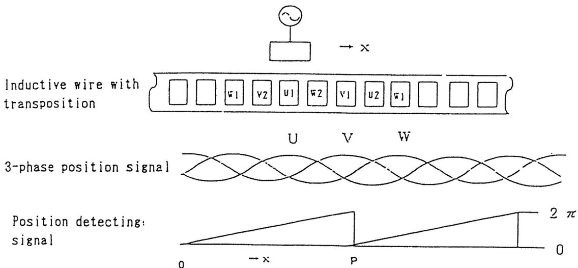
Fig.3. Principle of train position detection
