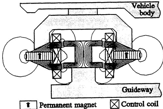
Fig. 1. Magnet with stable support force
