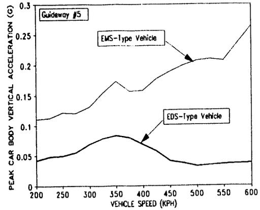
Figure 7. Steel "V" Guideway (Transrapid) 21 m Span, Carbody Vertical Accelerations
