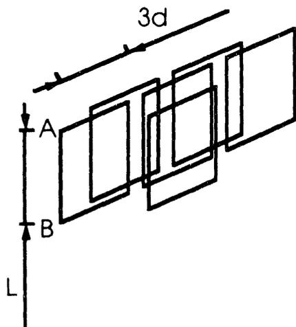
Fig. 2. Simplified model of synchronous motor for Maglev.
