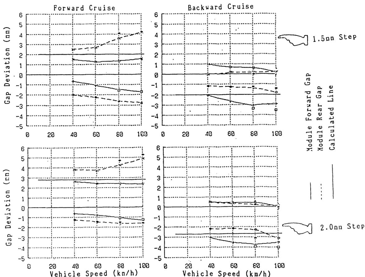
Fig.5 Maximum Deviation of Magnet Gap in Vertical Step Test
