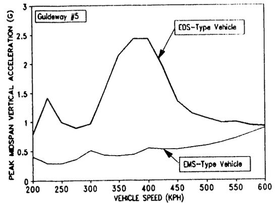
Figure 16. Steel "V" Guideway (Transrapid), 21 m Span, Mid-Span Vertical Beam Accelerations
