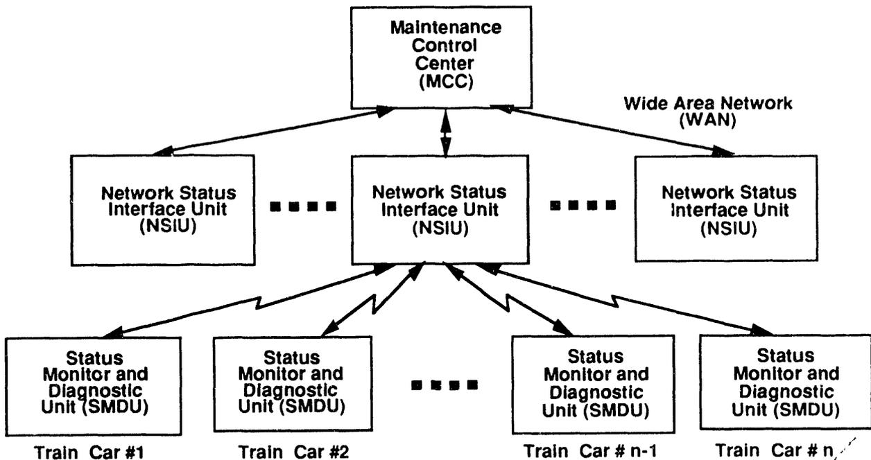
Figure 1. Automated Preventive Maintenance System Block Diagram
