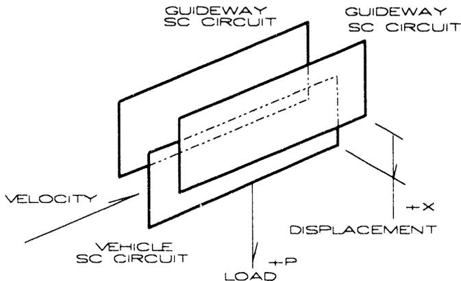
Fig. 5 Coordinate system for the case of a free vehicle with roof mounted rectangular superconducting circuit, magnetically suspended in a gravity field in the equilibrium position, below a sidewall guideway consisting of two SC circuits, Kozoriz [1-5].
