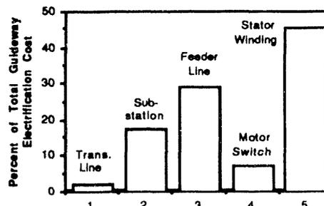
Fig. 3 Distribution of guideway electrification costs
