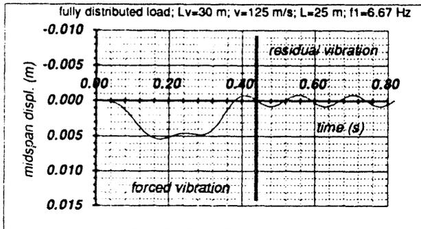
Figure 4. Beam Response (Fully Distributed Load)
