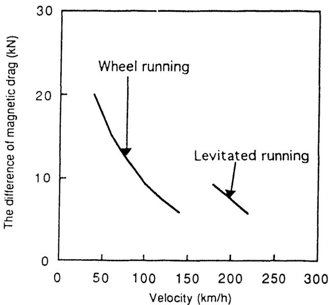
Fig. 3. The difference of magnetic drag
