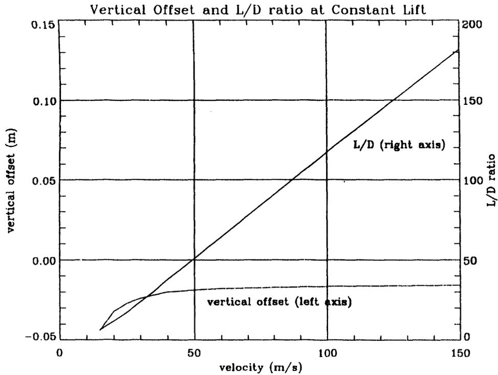
Fig. 1 - Plot of magnetic lift to drag ratio, L/D, (solid curve, right-side vertical scale), and vertical offset (dashed curve, left-side vertical scale), as a function of speed, at constant lift, for the Type I concept vehicle. Horizontal clearance, 0.145 m. Vertical offset is measured relative to horizontal plane of symmetry of guideway ladder.
