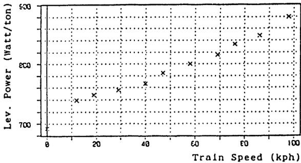
Fig.7 Levitation Power Consumption (per train weight)
