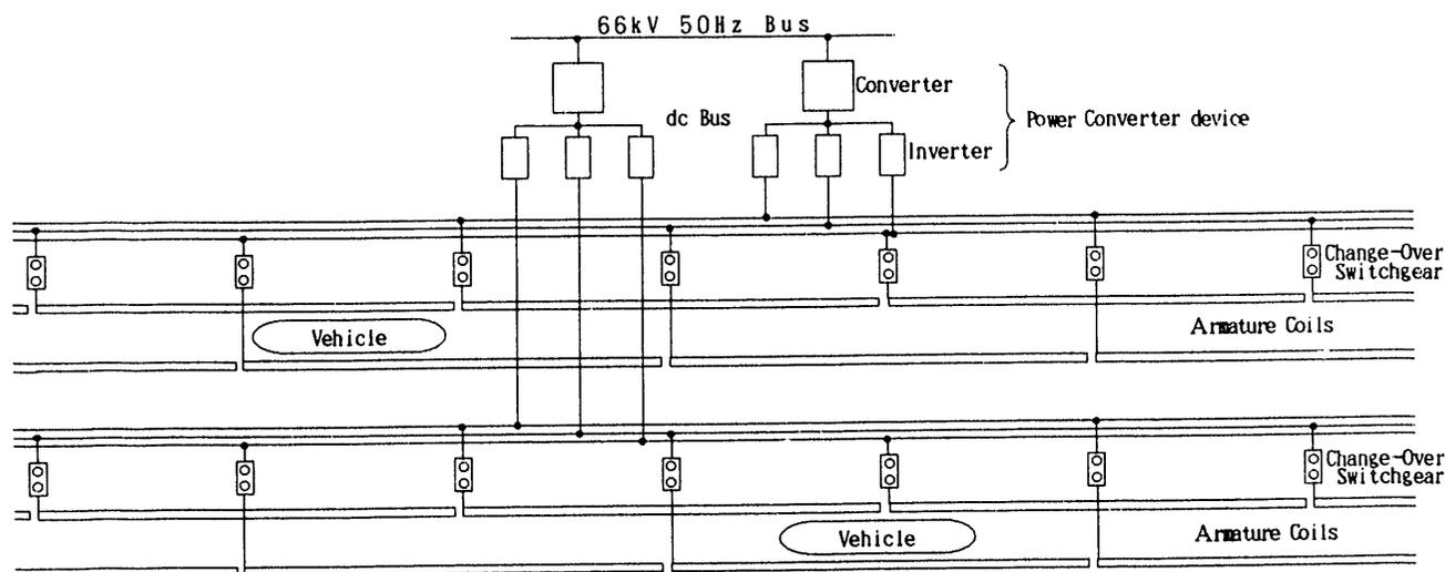
Fig.1 Power Supply System at the New Test Track
