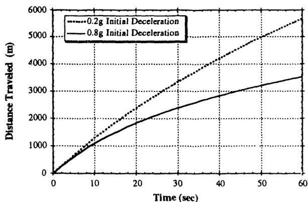
Fig. 7. Distance traveled by Maglev vehicle after drag chute deployment.
