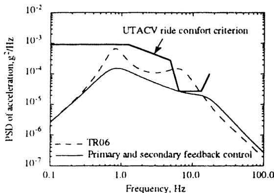
Fig. 9. PSD of vehicle acceleration using active and semiactive feedback controls in primary and secondary suspensions, with vehicle speed  $V = 100$  m/s and guideway roughness amplitude  $A = 10^{-6}$  m.
