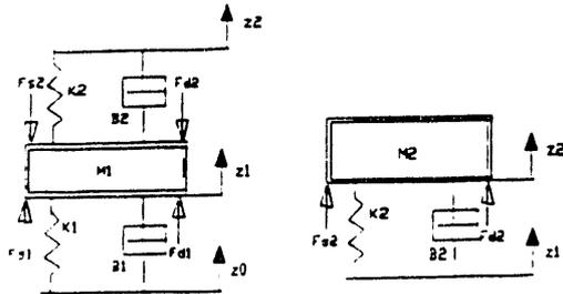
Fig. 2. Free body diagrams for (a) bogie mass and (b) car body mass in bounce mode (gravitational effects cancelled by initial spring forces).
