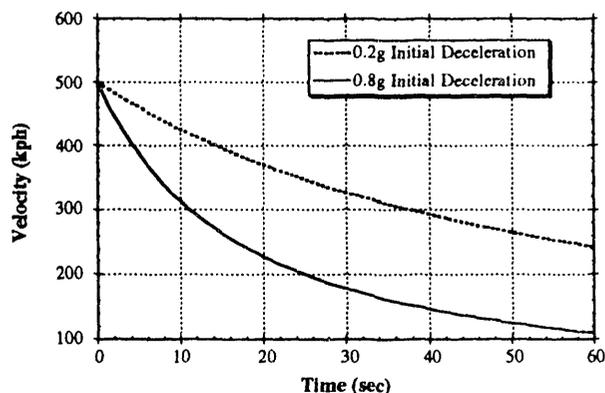
Fig. 6. Velocity of Maglev vehicle after drag chute deployment.
