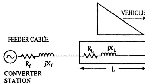
Fig. 9. Schematic of Power Supply to an LSM Block
