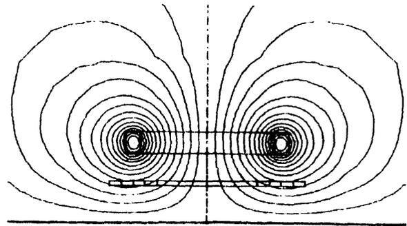
Fig. 3 - Plot of the flux distribution due to the superconducting coil,  $y = 0.25$  m,  $d=0.10$  m.
