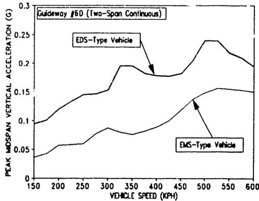
Figure 19. AASHTO Concrete Girders, Two-Span Continuous Guideway, Mid-Span Vertical Beam Accelerations
