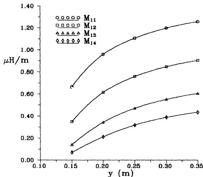
Fig. 5 - Self- and mutual inductances (for 1 turn)  $M_{11}$ ,  $M_{12}$ ,  $M_{13}$ ,  $M_{14}$  versus levitation height.
