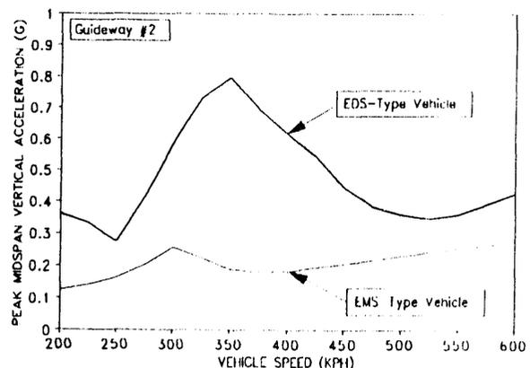
Figure 13. Concrete Box Guideway, 21 m Span, Mid-span Vertical Beam Accelerations
