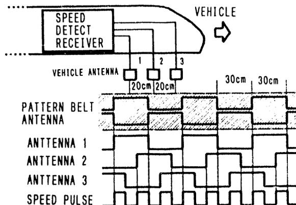
Fig. 6 Speed-detection pattern and output logic
