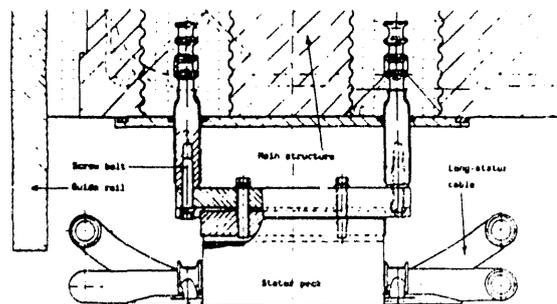
Fig. 6 Stator mountings TVE concrete guideway northern loop (one mounting axle)
