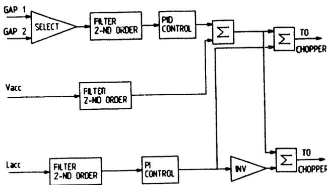
Fig. 8. Levitation Controller Block Diagram
