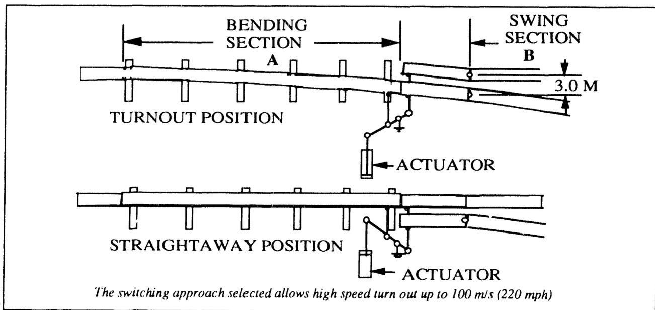
Fig. 9. Off-line switching concept
