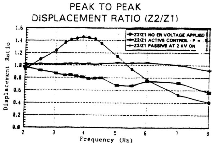
Fig. 8. Experimental transmissibility curves for soft and stiff passive and semiactive control concepts using ER fluids.
