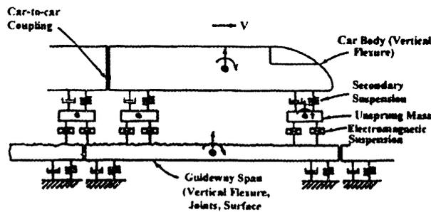
Model of EDS-Type Vehicle on Guideway
