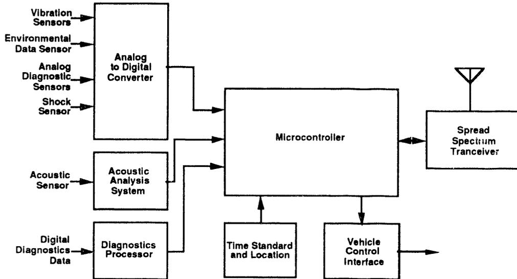
Figure 2. Status Monitor Diagnostic Unit Block Diagram
