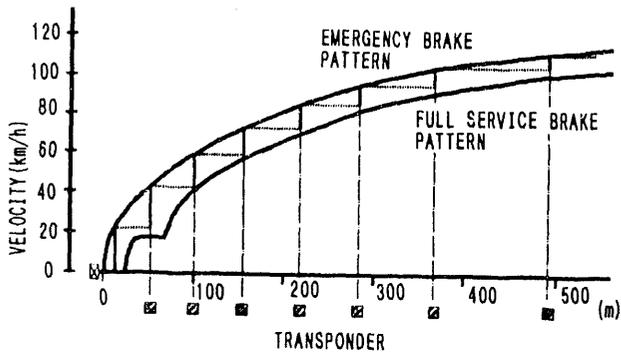
Fig. 2 ATP braking pattern
