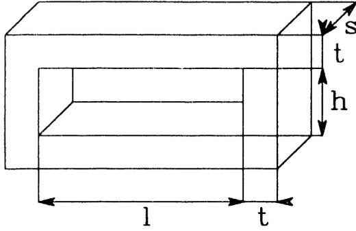
Fig.3 - Reference dimensions of armature and field coils, with number of turns respectively  $N_f$  and  $N_s$ .
