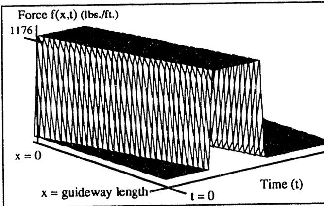
Fig. 6. Force applied to guideway as vehicle moves across
