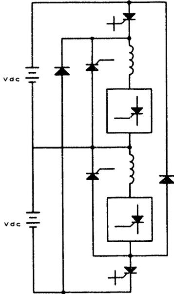
Fig. 7 A chopper with unidirectional I, bidirectional V.
