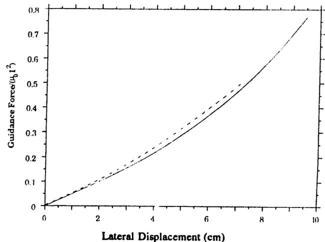
Figure 6. Normalized Guidance Force vs Lateral Displacement (cm). Four Magnets Each Side. Solid Curve (ANL); Broken Curve (Bechtel).
