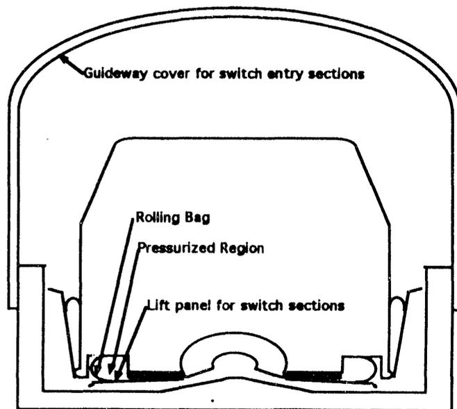
Figure 8 -- Entry section of stage two switch concept
