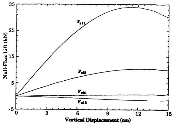
Fig. 6 Null-Flux Lift Force Components as a Function of Vertical Displacement. Speed: 138 m/s; Effective Gap: 20 cm; Lateral Shift: 5 cm. (See Table 1 for Other Parameters)
