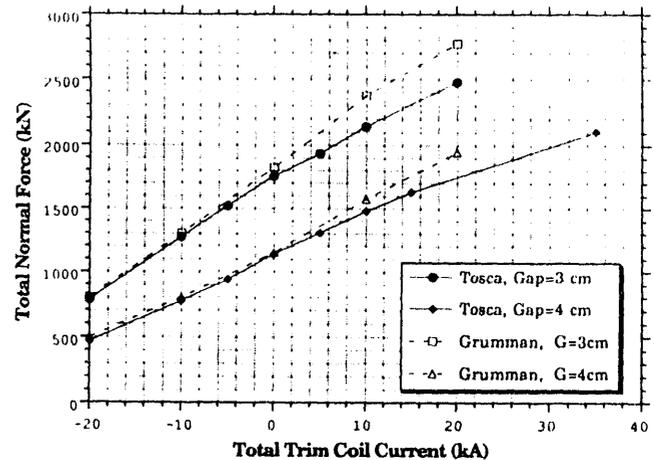
Figure 9. Total Force Normal to Face of Magnets. Current in Superconducting Magnets = 50 kA-T. Total Current in Both Trim Coils as Variable. (ANL/Grumman)
