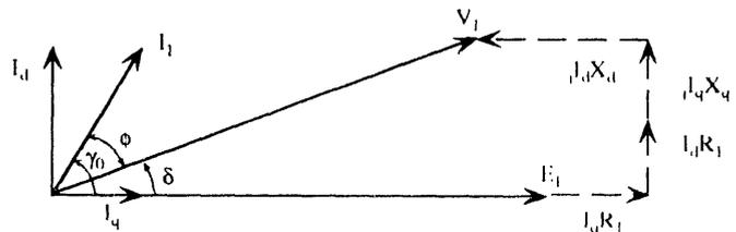
Fig. 8 Iron Core Phasor Diagram for Leading Power Factor
