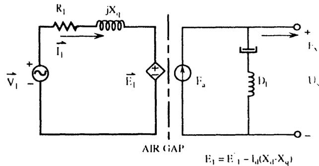
Fig. 5. Equivalent Circuit Model for the Linear Synchronous Motor
