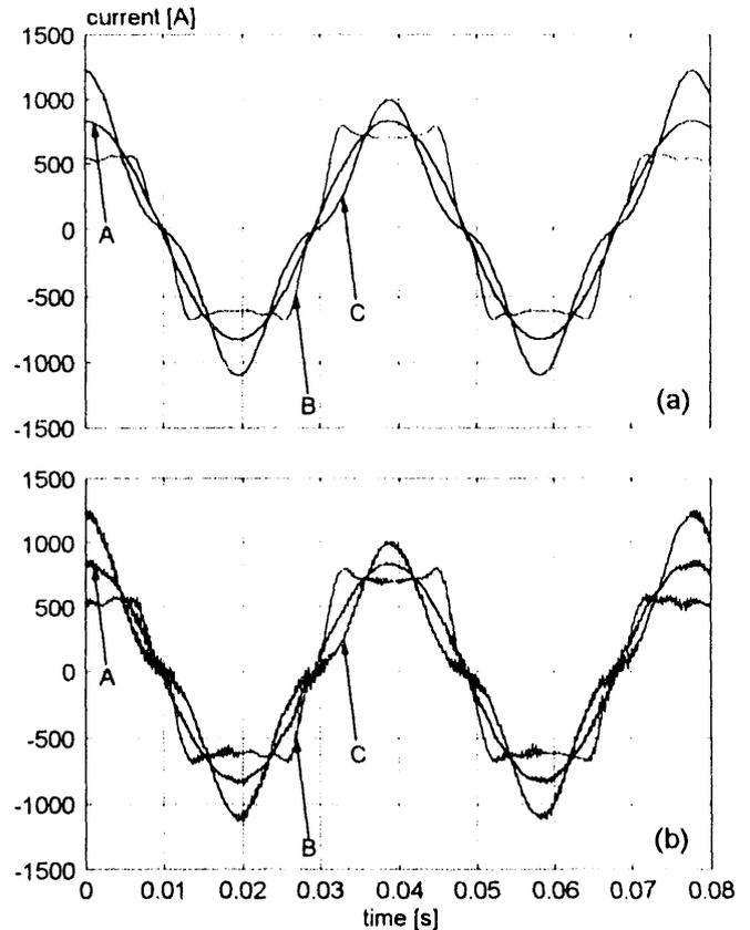
Fig.6 - Current vs. time for the three proposed strategies in the case of ideal (a) and actual (b) inverter.
