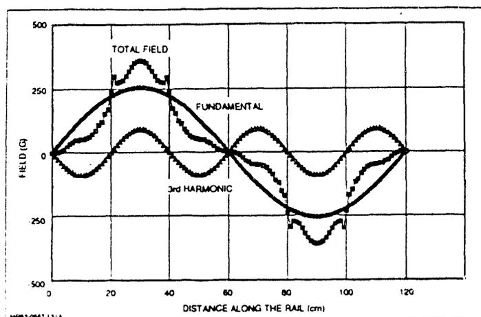
Fig. 3 Field Produced by 600 Hz Rail Current at the Poleface
