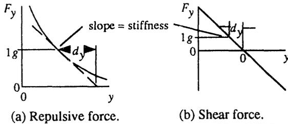
FIG. 4. TWO TYPES OF STIFFNESS THAT ARE POSSIBLE.
