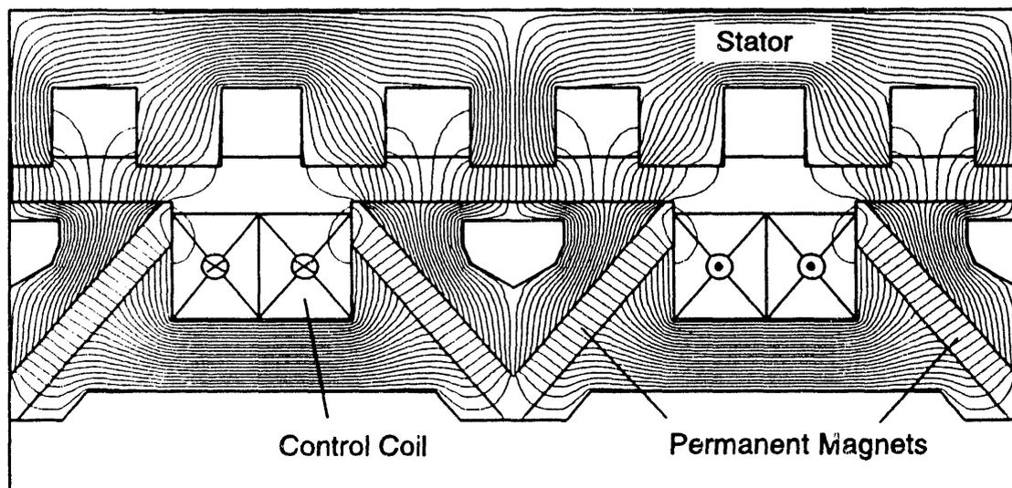
Fig. 5: Permanent magnetic excited suspension system (longitudinal section)
