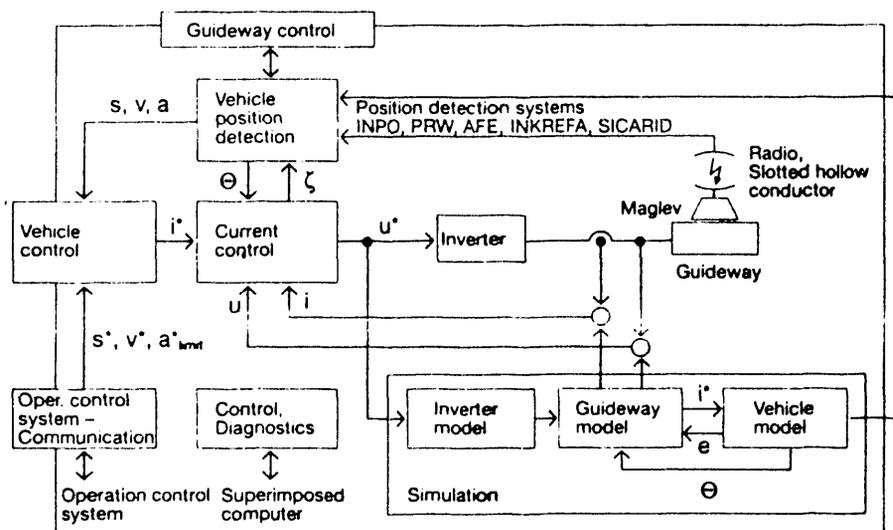
Fig. 4. Block diagram of digital drive control
