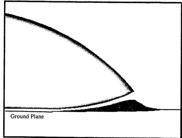
Fig. 9. Reverse flow region at aft end of simplified model.
