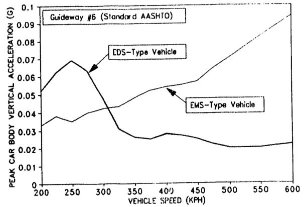
Figure 8. AASHTO Concrete Girders, 21 m Span, Carbody Vertical Accelerations
