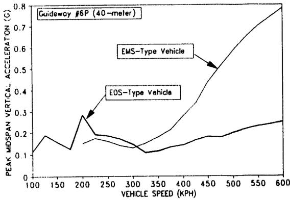
Figure 14. AASHTO Concrete Girders, 40 m Span, Mid-Span Vertical Beam Accelerations
