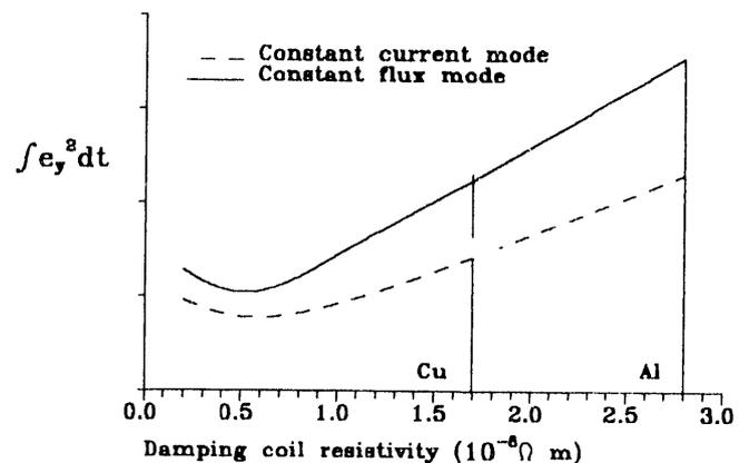
Fig. 10 - Performance index versus damping coil resistivity.
