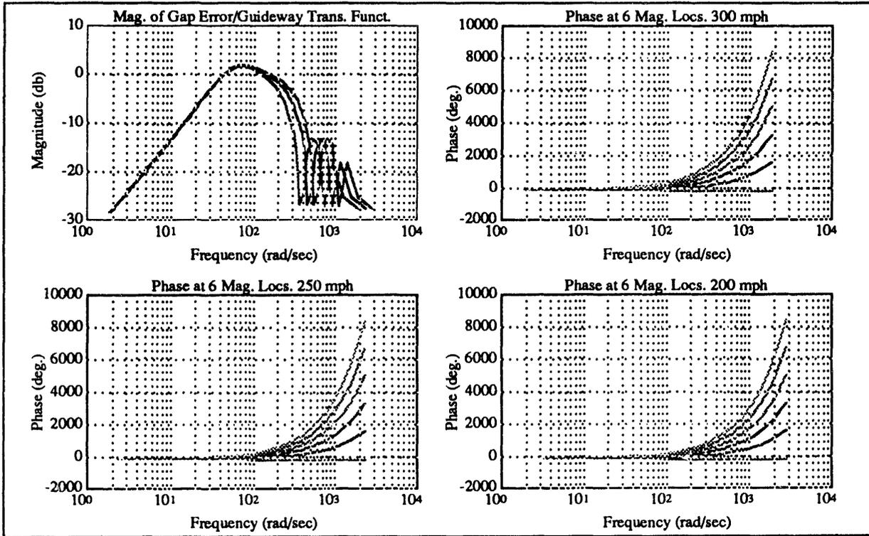
Fig. 4. Transfer Functions for Different Speeds and Magnet Module Locations
