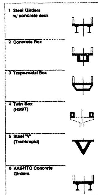
Fig. 2. Selected Guideway Structures
