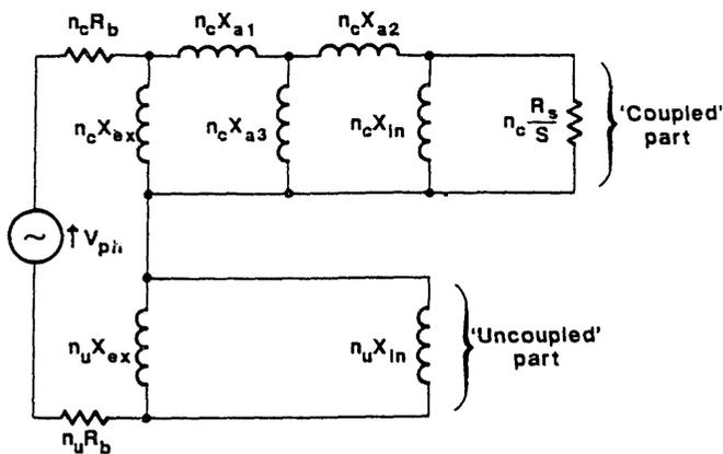
Fig. 4: Single-phase equivalent circuit of an air-cored, linear induction motor.
