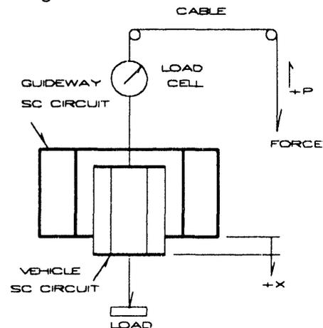
Fig. 1 Schematic sketch of MPW magnetic physics laboratory experimental setup at Academy of Sciences of Ukrainian SSR, Kozoriz [1-5].
