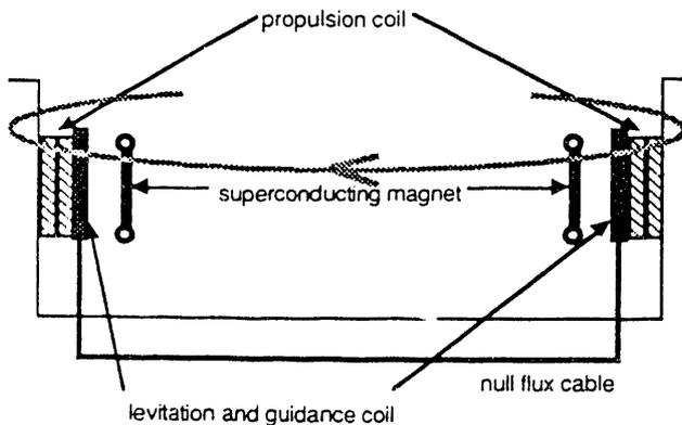
Fig. 5. Null-flux levitation + double layered propulsion system
