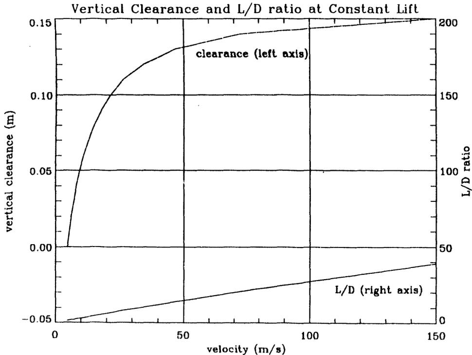
Fig. 2 - Plot of magnetic lift to drag ratio, L/D, (solid curve, right-side vertical scale), and vertical offset (dashed curve, left-side vertical scale), as a function of speed, at constant lift, for the Type II concept vehicle. Vertical clearance, 0.15 m, measured from sheet guideway surface to vehicle bottom surface.
