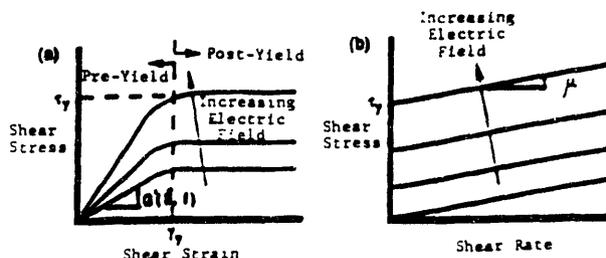
Fig. 1. Typical rheological behavior of an ER material denoting the pre- and post-yield material behavior.
