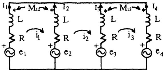
Fig. 3 Equivalent Circuit for the Cross-Connected Null-Flux Coil Suspension System
