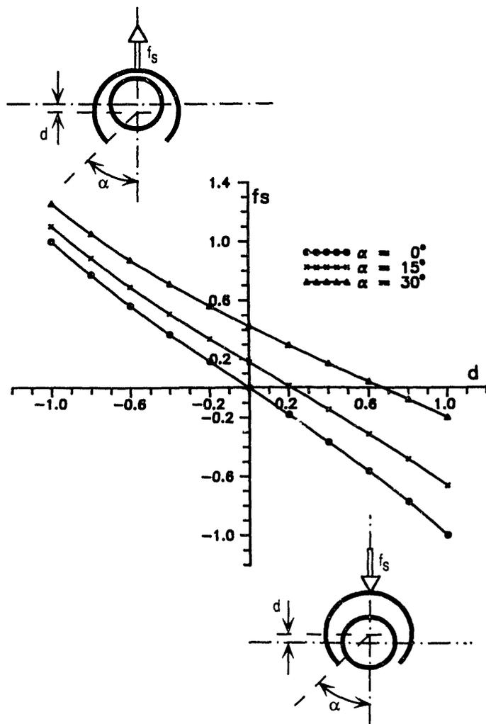
Fig. 5: Transverse force vs displacement between axes with sleeve opening-angle as a parameter.
