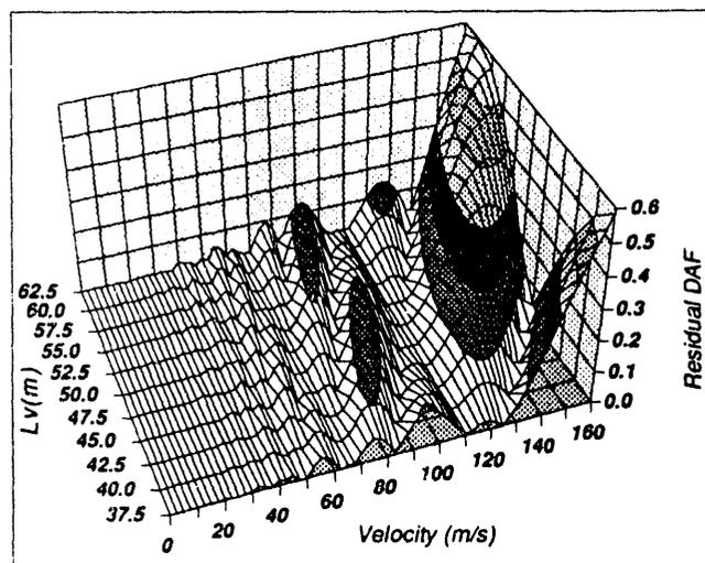
Figure 11. Fully Distributed Vehicle Length (RDAF)
