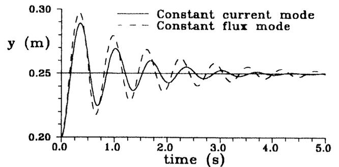
Fig. 8 - Step response with copper damping coils  $d = 0.10$  m.
