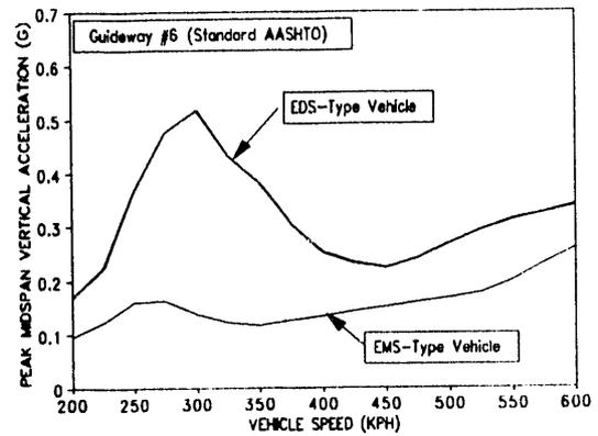
Figure 17. AASHTO Concrete Girder, 21 m Span, Mid span Vertical Beam Accelerations
