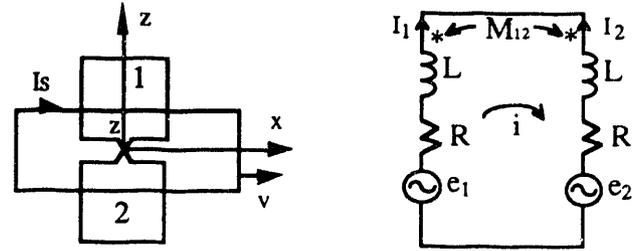
Fig. 1 Equivalent Circuit of a Single SCM Interacting with a Null-Flux Coil
