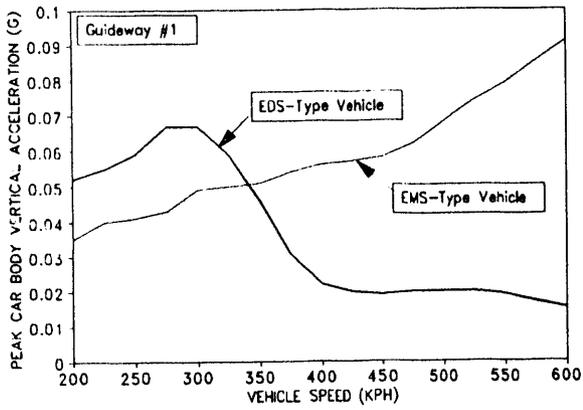
Figure 4. Steel Girder with Concrete Deck, 21 m Span, Carbody Vertical Accelerations
