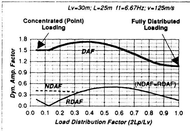
Figure 5. Dynamic Amp. Factor: Point vs. Dist. Loadings
