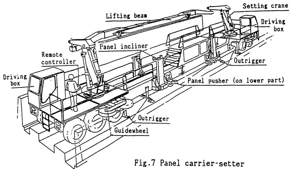
Fig.7 Panel carrier-setter
