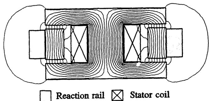
Fig. 7. Flux plot of reluctance motor in cross-section
