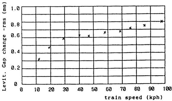
Fig.6 Levitation gap fluctuation vs. train speed
