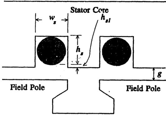
Figure 3. Definition of Dimensions for Calculation of Specific Permeances
