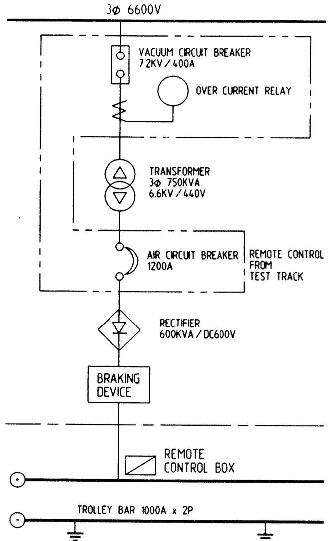
Fig. 11. Power System Schematic
