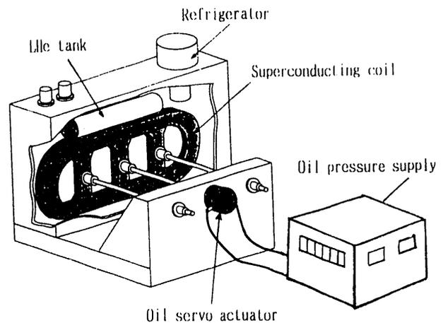
Fig. 8 Mechanical coil vibrating test facility
