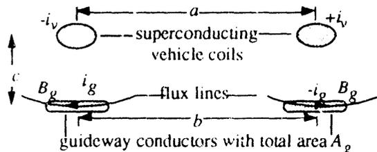
FIG. 1. TWO DIMENSIONAL MODEL OF EDS.
