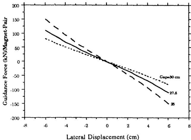
Figure 2. Guidance Force vs Lateral Displacement with Air Gap as Parameter.
