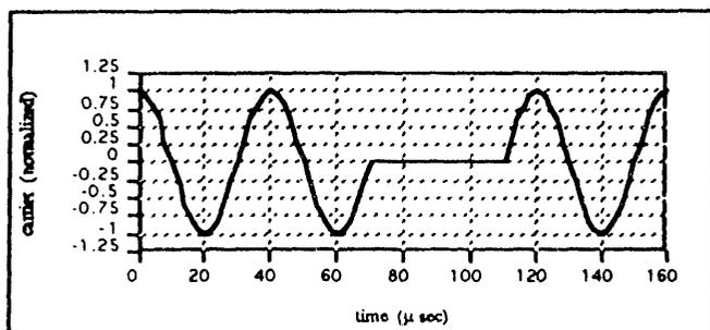
Fig. 8 25 kHz carrier with blank cycle
