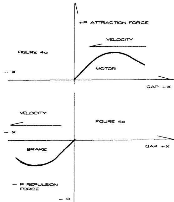
Fig. 4a/4b MPW linear motor +P vs +X characteristic is shown in fig. 4a, while MPW regenerative braking -P vs -X is in fig. 4b, Kozoriz [1-5].
