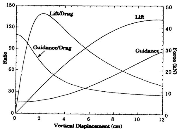
Fig. 8 Total Lift, Total Guidance, Lift/Drag, and Guidance/Drag as a Function of Vertical Displacement. (See Table 1 and Fig. 6 for Other Parameters)
