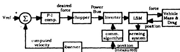
Fig. 2 Block diagram of velocity control loop
