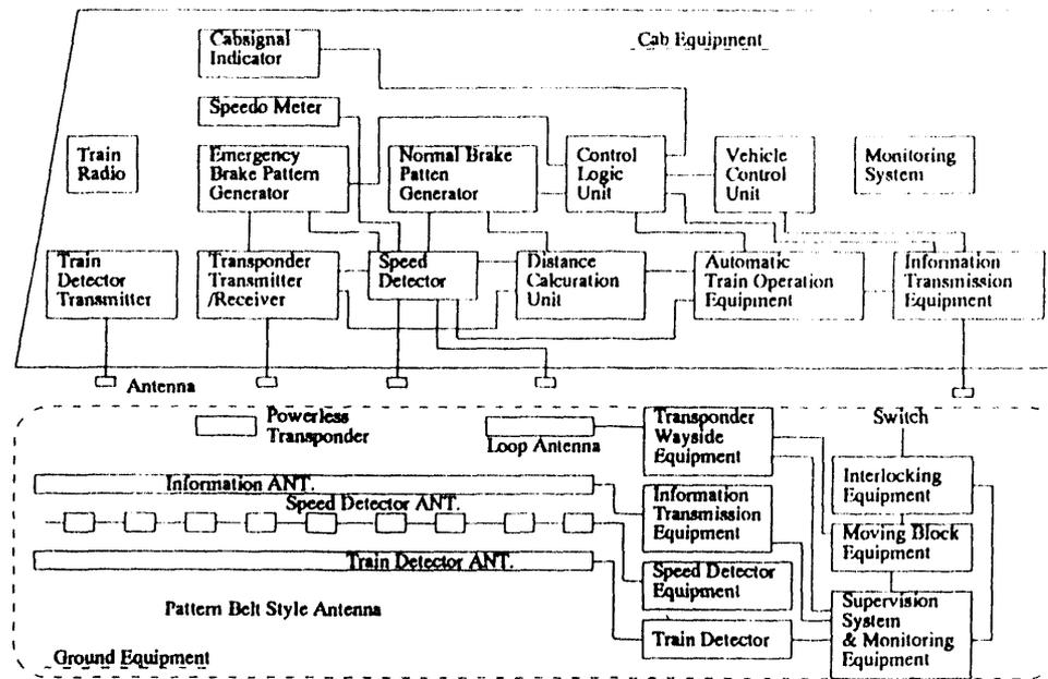
Fig. 1 Configuration of the system
