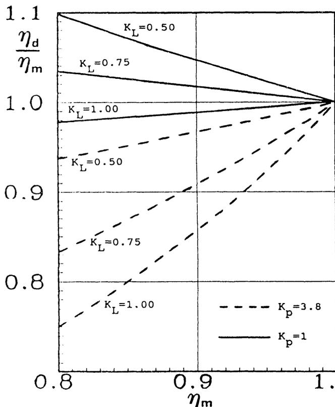
Fig.4. Ratio between the armature efficiencies of the EDS and EMS systems ( $\eta_d/\eta_m$ ) as a function of the armature efficiency that can be attributed to the system EMS; parameters: ratio between the polar pitches ( $K_p=\tau_d/\tau_m$ ) and ratio between the lengths of the fed segments of the track ( $K_L=L_{ad}/L_{am}$ ).
