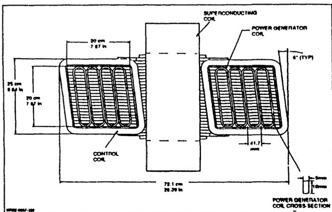
Figure 3: Skewed Magnet Poles with Power Generator Coils
