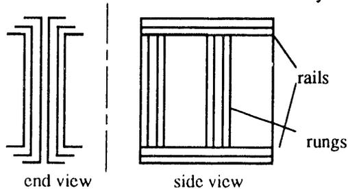
FIG. 10. SIMPLIFIED DETAIL OF SUSPENSION LADDER.
