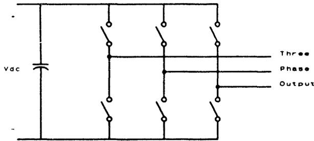
Fig. 2 A three-phase Voltage Source Inverter.
