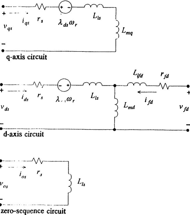
Figure 2. Equivalent Circuit of the LLSM With the Reference Frame Fixed in the Rotor
