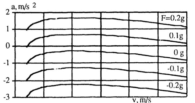
Fig. 3. Acceleration vs. speed for different motor thrusts.
