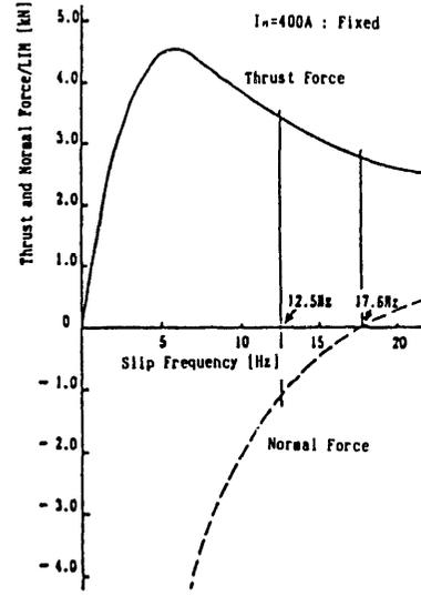
Fig.2 Thrust and Normal Force of LIM
