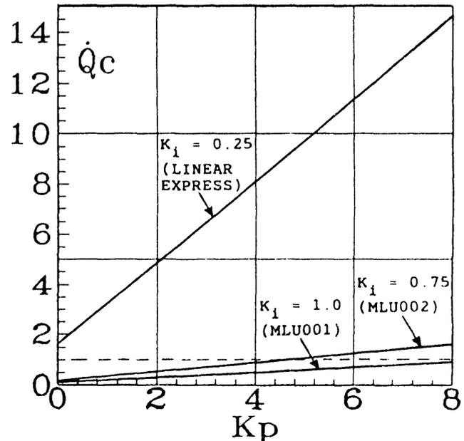
Fig.1. Ratio of the quantity of the armature conductive material of EDS systems referred to that of the EMS system ( $Q_c = Q_{cd} / Q_{cm}$ ), as a function of the ratio between the corresponding polar pitches ( $K_p = \tau_d / \tau_m$ ); parameter:  $K_i = L_{id} / L_{im}$ , ratio between the inductor lengths.
