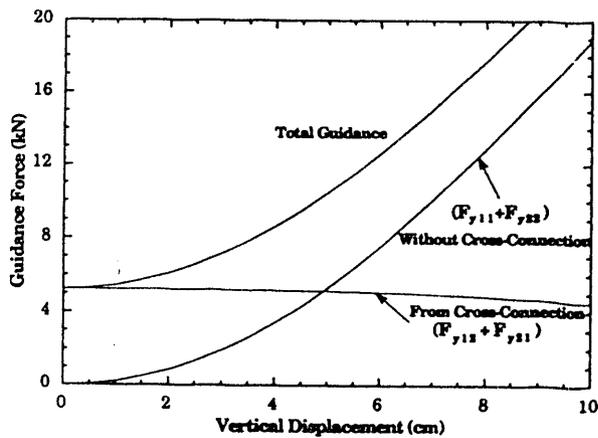
Fig. 7 Guidance Force Components vs Vertical Displacement. (See Table 1 and Fig. 6 for Other Parameters)
