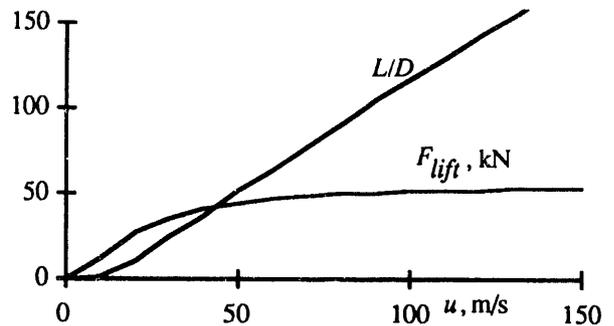
FIG. 12. L/D AND LIFT FOR 8-COIL MODULE.
