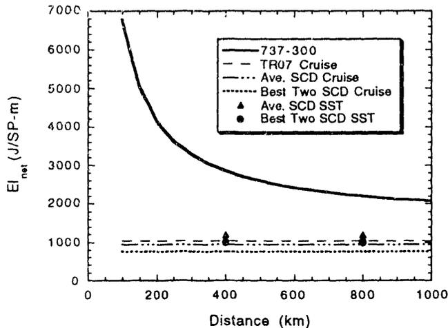
Fig. 2. Net energy intensities including energy supply efficiencies (90% jet fuel, 45% electricity)
