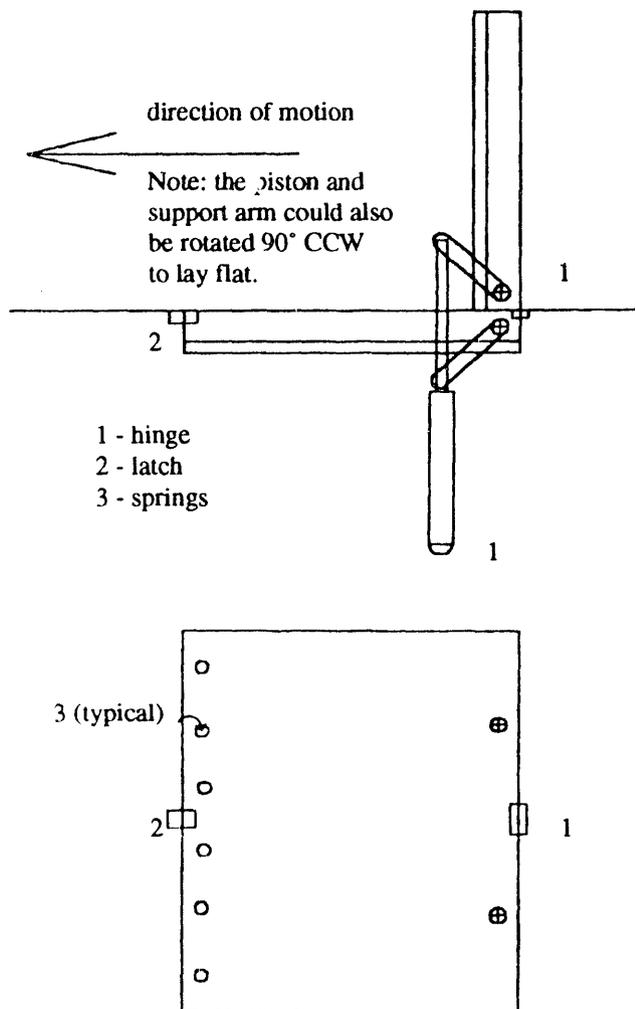
Fig. 2. Surface plates opening aft.
