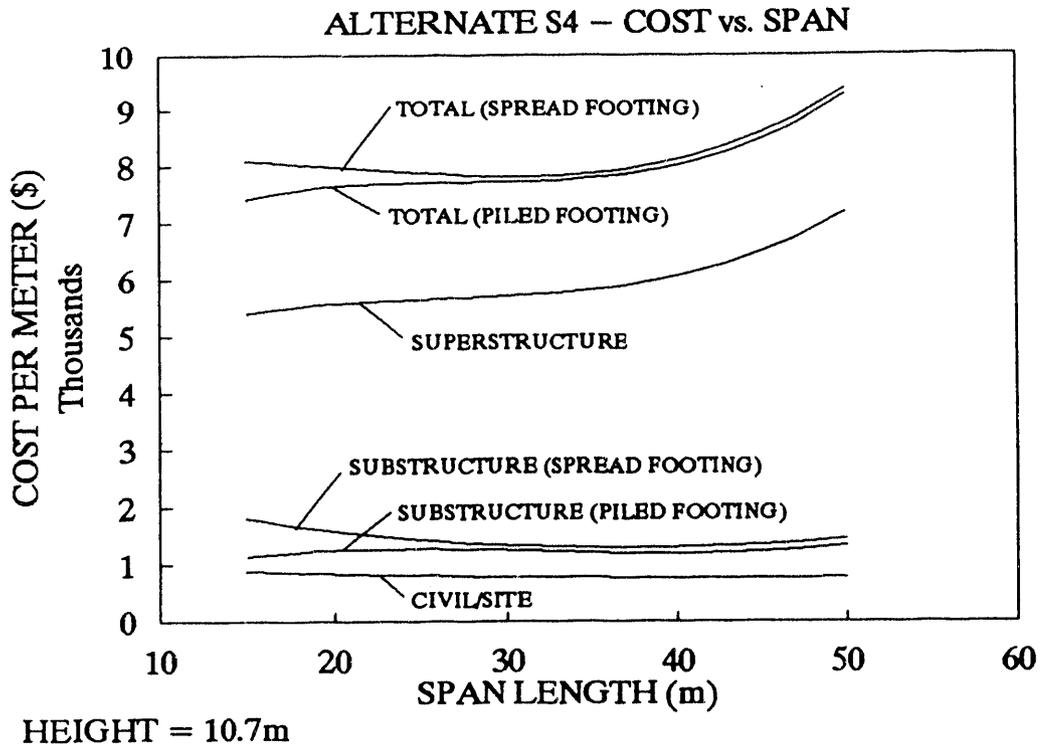
**Figure 3. Spine box girder component and total costs as a function of span length**
