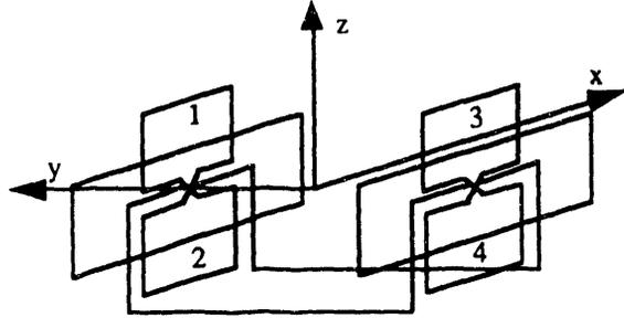
Fig. 2 Cross-Connected Figure-Eight Null-Flux Coils for Maglev Levitation and Guidance
