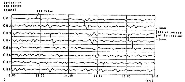
Fig.2 The levitation gap waveform at 100km/h running
