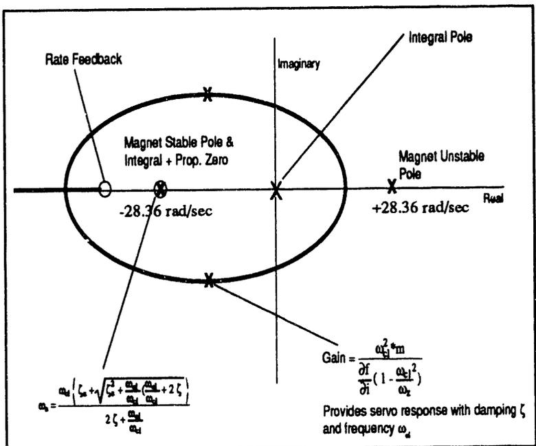
Fig. 2. Root Locus for Servo Design
