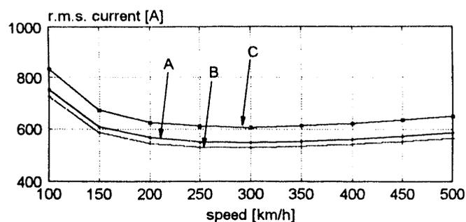
Fig.8 - Current r.m.s. value versus speed for the three proposed strategies.
