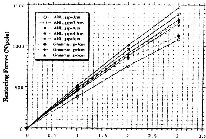
Figure 10. Lateral Restoring Force vs Displacement (cm) (ANL).
