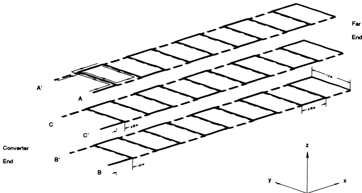
Fig. 1. Exploded View of Magneplane LSM Winding
