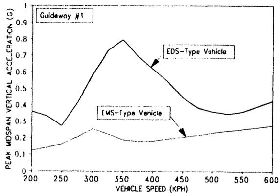
Figure 12. Steel Girder Beams with Concrete Deck, 21 m Span, Mid-Span Vertical Beam Accelerations
