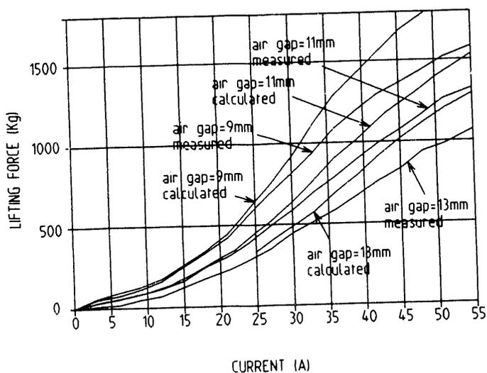
Fig. 13. Magnet Lifting Force
