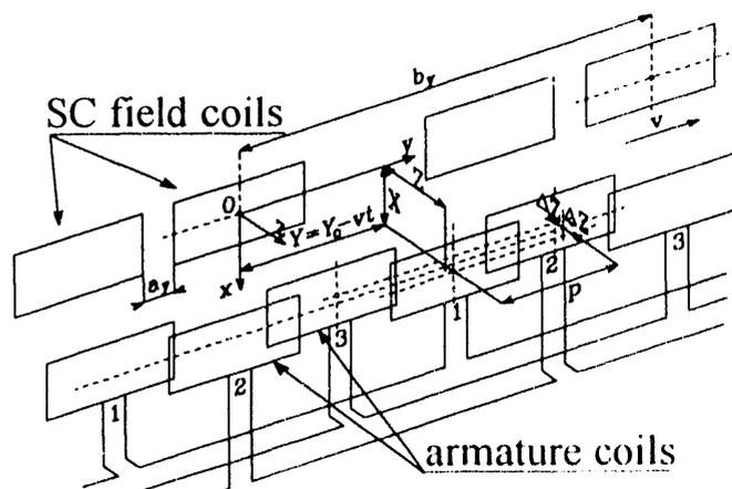
**Fig.2** - Field and armature coils of the LSM. [ $b_y$ : polar pitch;  $a_y$ : distance between the field coils of a pair;  $p$ : pitch of the armature coils; 1,2,3: phases;  $X, Y = Y_0 - \omega t, Z \pm \Delta Z$ : coordinates of a generic armature coil;  $2\Delta Z$ : distance between the armature layers;  $\omega$ : train speed]
