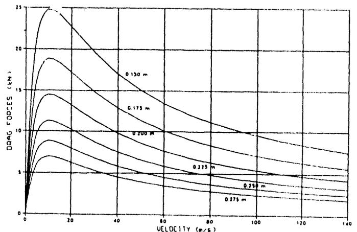
Figure 13. Drag Forces Calculated for Two Sets of Two Magnets on a Single Bogie of the Baseline 45-Passenger Vehicle. (ANL)
