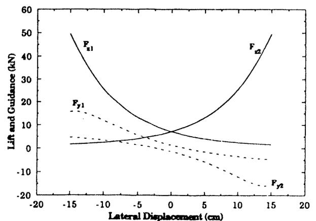
Fig. 11 Lift and Guidance Force Acting on Left- and Right-Hand Side SCMs as a Function of Lateral Displacement. Speed: 138 m/s; Effective Gap: 20 cm; Vertical Offset: 3 cm. (Also see Table 1 for Other Parameters)
