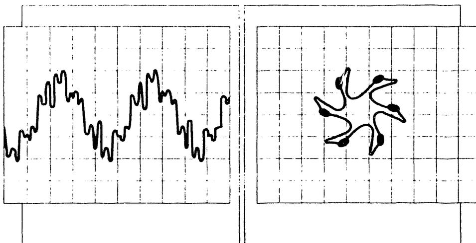
Fig. 3. Inverter current at  $\gamma = 18.7^\circ$ ,  $f_1 = 240 \text{ Hz}$ ,  $f_{Res} = 1680 \text{ Hz}$ ,  $U_d = 2 \times 200 \text{ V}$ , (20 A/T, 1 ms/T)
