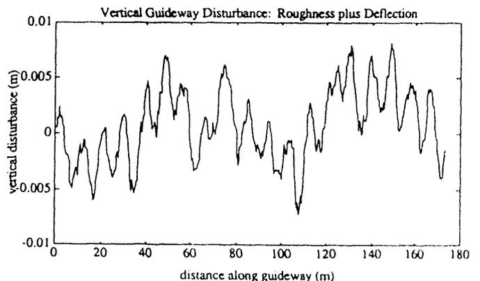
Fig. 2 Combined guideway disturbance.
