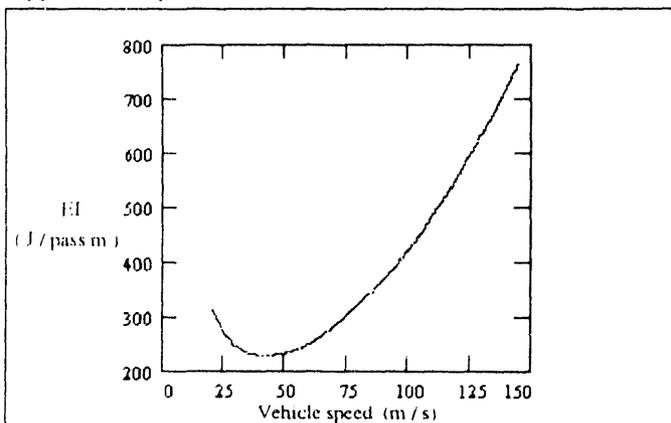
Fig. 3. EI as a function of speed for maglev vehicle.
