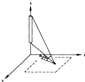
Fig. 2. Geometry of Current Stick and Point in Space Where Magnetic Field is Desired
