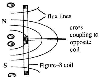
Fig. 14. Guidance coil flux pattern.
