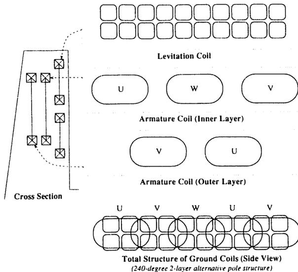
Fig. 3 Ground coil arrangement
