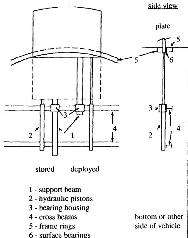
Fig. 3. Plug-type plates.
