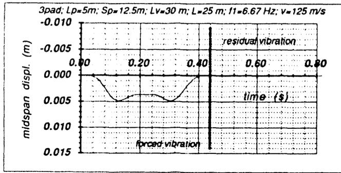
Figure 8. Beam Response for  $Sp = 12.5$  m ( $v = 125$  m/s)
