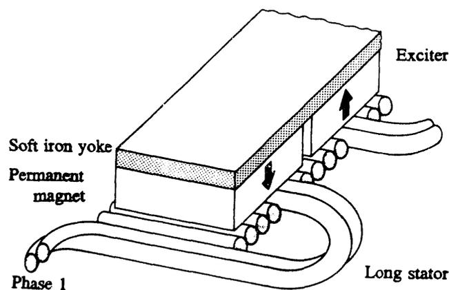
Fig. 9. Permanent excited long-stator motor
