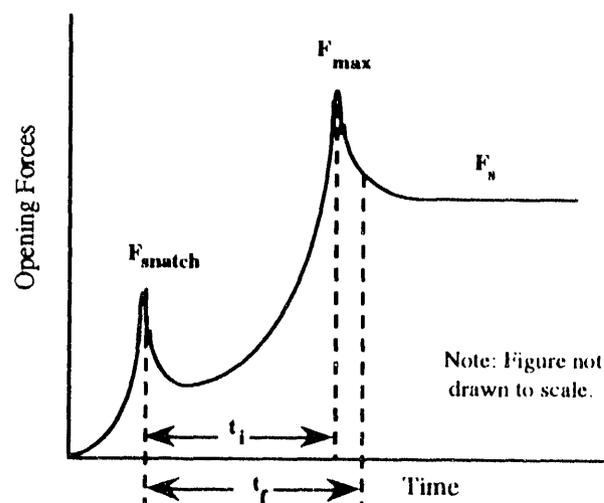
Fig. 4. Opening forces during deployment of parachute for infinite mass assumption.
