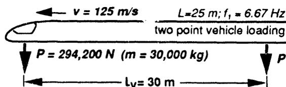
Figure 1. Two Point Vehicle Loading
