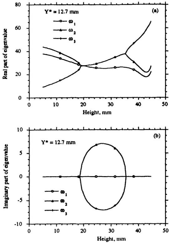
Figure 13. Maglev-system eigenvalues vs. vehicle levitation height, with  $Y^* = 12.7$  mm.
