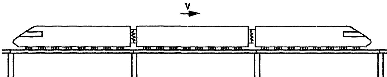
Fig. 1. Model of multicar, multiloading maglev vehicle traveling along a guideway.
