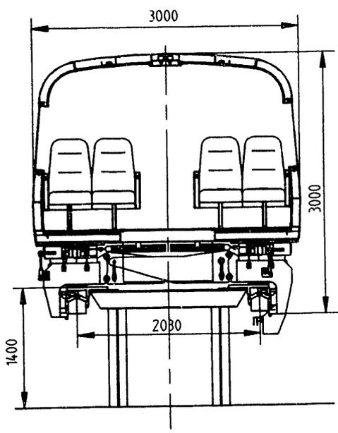
Fig. 3. Sectional View of the System
