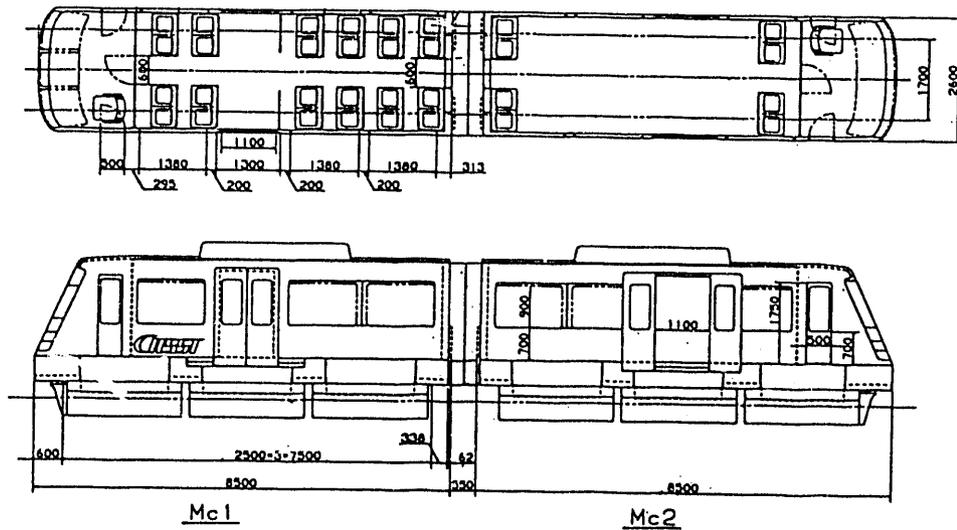
Fig.2 HSST-100 vehicle used for test
