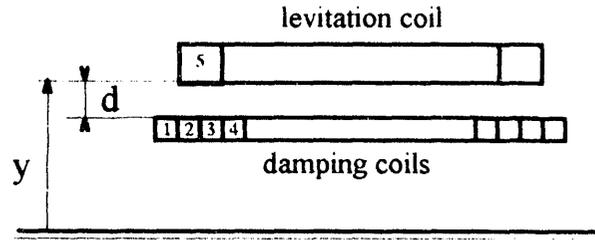
Fig. 2 - Cross-section of the levitation system with damping coils.
