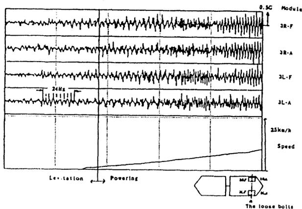
Fig.7 The vertical acceleration of each module on the rail with loose bolts
