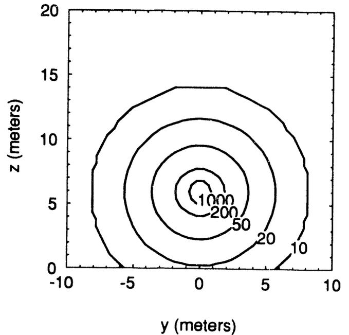
Fig. 4. Magnetic Field From a Distribution Line in mG
