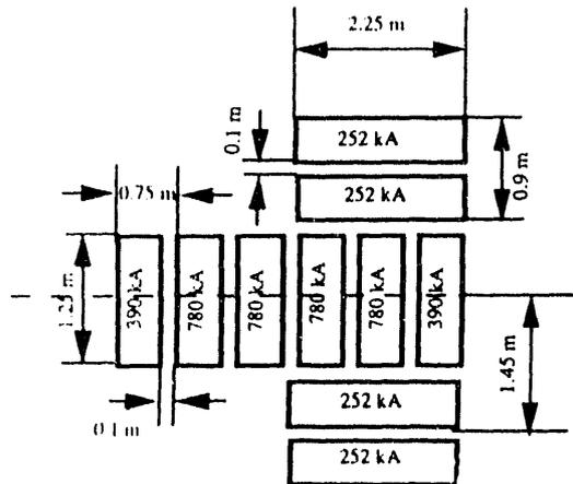
Figure 11. Dimensions, Configuration, and Currents of Magnets used at one end of Magneplane 140-Passenger Vehicle. A Mirror Image of these Magnets is Used at the Opposite End of the Vehicle. (Magneplane)
