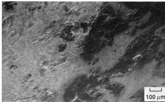
Figure 4.—The carbon layer has been abraded off of the upper left part of this arc-textured Nb-1%Zr radiator surface on exposure to 97 m/s dust-laden wind.
