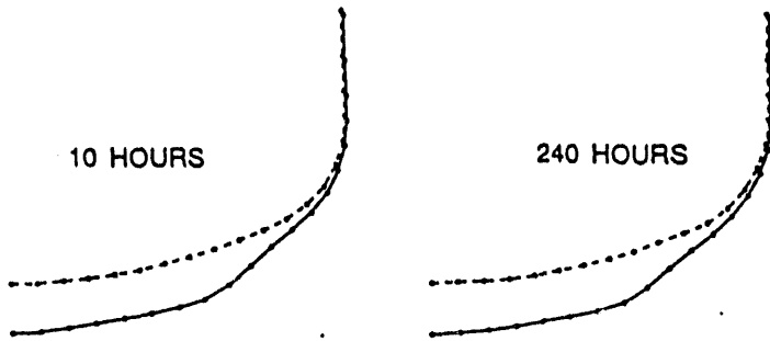
MESH PLOT FOR 75 PSI INTERNAL PRESSURE DISPLACEMENT MAGNIFICATION = 10
