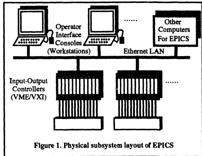
Figure 1. Physical subsystem layout of EPICS
