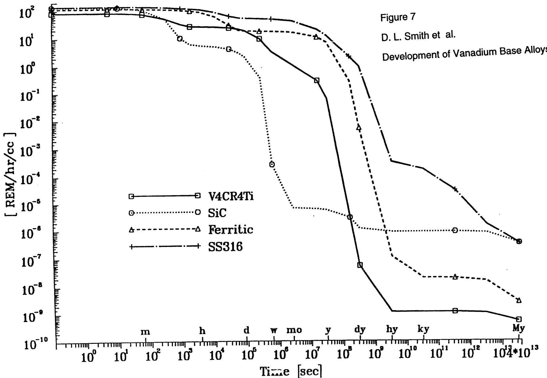
Structural Materials @ Na - ITER [ 1 MW/m<sup>2</sup> - 3 MWa/m<sup>2</sup> ]
