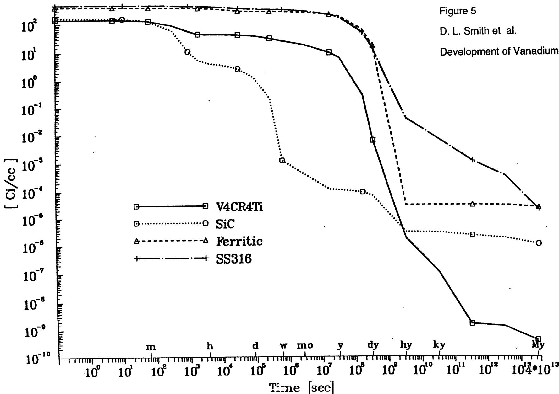
First Wall at 5 MW/m<sup>2</sup> Wall loading [5 y]
