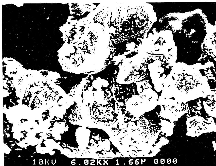
Figure 7.6: SEM picture of untreated CaS grains.
