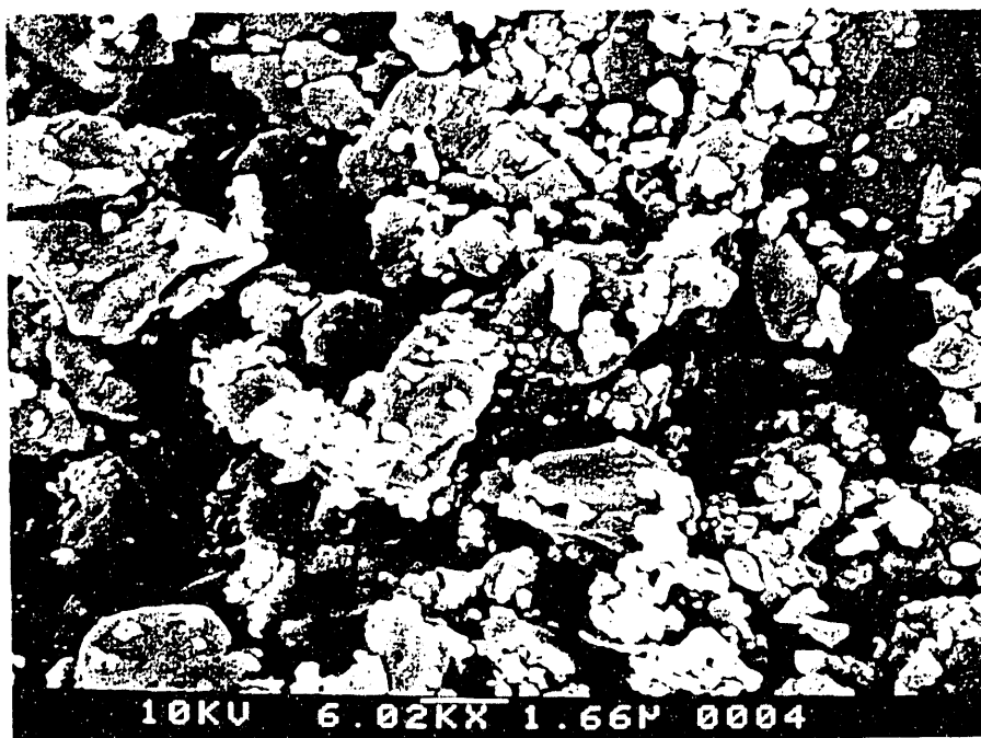
Figure 7.7: SEM picture of CaS grains heated under a N 2 atmosphere.
