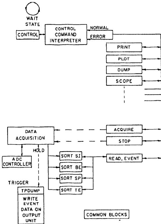
Figure 2: Acquire subroutine and data flow structure.
