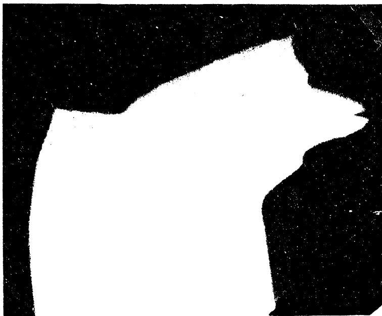
B. Section through burst vessel showing failure path (along top of piece) through weld interface (left) and weld heat-affected zone (right) (10X, EE46716-A)
