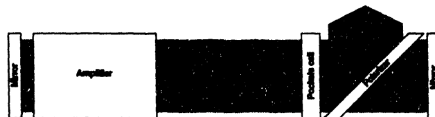
Figure 1. An optical switch enables a multipass laser amplifier architecture. The switch deflects the optical pulse out of the cavity after multiple gain passes.
