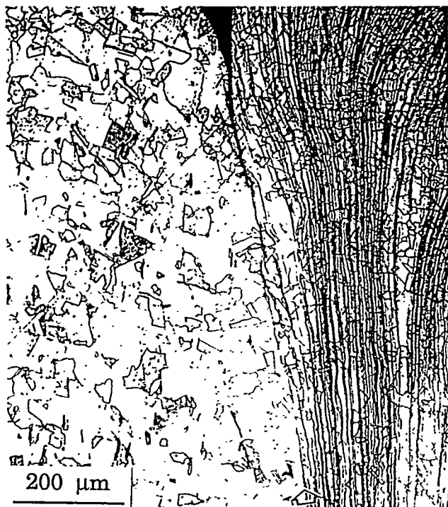
Sample CER-2 Welded at Less Than Intermediate Parameter Settings. Cross Section and Bond Line at Top.
