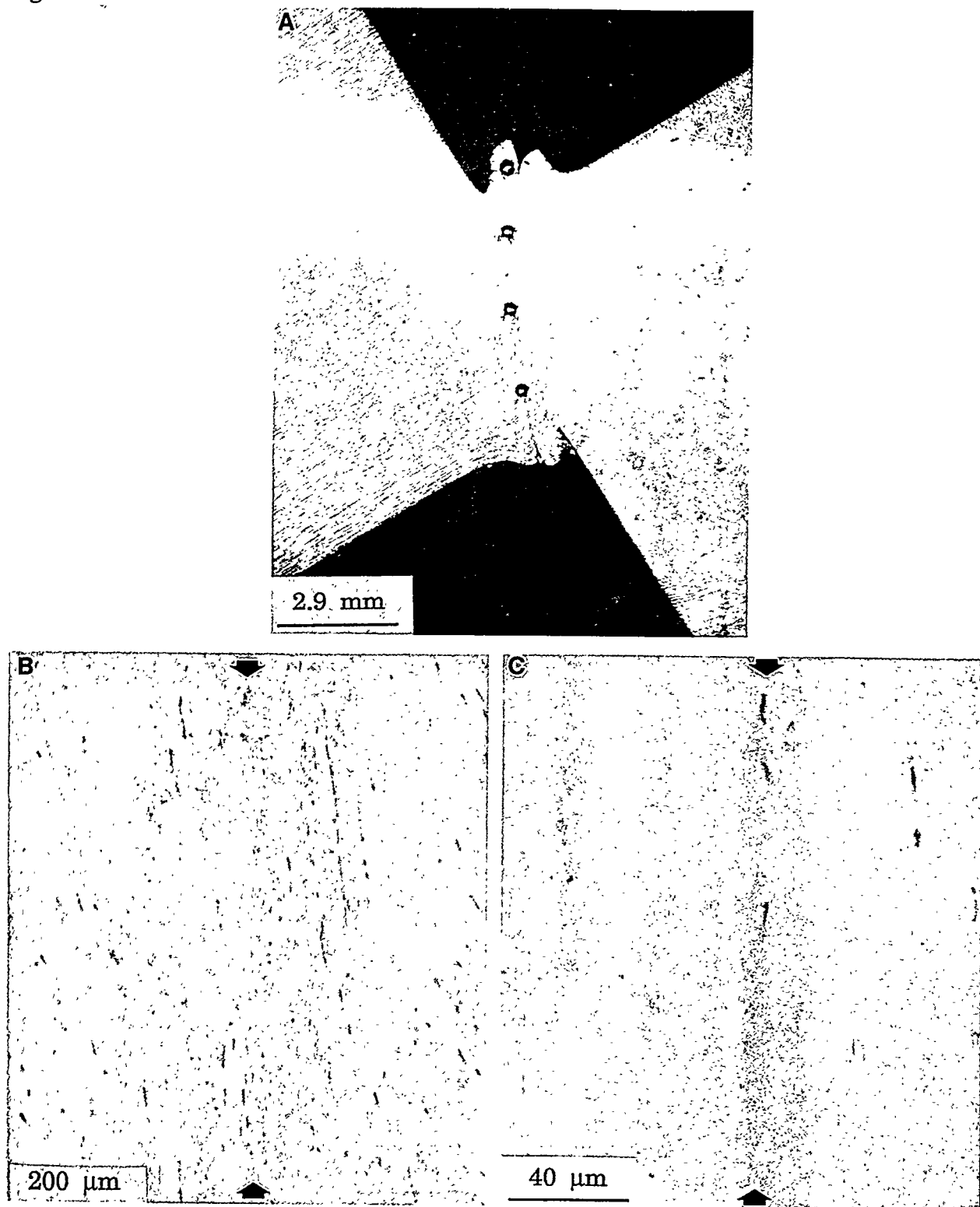
Figure 4: Sample KS06 Welded at Lowest Range of Parameters. Weld Cross Section (A) and Bond Line at Center (B,C). Note Relatively Good Bonding Indicated by Lack of Continuous Bond Line (Arrows). Indentations Present from Hardness Tests (A). Plug Material on Left in (A) and on Right in (B,C). Edges of Plug and Nozzle in (A) Indicate Interference Fit Prior to Welding.
