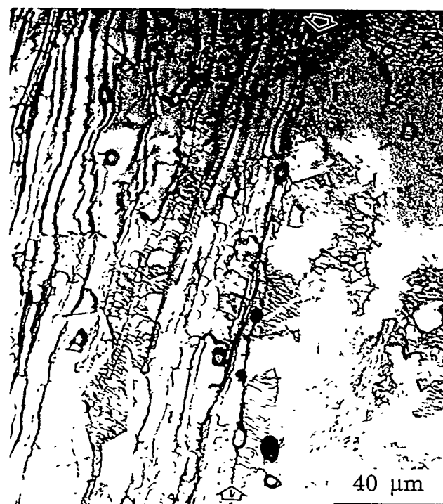
Sample KS19 Welded at Intermediate Recommended Parameter Settings. Cross Section and Bond Line at Top.
