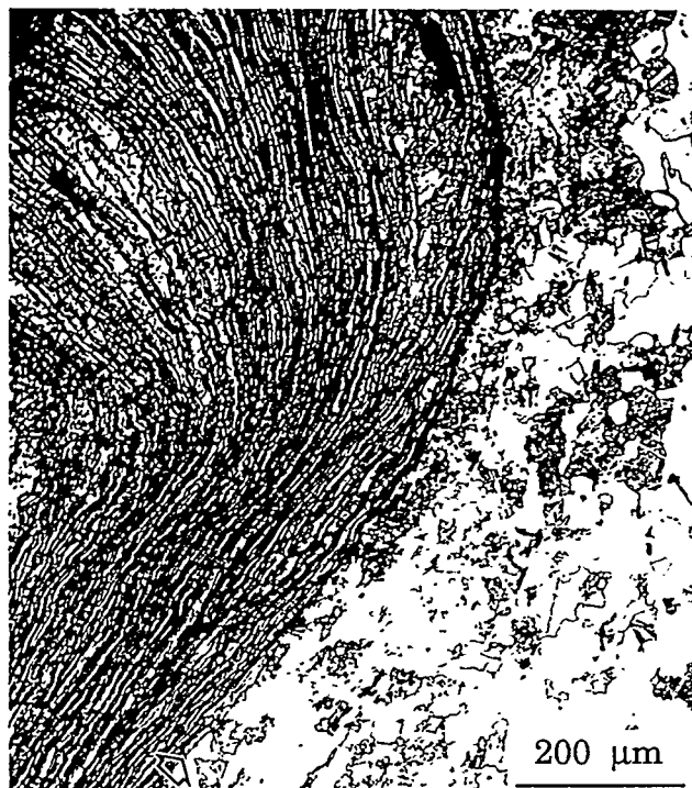
Sample KS19 Welded at Intermediate Recommended Parameter Settings. Cross Section and Bond Line at Top.
