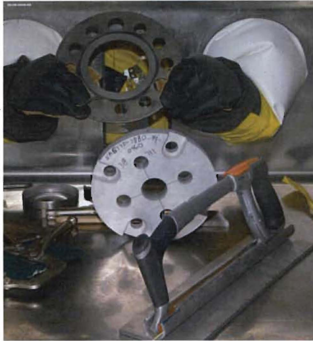
Figure 2. Plates from the APR (smaller and darker, approx 2.7 kg net. wt.) and the first plate from the SPR-II (larger and lighter in color, approx. 16 kg net wt.).
