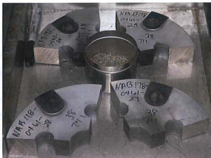
Figure 6. Size reduced plate and associated fines.
