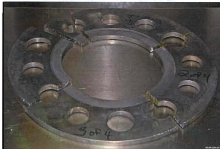
Figure 4 shows the first APR plate size reduced into 4 pieces
