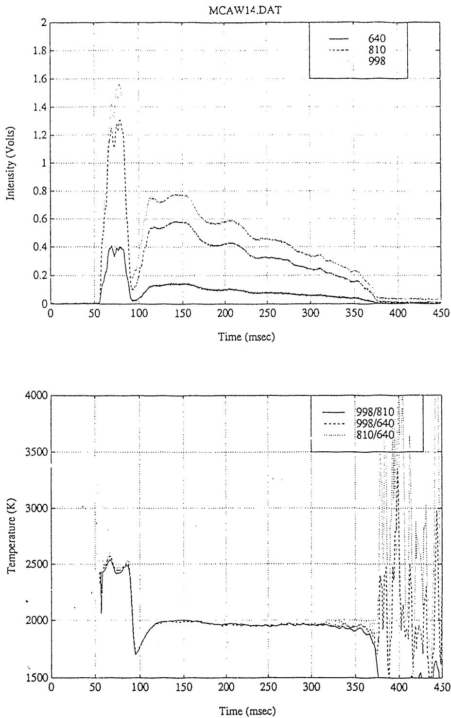
• FIGURE 2. Three-color pyrometry intensity signals (top row) and two-color ratio temperature profiles (bottom row) for a micronized CWF agglomerate, with initial diameter  $\approx 270\mu\text{m}$ , burning in air at  $T_g$  of 1450 K,  $\rho_a = 0.58 \text{ g/cm}^3$ .
