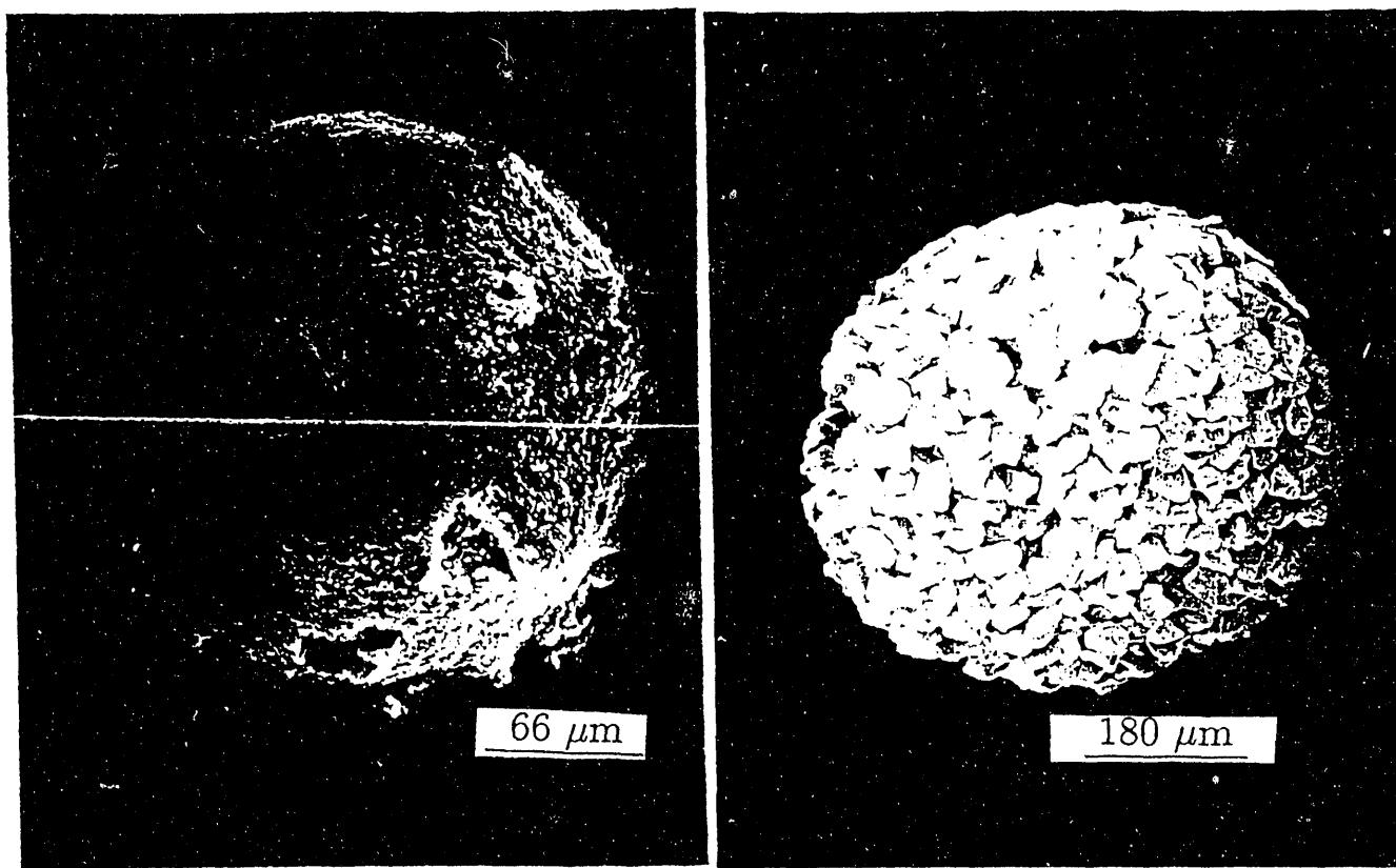
• FIGURE 1. (a) SEM photograph of a dry micronized CWF agglomerate with diameter  $\approx 250\mu\text{m}$ ; coal grain  $\approx 3.5\mu\text{m}$ . (b) SEM photograph of a dry pulverized CWF agglomerate with diameter  $\approx 585\mu\text{m}$ ; coal grain  $\approx 40\mu\text{m}$ .
