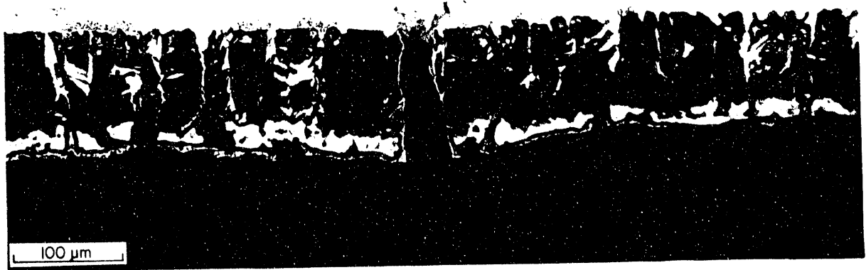
Fig. 2. Chromized coating on modified 316 (HT-UPS) stainless steel after creep testing at 700°C.
