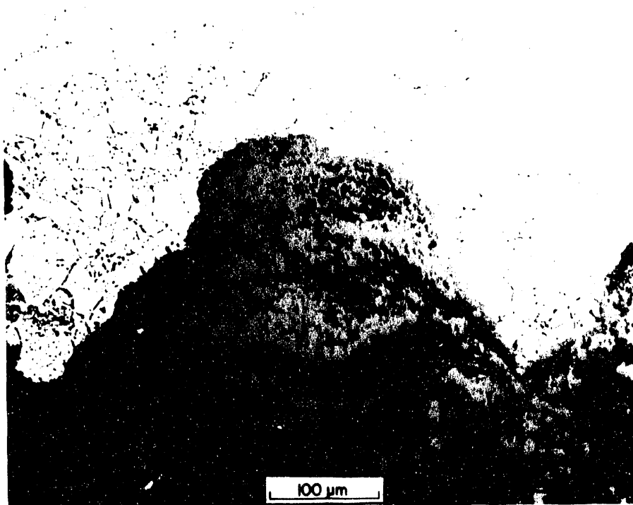
Fig. 11. Oxidation of modified alloy 800 tube after 500 h at 900°C with a cycle to near room temperature each day.
