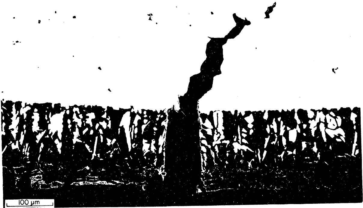
Fig. 1. Chromized coating on 17-14CuMo stainless steel after creep testing at 700°C.
