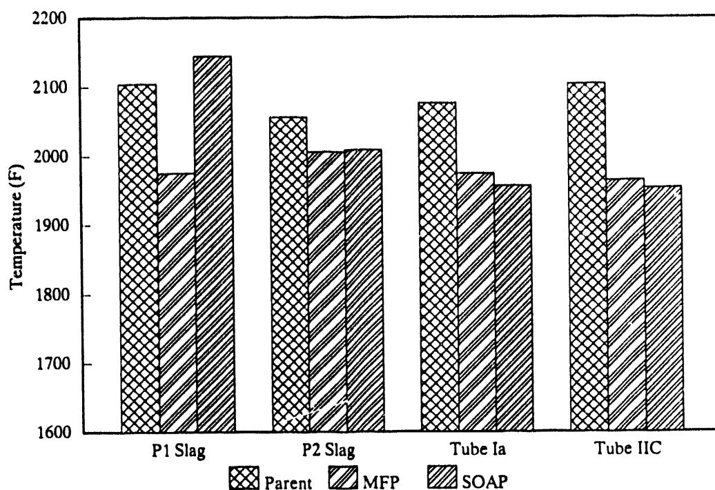
Figure 9. Reducing atmosphere ash fusion softening temperatures for the outer waterwall panel and steam-tube deposits.
