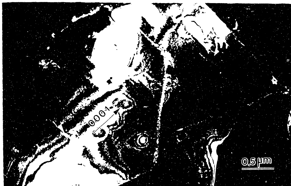
Figure 7. Transmission electron micrograph of Laves phase \text{MgNi}_2 after uniaxial compression. Stacking faults and slip bands are seen on nonbasal planes, indicative of a variety of slip systems in this phase.
