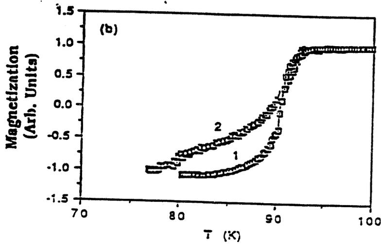
Fig. 1 (a) Resistivity vs temperature curves, and (b) magnetization vs temperature curves are shown for the samples sintered at  $940^\circ\text{C}$  in pure  $\text{O}_2$  marked by 1 and in 0.5%  $\text{CO}_2/\text{O}_2$  marked by 2.
