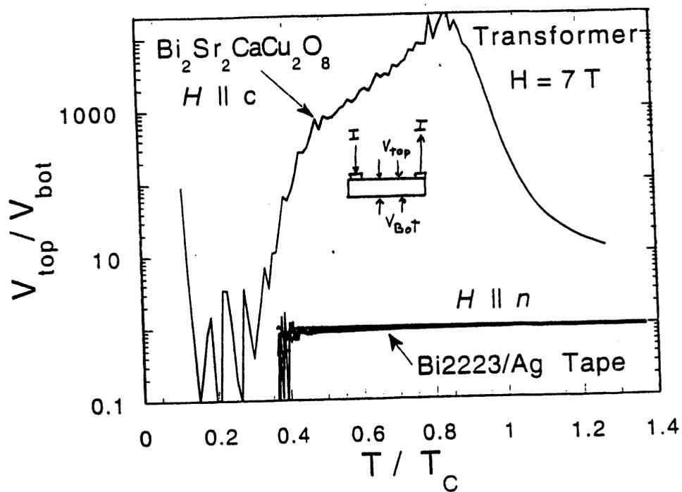
Fig. 4. Comparison of the resistivity anisotropy using the transformer configuration (current contacts on the top surface of the sample, voltage contacts on both the top and the bottom) at  $H = 7 \text{ T}$  and  $H \parallel c$  for a  $10 \mu\text{m}$  thick Bi-2212 single crystal and  $H \parallel n$  for a  $50 \mu\text{m}$  thick Bi-2223/Ag tape.
