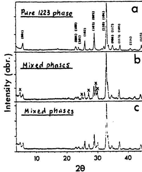
Fig. 3. X-ray powder diffraction patterns of pulverized pellets of (a)  $Tl_{0.78}Bi_{0.22}Sr_{1.6}Ba_{0.4}Ca_2Cu_3O_{9-\delta}$ , (b)  $Tl_{0.5}Pb_{0.5}SrBaCa_2Cu_3O_{9-\delta}$  and (c)  $Tl_{0.78}Bi_{0.22}SrBaCa_2Cu_3O_{9-\delta}$ . All pellets were made by sintering at 880°C for 3.0–4.5 h in air and quenched in air at room temperature.
