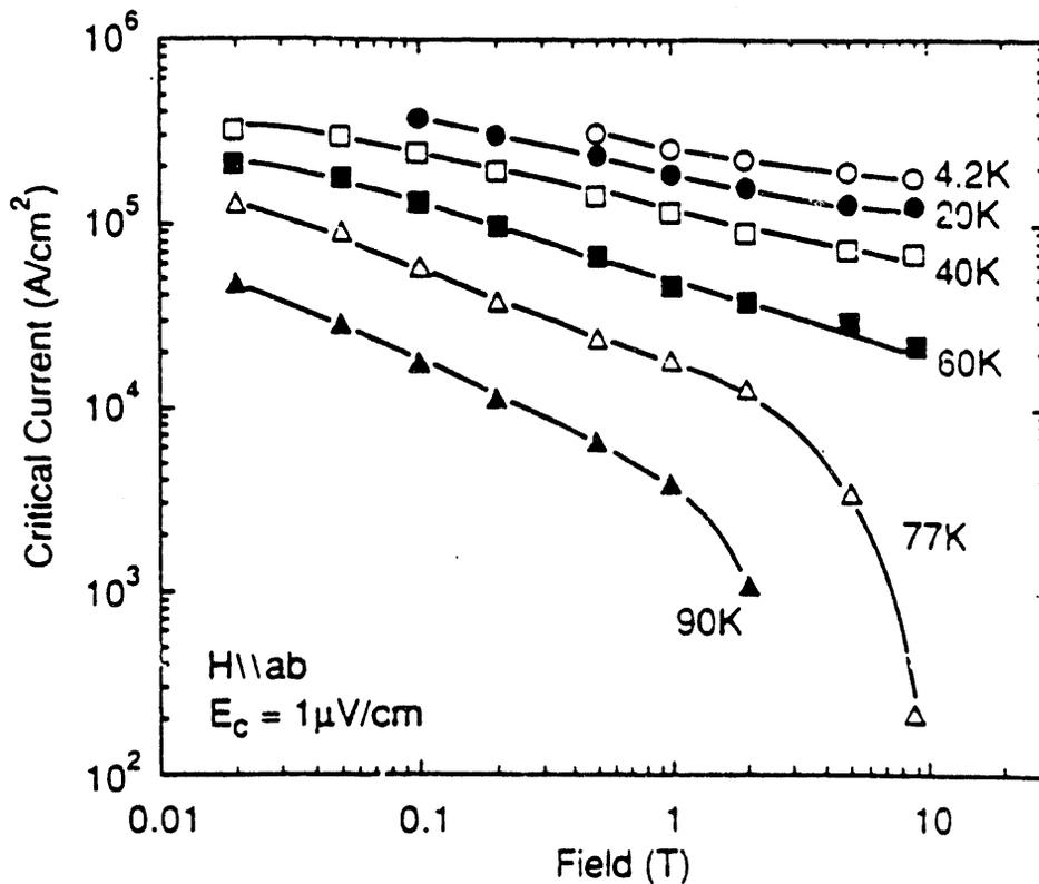
Figure 7. Critical current density versus applied field for  $H \parallel c$  and  $H \parallel ab$  at 77 K for Ti-1223 film applied by spray pyrolysis and reacted using a two-zone method. (Due to DeLuca et al. reference 49)
