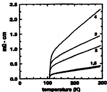
Fig. 3. Resistivity vs. temperature plots for slices from tape A. The high resistivity of slice 4 is believed to be due to a current path that was longer than the measured macroscopic dimension (see ref. [6]), consistent with the presence of cracks in the slice. The zero-temperature intercept of slice 4 is not anomalous; this parameter steadily decreases to  $\sim 0 \mu\Omega \text{ cm}$  as the slice position moves towards the outside.
