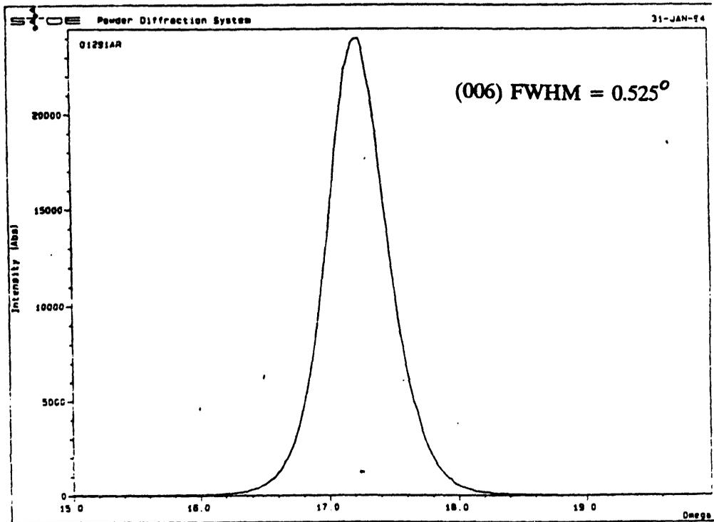
Characteristics of the (Tl, Bi) Sr<sub>1.6</sub> Ba<sub>0.4</sub> Ca<sub>2</sub> Cu<sub>3</sub> O film
