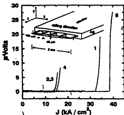
Fig. 1. Voltage-current traces for different microslices of tape A at 77 K and zero applied field are shown. The slices were also measured in a field of 8 mT applied normal to the broad face of the original tape surface; the  $J_c$  values were then unchanged (slice 1), 0.45 (3) and 0.8 (4) of the zero field values, respectively. The geometry of the slices cut from tape A and the coordinate axes of the cuts are shown in the inset.
