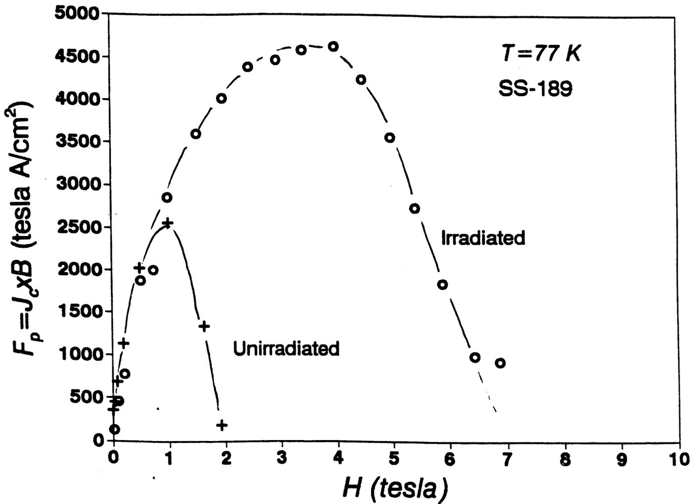
**The Flux Pinning Force Density  $F_p$  of
