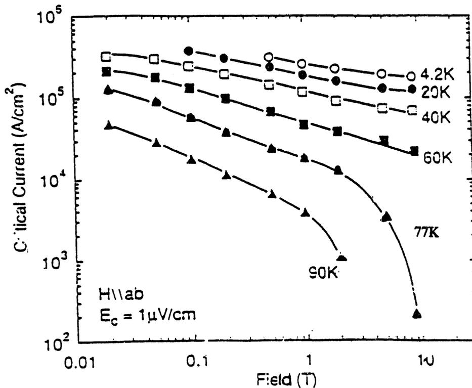
Figure 7. Critical current density versus applied field for  $H \parallel c$  and  $H \parallel ab$  at 77 K for Tl-1223 film applied by spray pyrolysis and reacted using a two-zone method. (Due to DeLuca et al. reference 49)
