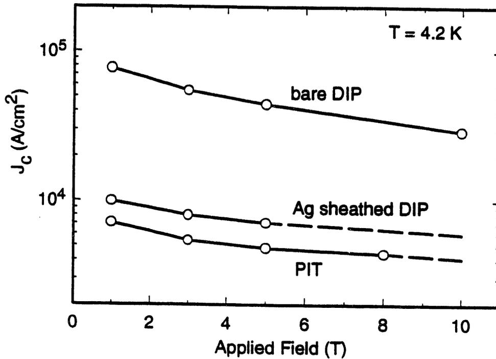
Figure 2.  $J_c(4.2K)$  in the overall silver plus ceramic cross-section
