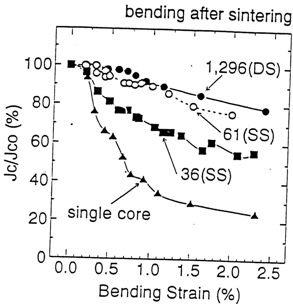
Fig.2 Bending strain characteristics of the high- $T_c$  superconducting tape
