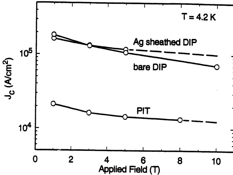
Figure 1.  $J_c(4.2K)$  in the ceramic layer
