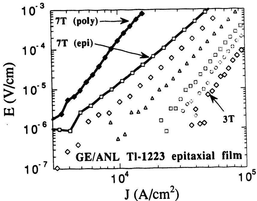
Figure 2. Comparison of I(V) for polycrystalline (a) and epitaxial (b) films of Tl-1223 showing the enhanced dissipation across grain boundaries. An explicit comparison is shown in (b) for a field of 7 T.
