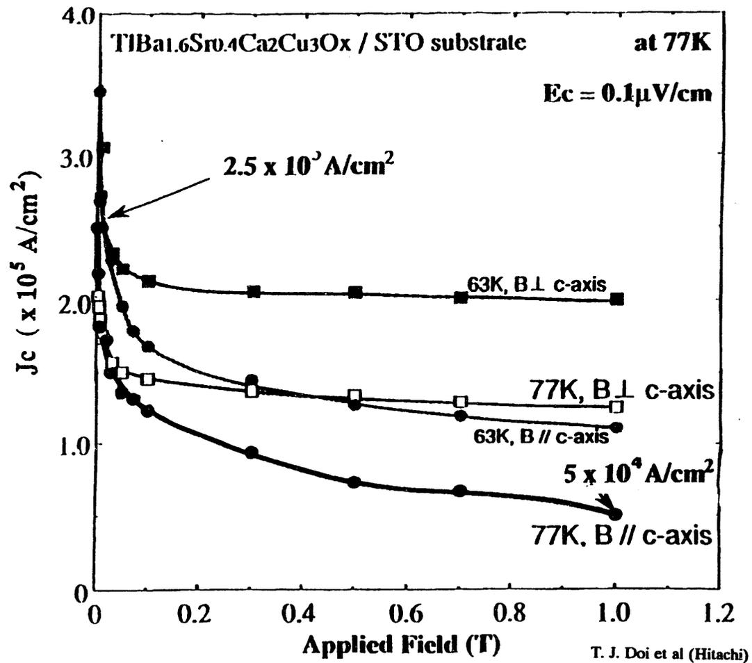
Fig. The magnetic field dependence of TlBa<sub>1.6</sub>Sr<sub>0.4</sub>Ca<sub>2</sub>Cu<sub>3</sub>O<sub>x</sub> on STO
