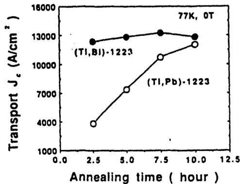
Fig. 4. Comparison of the effects of the annealing time on the transport  $J_c$  (77 K, 0 T) of the in-situ synthesized superconducting tapes of  $Tl_{0.78}Bi_{0.22}Sr_{1.6}Ba_{0.4}Ca_2Cu_3O_{9-\delta}$  and  $Tl_{0.5}Pb_{0.5}Sr_{1.6}Ba_{0.4}Ca_2Cu_3O_{9-\delta}$ .
