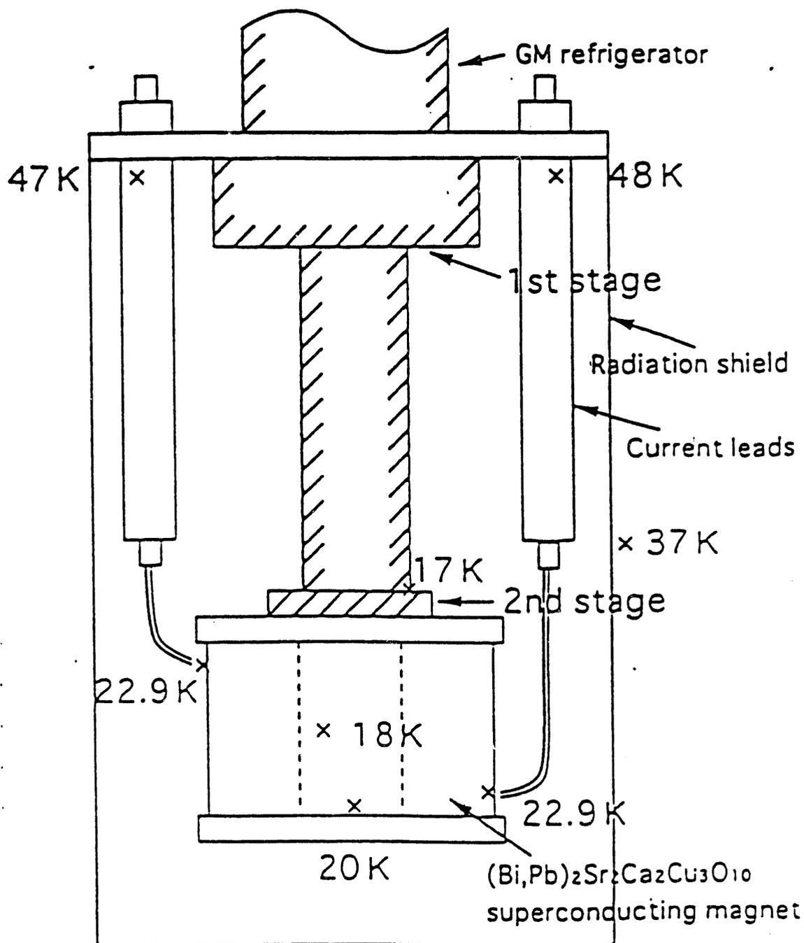
Fig.5 Temperature profile in the conduction-cooled high- $T_c$  magnet system when the coil was operated at 30.8A and held for 100h.
