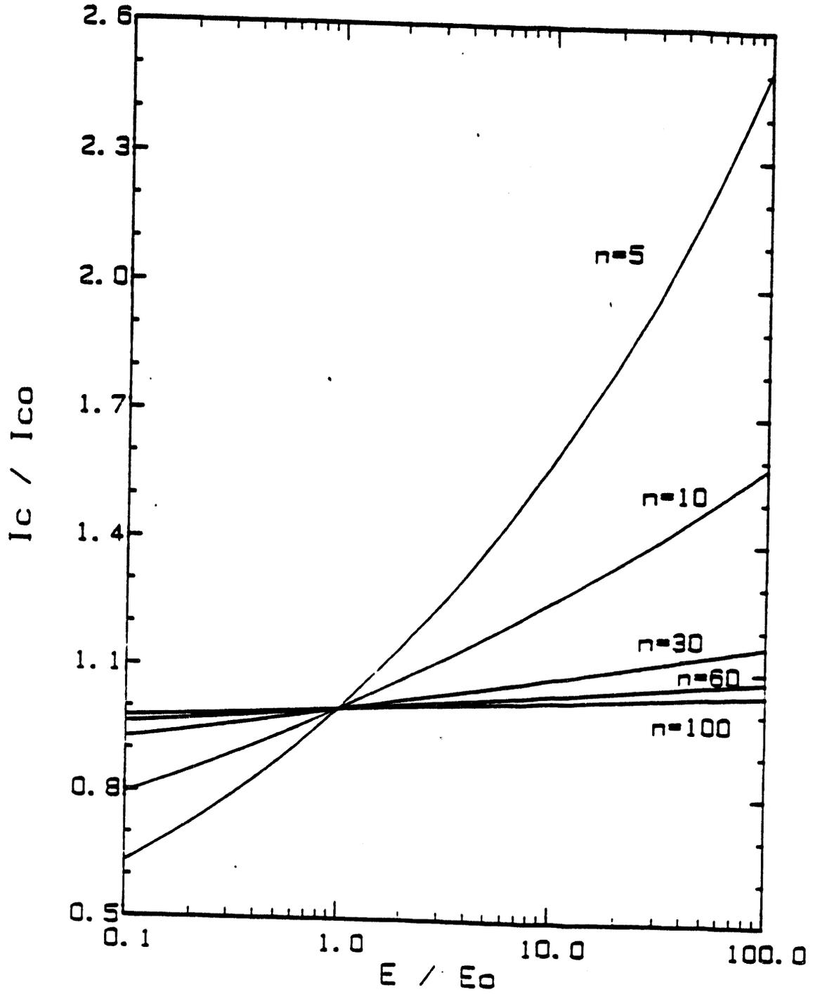
Fig. 4.1. The dependence of  $I_c$  on electric field criterion for various  $n$  values.
