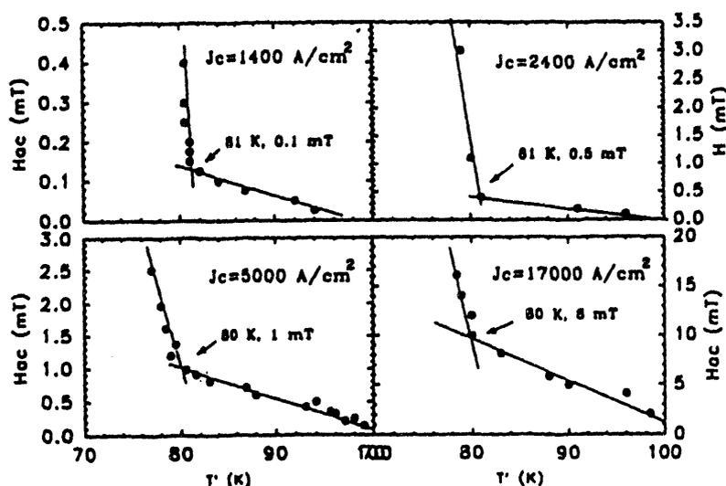
Fig.5 Field dependence of  $T'$  for various tapes with different  $J_c(0T, 77K)$  values
