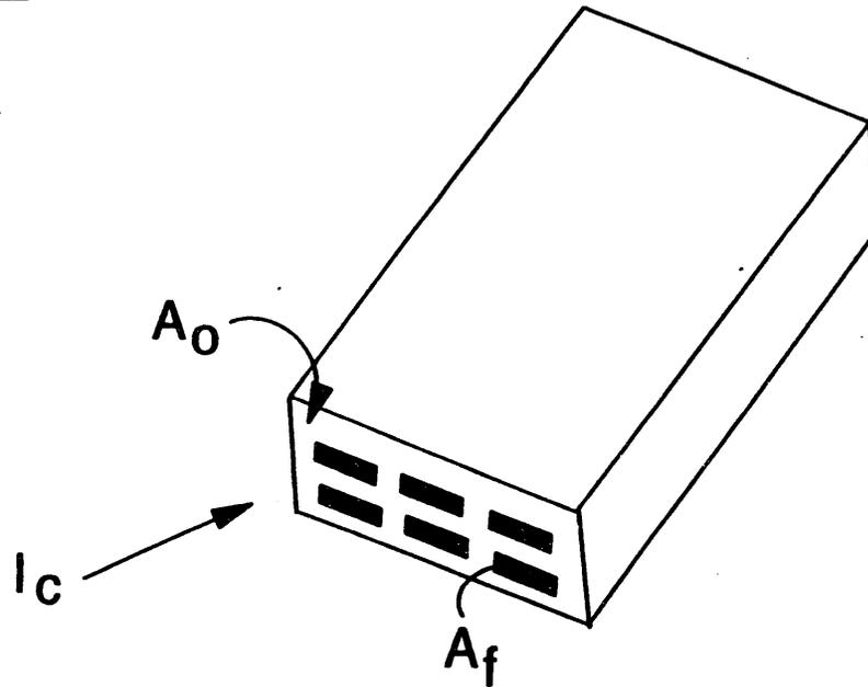
Filament Critical Current Density =  $J_c = I_c / A_f$
