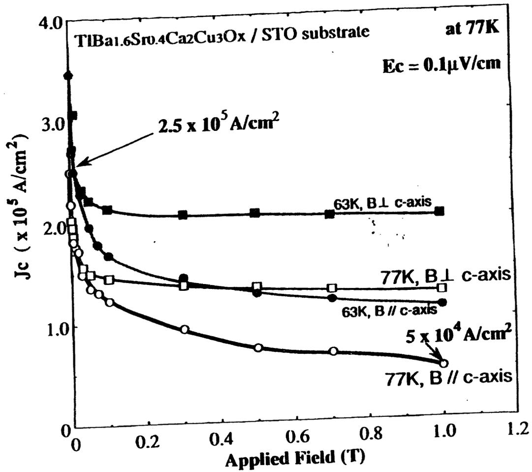
Fig. The magnetic field dependence of TlBa<sub>1.6</sub>Sr<sub>0.4</sub>Ca<sub>2</sub>Cu<sub>3</sub>O<sub>x</sub> on STO.
