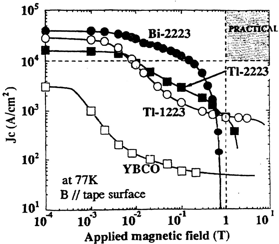
Fig. Transport  $J_c$  of HTS wires
