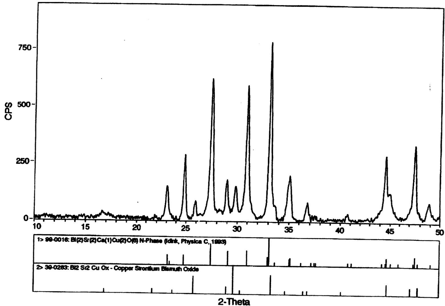
X-Ray diffraction of BSCCO precursor powders produced by SCI.
