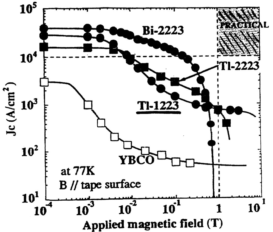
Fig. Transport  $J_c$  of HTS wires
