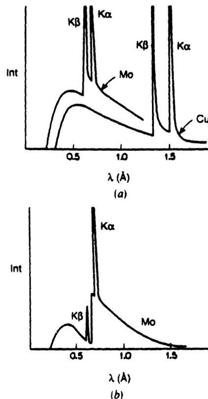
Fig. 1. X-ray spectra. (a) Mo tube (operated at 50 kV) and Cu tube (operated at 35 kV). (b) Mo spectrum if a 0.001 in Nb  $\beta$  filter is used.
