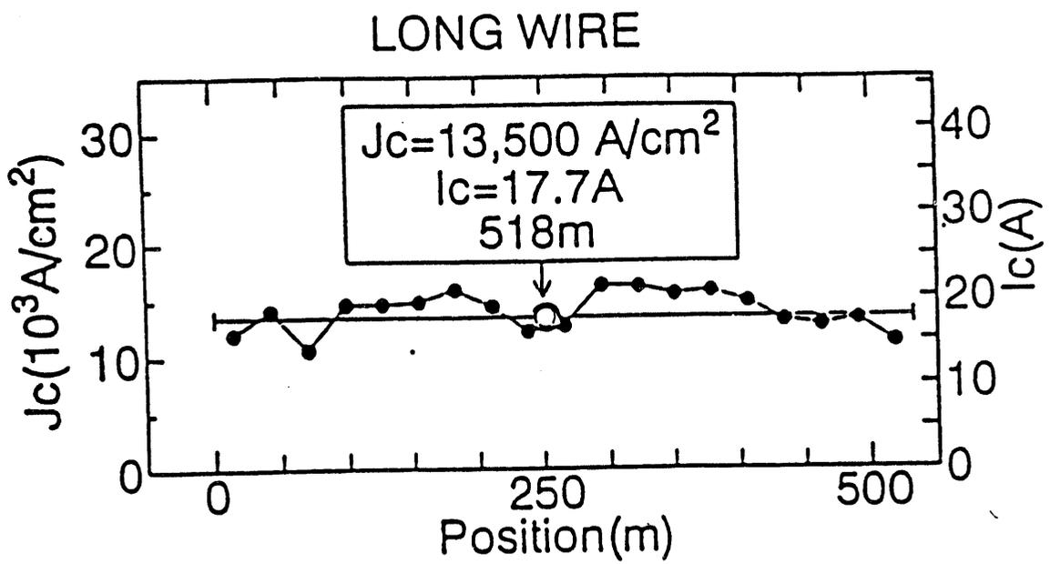
Fig.1  $I_c$  distribution of high-T<sub>c</sub> superconducting tape of 518 M
