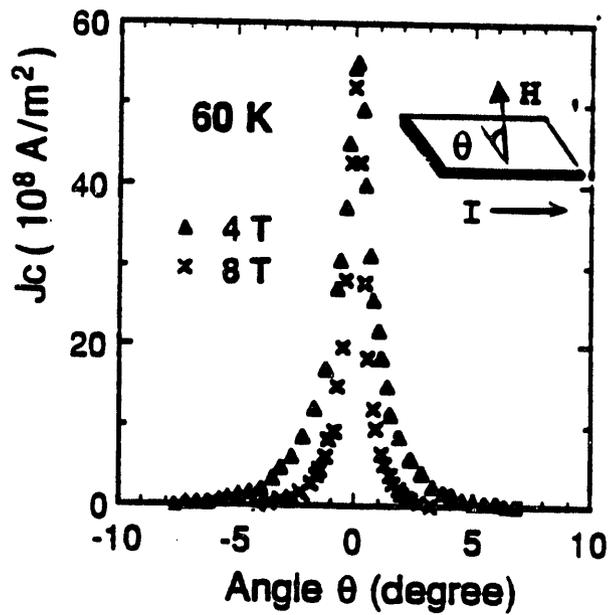
Fig. 3(b)  $J_c(H, \theta)$  measured at 60 K as a function of the angle between applied field and the  $a-b$  plane.
