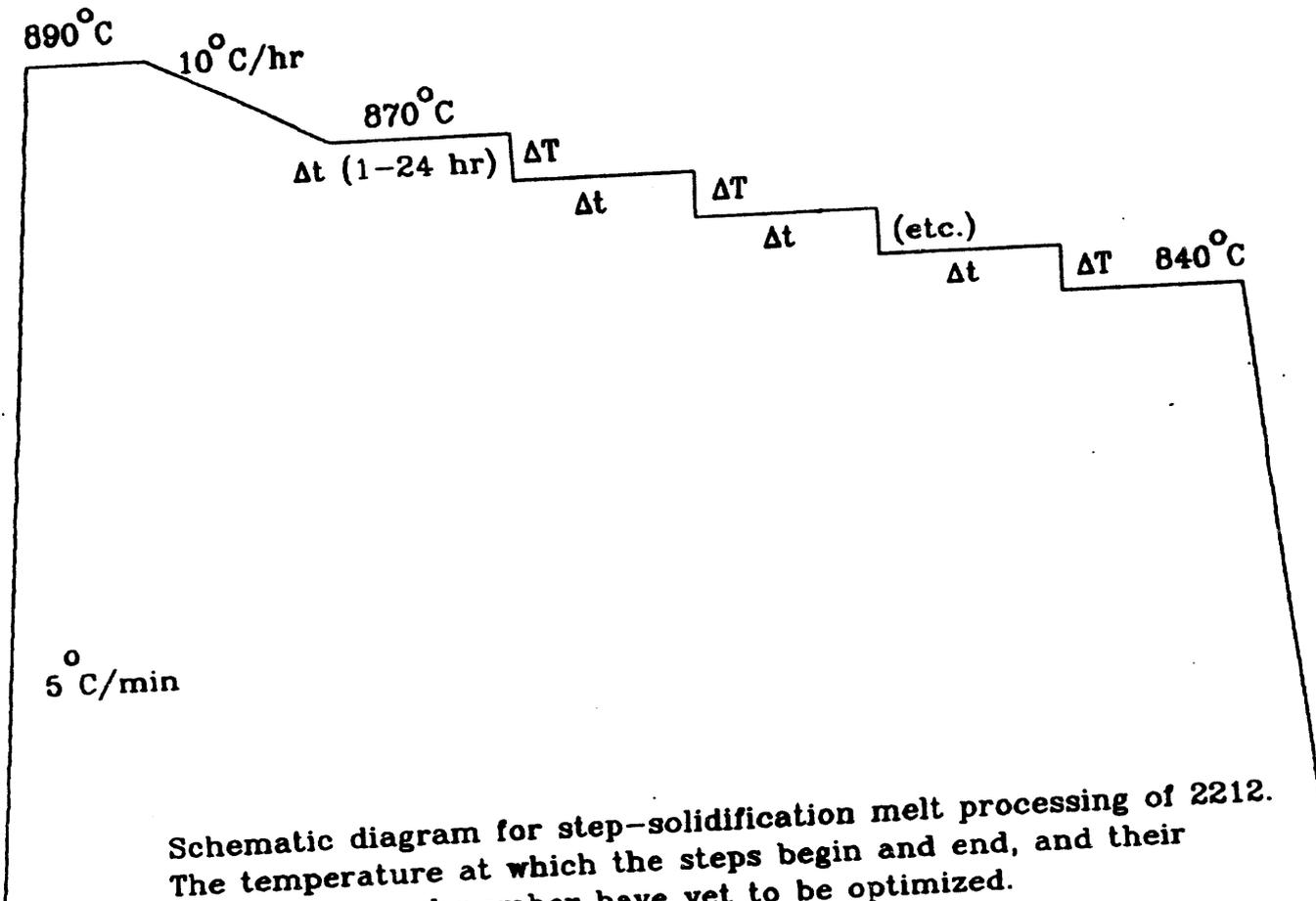
Schematic diagram for step-solidification melt processing of 2212. The temperature at which the steps begin and end, and their length, size, and number have yet to be optimized.
