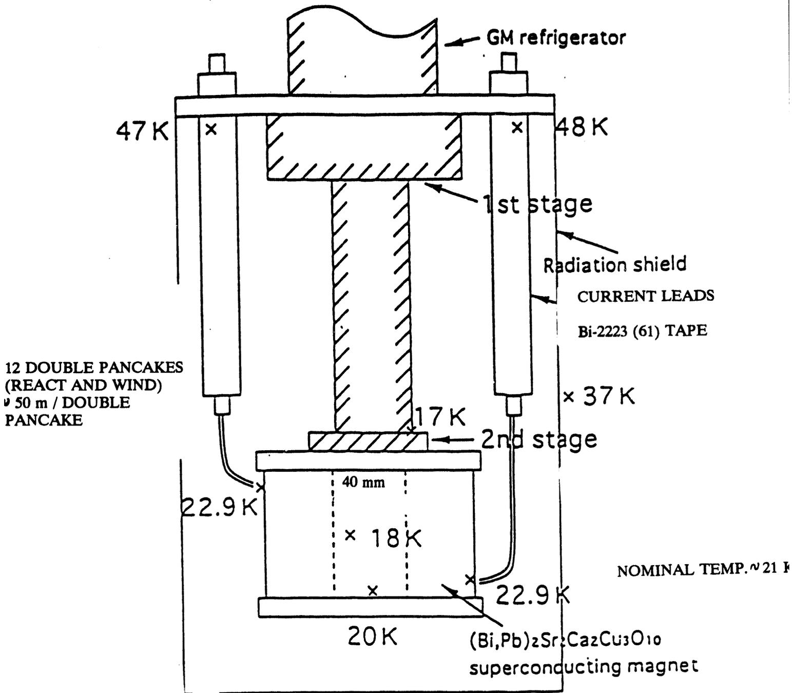
Fig.5 Temperature profile in the conduction-cooled high- $T_c$  magnet system when the coil was operated at 30.8A (1.0 T) and held for 100h. K. Ohkura et al. (Sumitomo)
