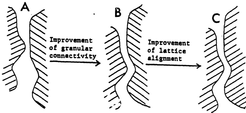
For Tl-based tapes with similar lattice alignment as shown by X-ray diffraction,  $J_c$  can be raised by a large factor by improvement of granular connectivity via uniaxial compression.
