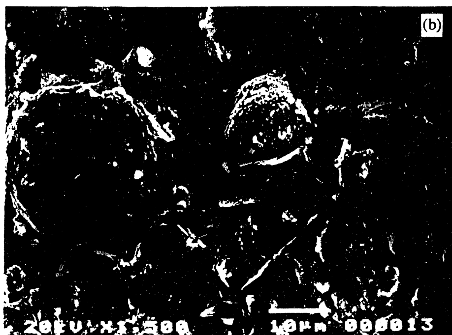
Fig. II. SEM micrographs of (a) magnesium phosphate waste form, (b) zirconium phosphate waste form.
