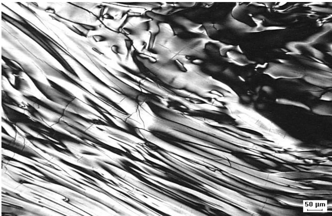
Figure 14: Polarized Light Photomicrograph Showing Flow Orientation In a Particle from Bottom Portion of Coke Run 3 with CTD at 50 psig
