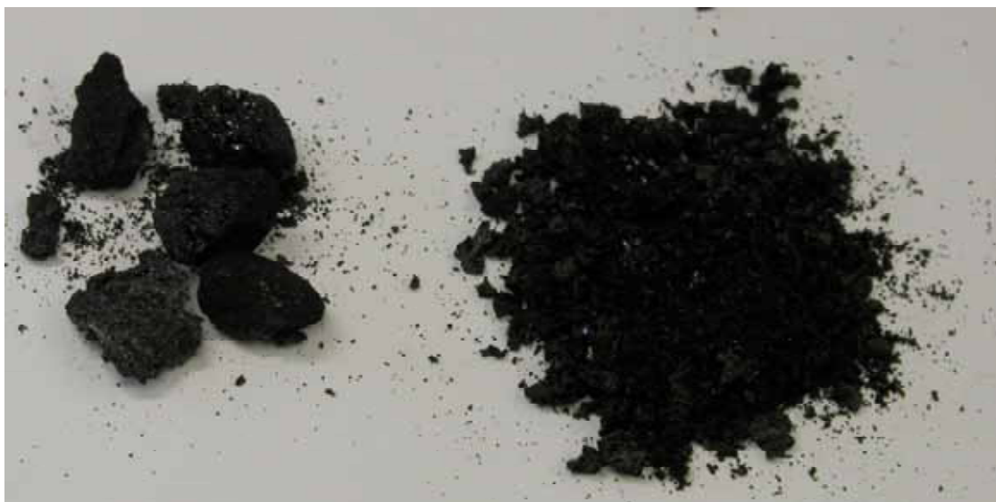
Figure 2. Products formed at 600°C. The product consisted of two phases. One phase consisted of large lumps of material that had a coke-like appearance, while the second phase was a powder similar to that formed at 500°C
