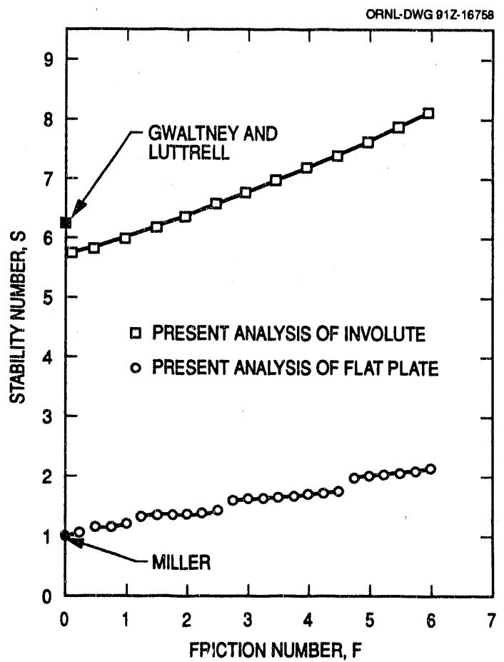
Fig. 2. Effect of fluid friction on hydraulic instability of fuel plates of ANS PS-2 geometry.
