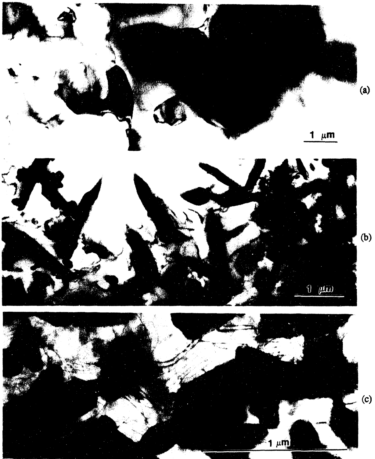
Fig. 6 TEM micrographs of (a) the eutectic \text{Cr}_2\text{Nb} structure in CN-61, (b) block particles in CN-60, and (c) dislocations in CN-60. All specimens were annealed for 3 d at 1100^\circ\text{C} .
