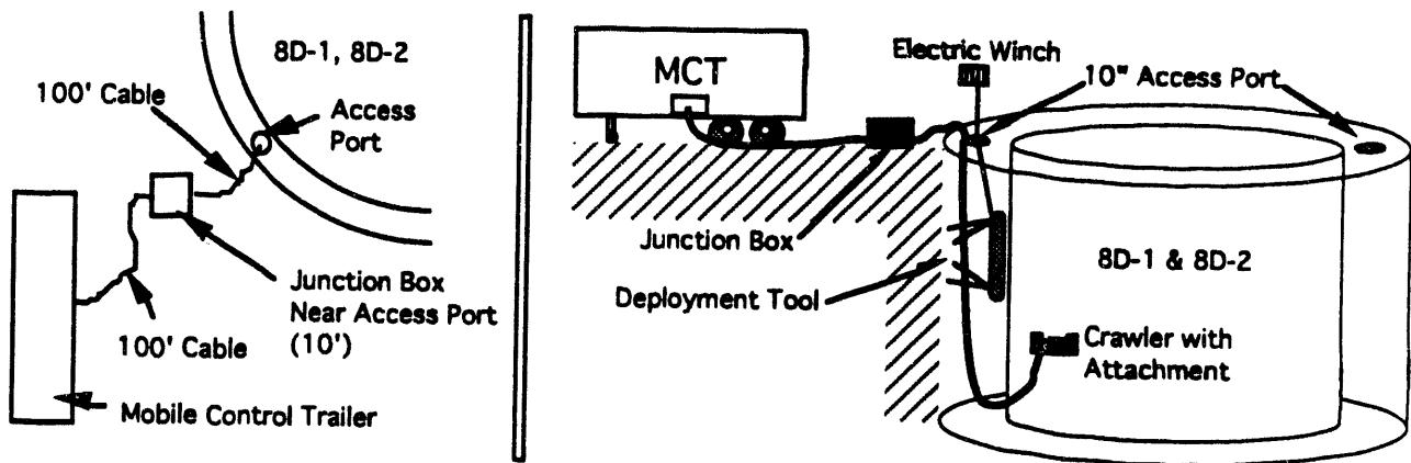
Figure 1 E&MT Waste Tank Inspection System
