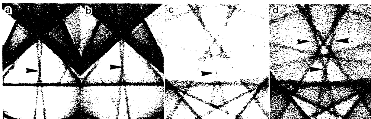
Fig. 3. CBED pattern taken near the [530] incidence a) on the substrate, b) on the layer showing the lattice parameter change; CBED patterns taken with the electron beam incidence slightly tilted from [221]; exact orientation [0.981 0.196 0]; c) on the substrate, d) on the layer. Note loss of the mirror symmetry in the last pattern.
