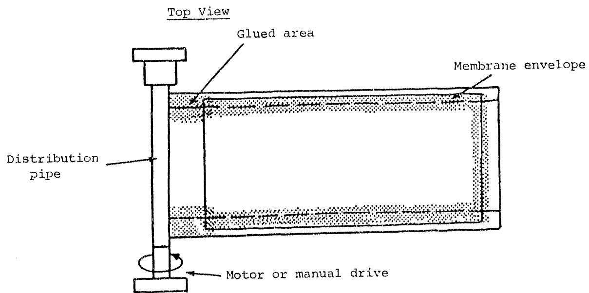
Figure 1. Module winding apparatus.
