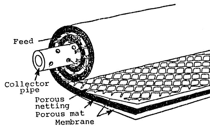
Figure 2. Schematic of a crossflow spiral-wound module.
