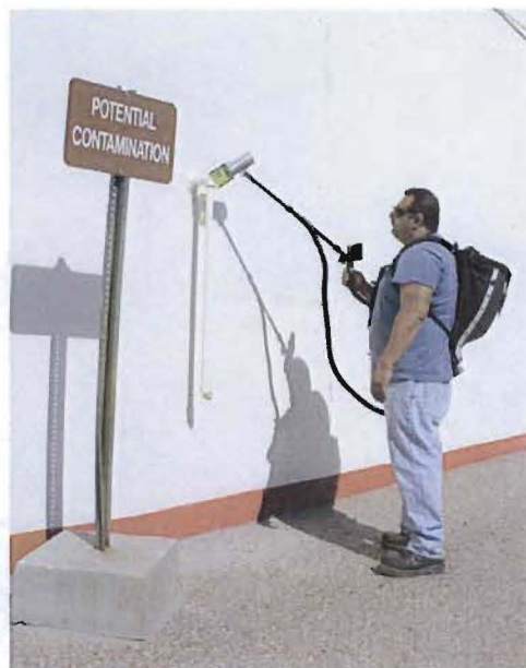
Figure2. A picture of the backpack system is being shown by Leon Lopez. On the right hand side is a typical LIBS spectrum of an aluminum alloy (Al 7075) sample in the region 200 – 420 nanometers (nm).
