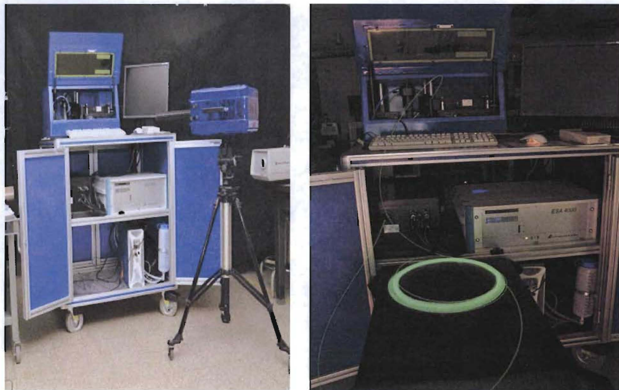
Figure6. In this picture is shown a general view of the Cart / Rack mounted LIBS system on the left and the system coupled to a 50 meter fiber optic cable illuminated with a green alignment laser for visual effects.
