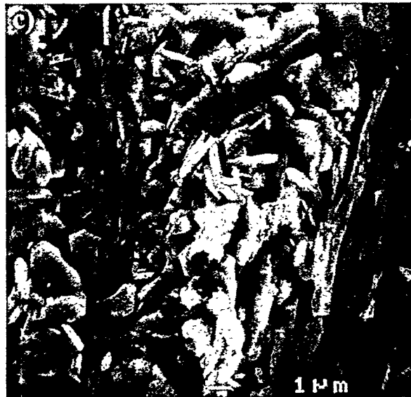
Figure 3.106: SEI micrographs showing fractured cross-section of T7.572 after 100 hrs of exposure. a) fractured section at 33x, b) fractured section at 100x, c) inner scale region at 4,000x
