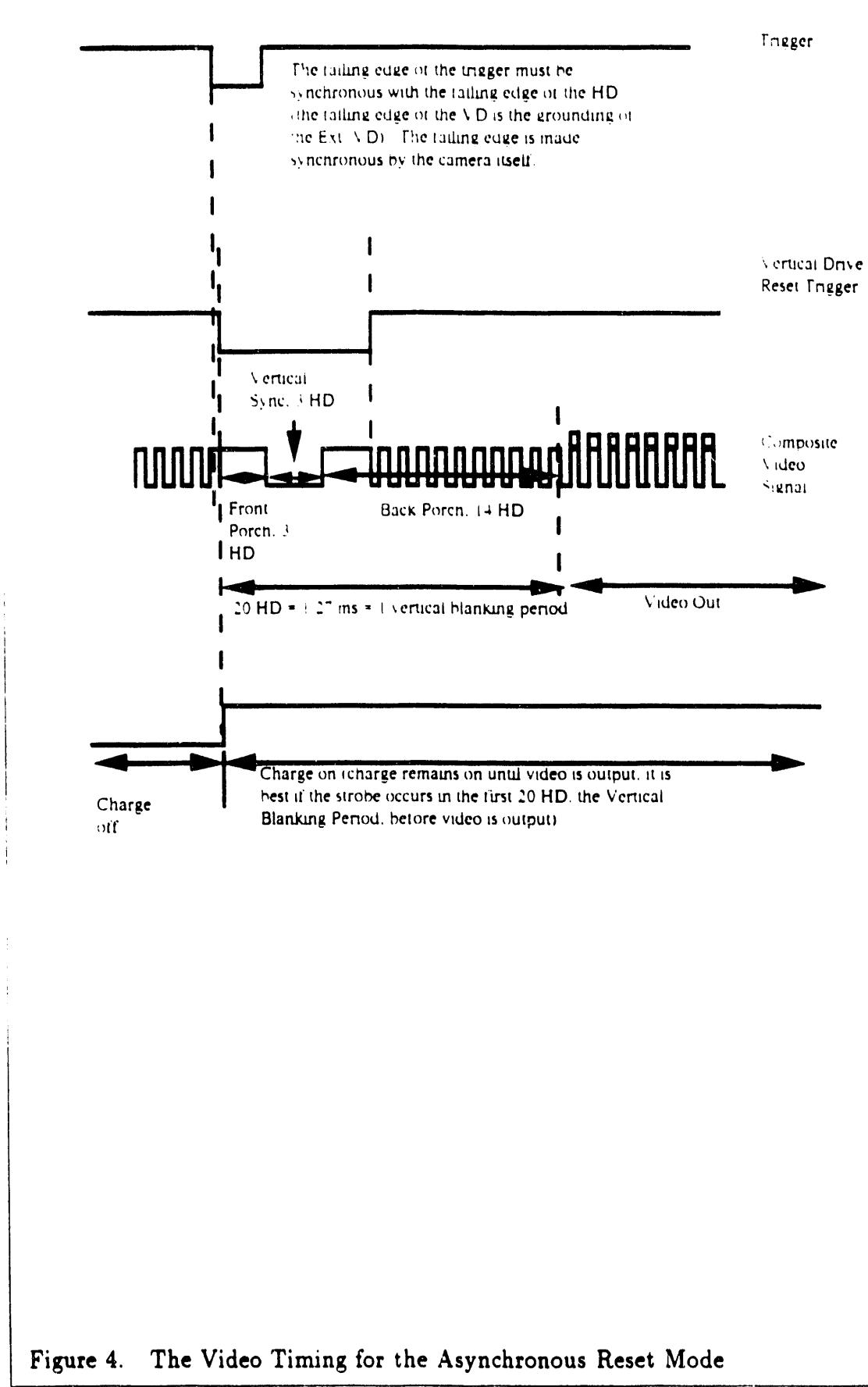
Figure 4. The Video Timing for the Asynchronous Reset Mode
