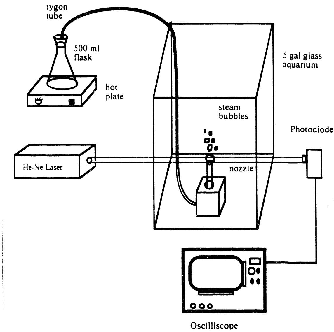
Figure 9. Arrangement to Find the Interval Between Steam Bubbles
