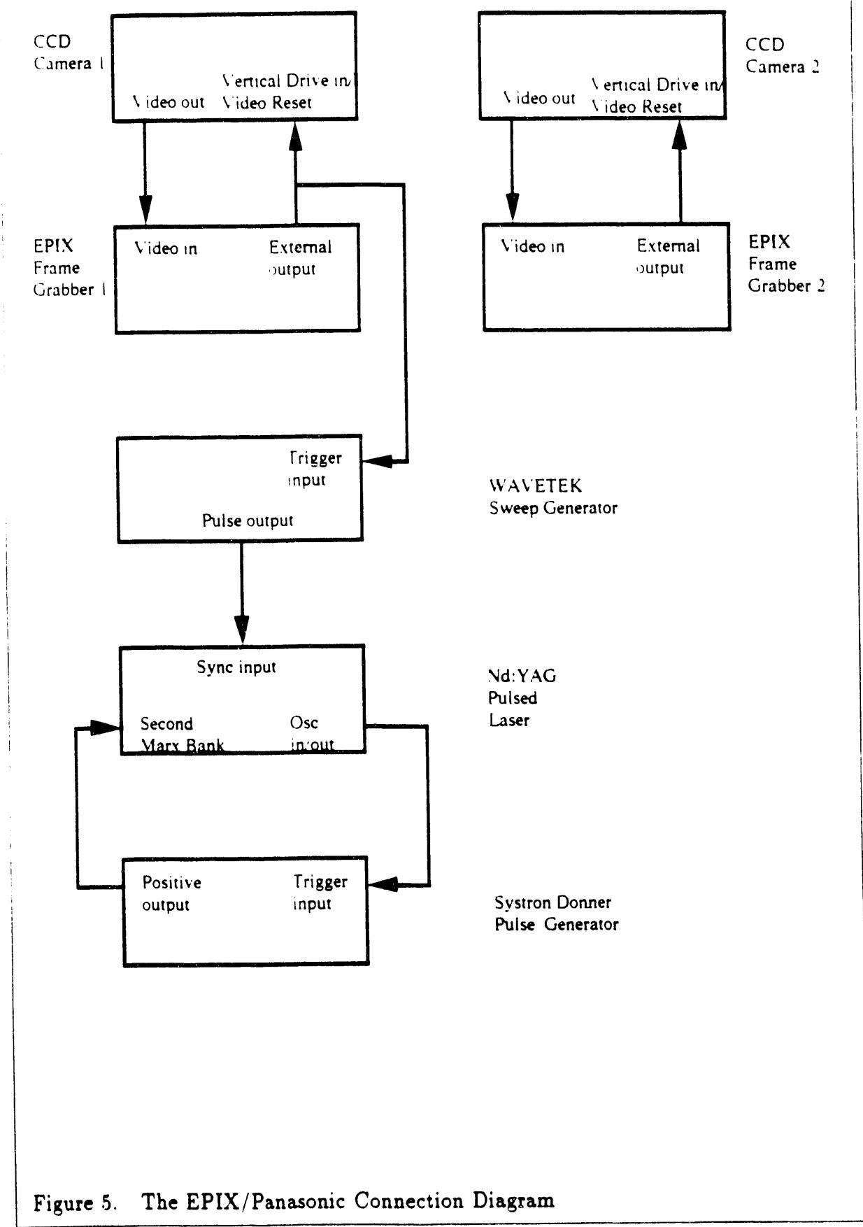
Two cameras are required because their optimum framing rate is 33.3 ms and it is desired to capture a microsecond separation between pulses in the double pulse mode of the laser. An absolute maximum framing rate of 60 frames per second can be achieved (according to the camera specifications), however, at their maximum resolution, the maximum framing rate is 33 frames per second (unless double speed mode is used). The cameras are used at a 640 x 480 resolution.
