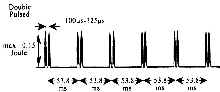
Figure 7. Single Pulse Mode and Double Pulse Mode
