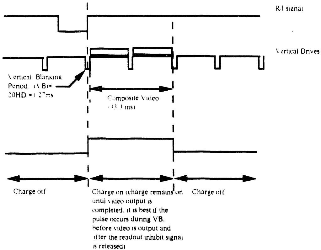
Figure 3. The Video Timing for the Readout Inhibit Mode
