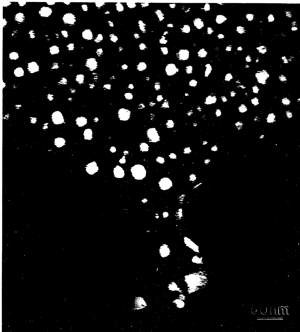
[100] \gamma' dark field of unirradiated HTH Alloy X-750 (Heat A1) showing \gamma' precipitates along incoherent interface between grain boundary and M_{23}C_6 .
