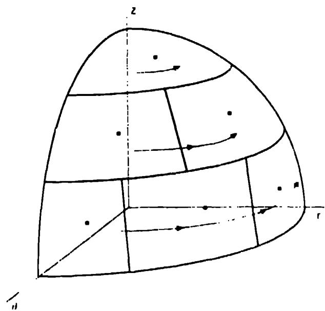
Figure 5-3 The  $S_v$  Angular Bin Arrangement for  $N = 6$
