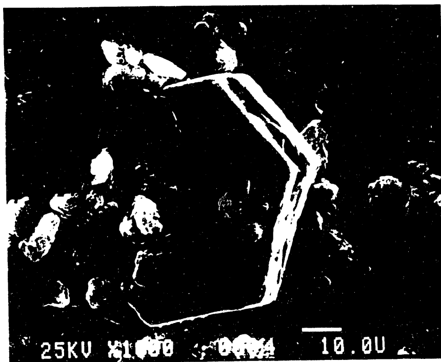
Figure 13. Crystals of \text{Ca(OH)}_2 in S24.
