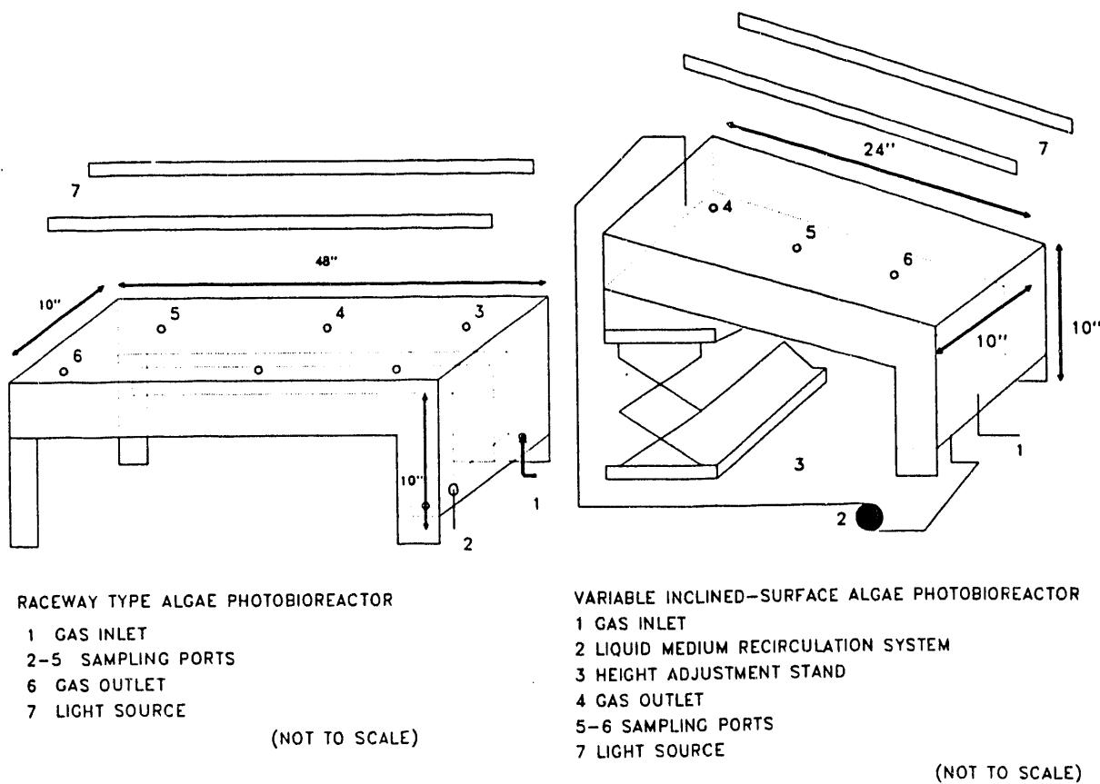
Figure 1. SCHEMATIC ILLUSTRATION AND APPROXIMATE DIMENSIONS OF THE ALGAE PHOTOBIOREACTORS ASSEMBLED BY USING 1/2 INCH THICK PLEXIGLASS PLATE
