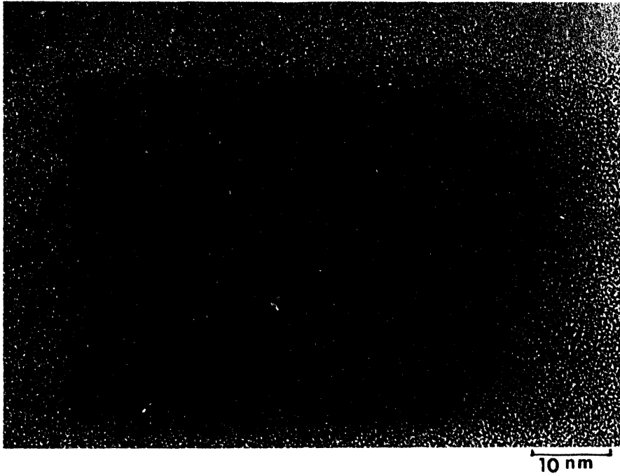
Figure 5.1.1. HRTEM showing amorphous nature of DLC.
