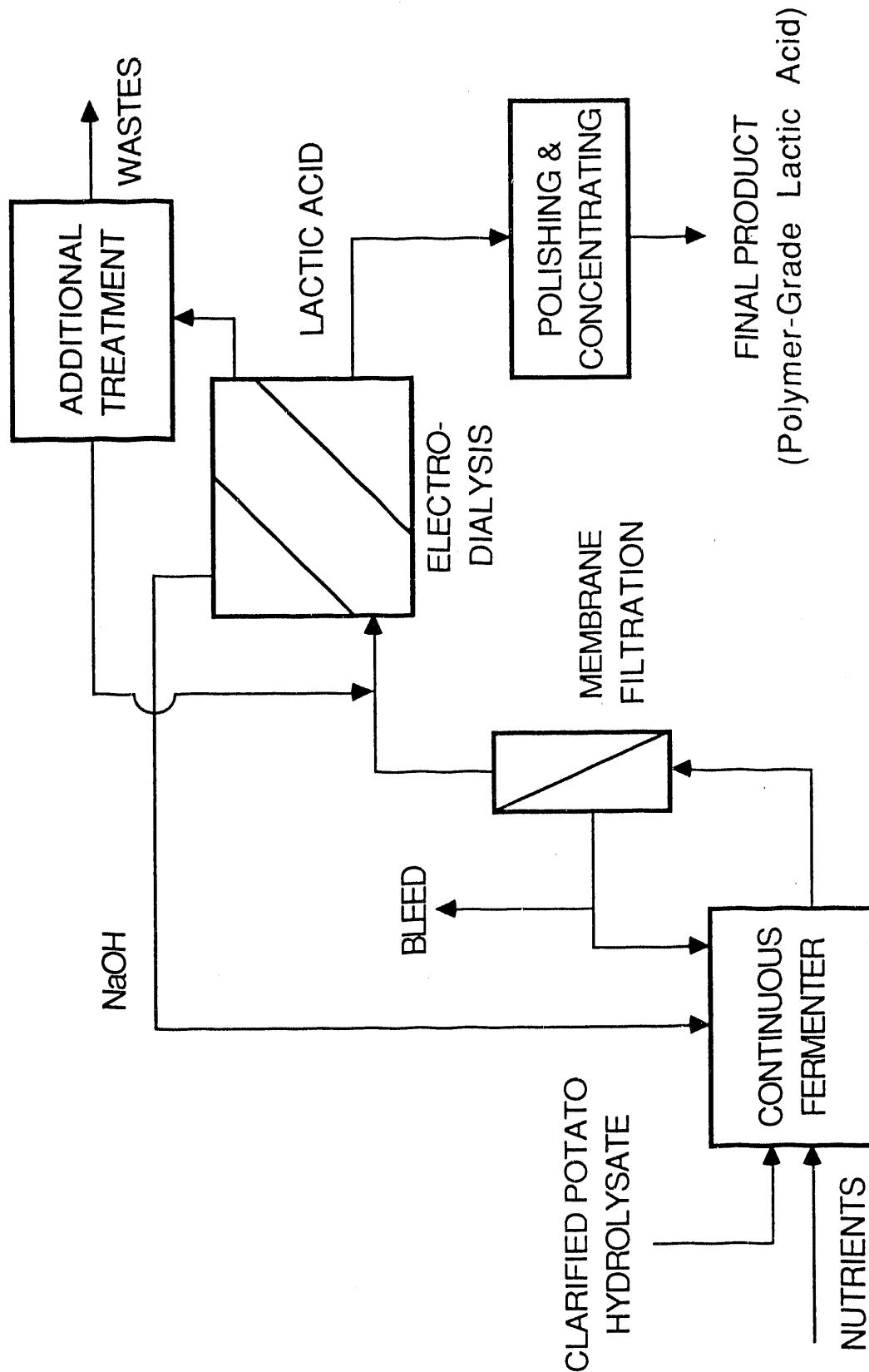
Figure 1. Flowchart of the Argonne Lactic Acid Process
