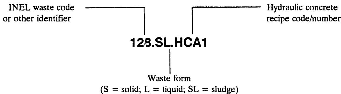
where the hydraulic concrete recipe code/number portion may have an "HC" for hydraulic concrete (Portland cement), or an "HCA" for hydraulic concrete with an additive (Portland cement plus sodium silicate).
