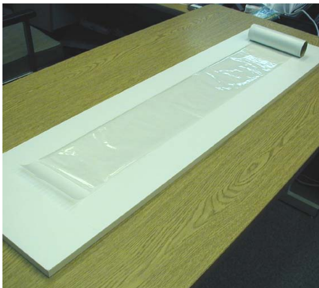
Figure 2. 6F35 random copolymer film, one of seven 6F series copolymer films cast this quarter. The films appear to be void-free and uniform in thickness (25 \mu\text{m} ).
