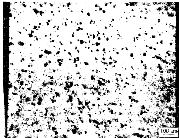
Figure 5. Photomicrograph of unetched rolled composite strip showing distribution of SiC particulate in Al-6061 matrix.
