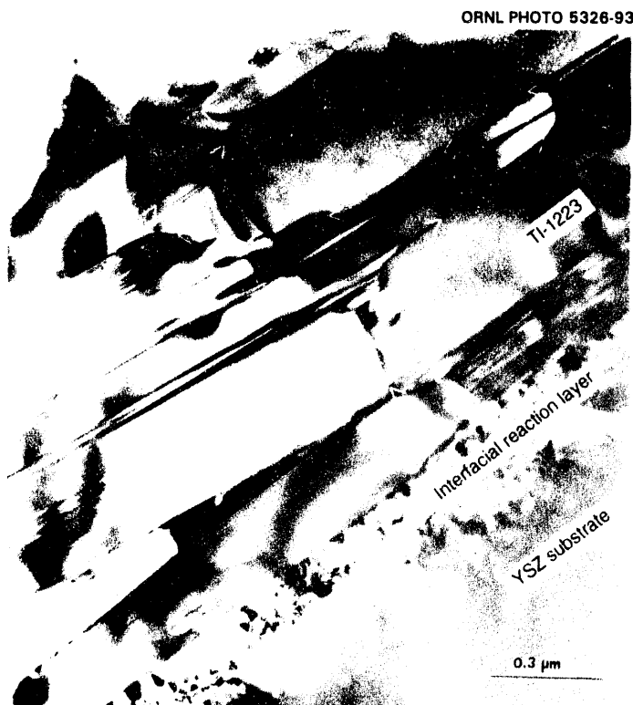
Fig. 1.4. Transmission electron microscopy cross-section image showing the substrate, a thin reaction layer, and tilt (perpendicular to the substrate) and twist (parallel to the substrate) grain boundaries. As indicated by the arrows, tilt boundaries tend, in combination with short segments of twist boundary, to extend over several grains. The thin area in this view covers about half the sample thickness.
