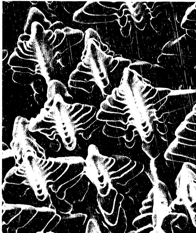
This micrograph shows dendrites (treelike crystallites) in a weld made on a single-crystal PWA-1480 turbine blade alloy. ORNL researchers have found that making and studying welds in single crystals of stainless steel can provide new insights into how a weld's microstructure is formed.
