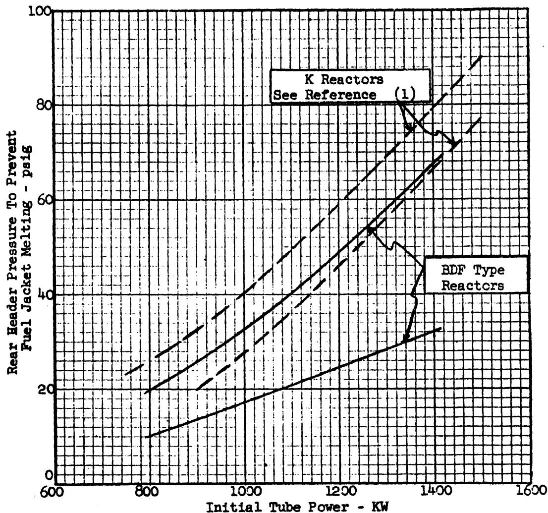
NOTE: The solid lines of this figure are cross-plots from Figure 1 at a heater rod temperature of 1000 F. This should be approximately equivalent to a 1220 F uranium fuel surface temperature.
