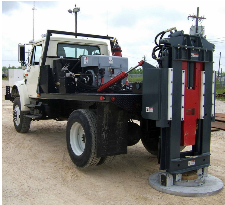
Figure 4: An AXIS™ accelerated weight-drop seismic source was used for seismic surveys.
